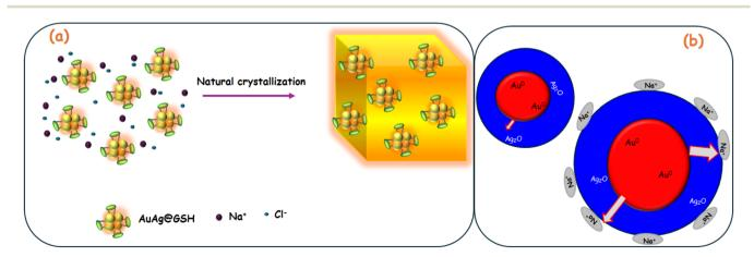
Scheme 2 Mechanism of Na<sup>+</sup> induced fluorescence enhancement based on (a) natural crystallization and confinement, (b) charge redistribution.
