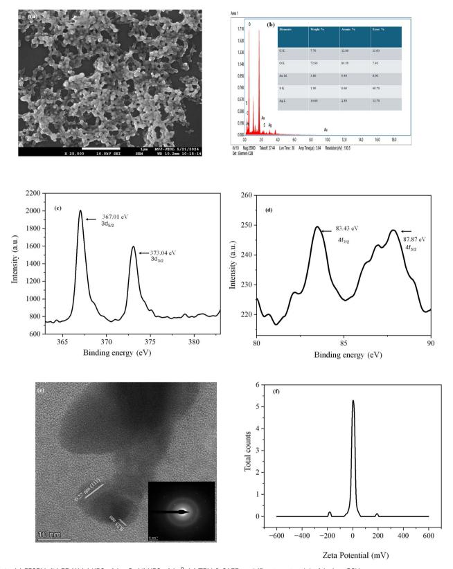
Fig. 1 (a) FESEM, (b) EDAX (c) XPS of  $Ag_2O$ , (d) XPS of  $Au^0$ , (e) TEM & SAED and (f) zeta potential of AuAg@GSH.
