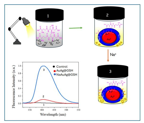
Scheme 1 Na+ highly enhanced the fluorescence of hydrothermally synthesized AuAg@GSH
