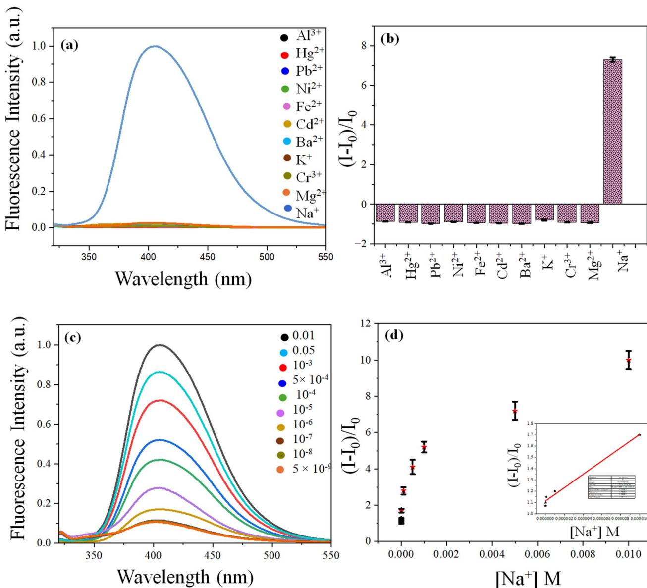
Fig. 2 (a) Fluorescence spectra and (b) bar diagram of AuAg@GSH with metal ion; (c) fluorescence spectra of AuAg@GSH with [Na<sup>+</sup>] and (d) LOD estimation of Na<sup>+</sup> detection.
