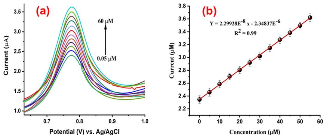
Fig. 12 (a) DPV response of PVP-SrO/GCE against various VNB concentrations in 0.1 BRB (pH 5.0), ranging between 0.05 and 60.0  $\mu\text{M}$ . (b) The linear plot corresponding to oxidation peak currents to the various concentrations of VNB, with  $R^2 = 0.99$ .
