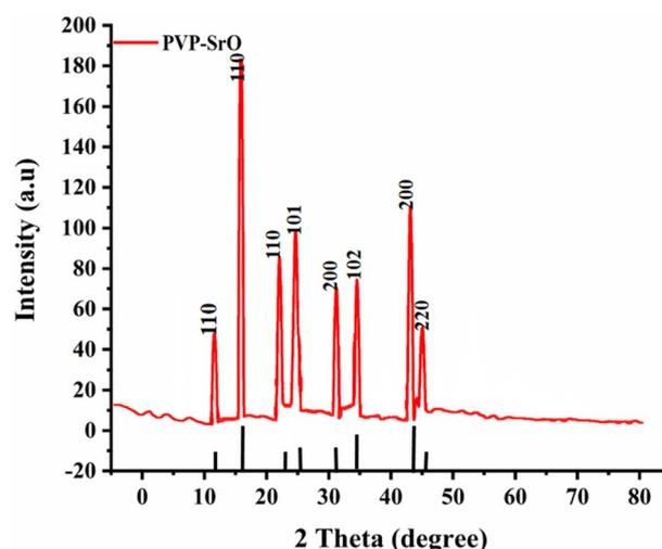
Fig. 4 XRD patterns of PVP-SrO nanostructures.
