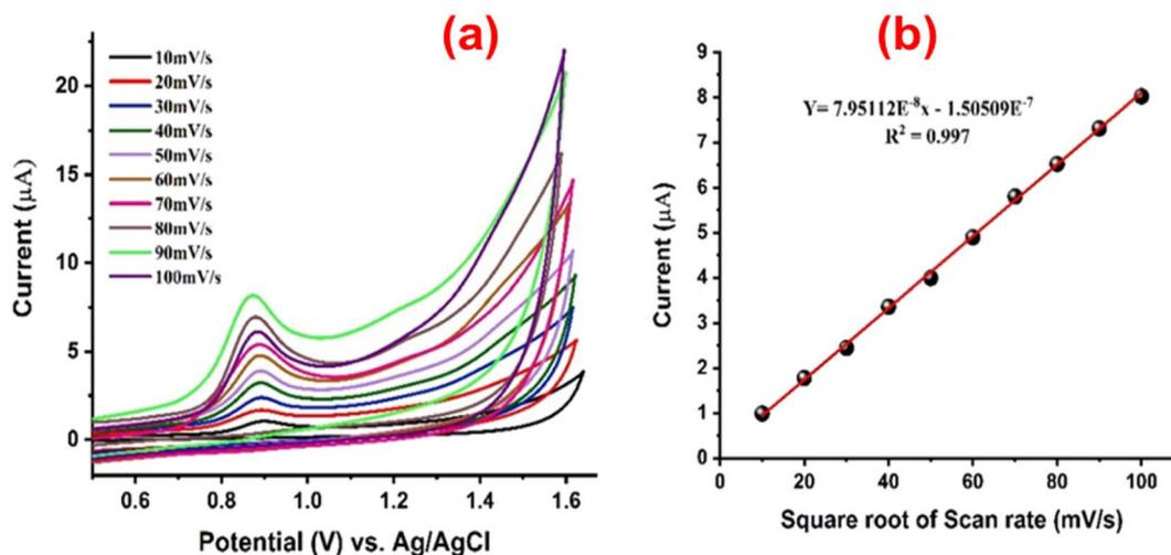
Fig. 11 (a) CV response of PVP-SrO/GCE to 20.0  $\mu\text{M}$  VNB in 0.1 M BRB (pH 5.0) at different scan rates from 10.0 to 100  $\text{mV s}^{-1}$ . (b) A linear correlation plot of oxidation peak current against the square root of scan rate, showing an  $R^2$  value of 0.997.
