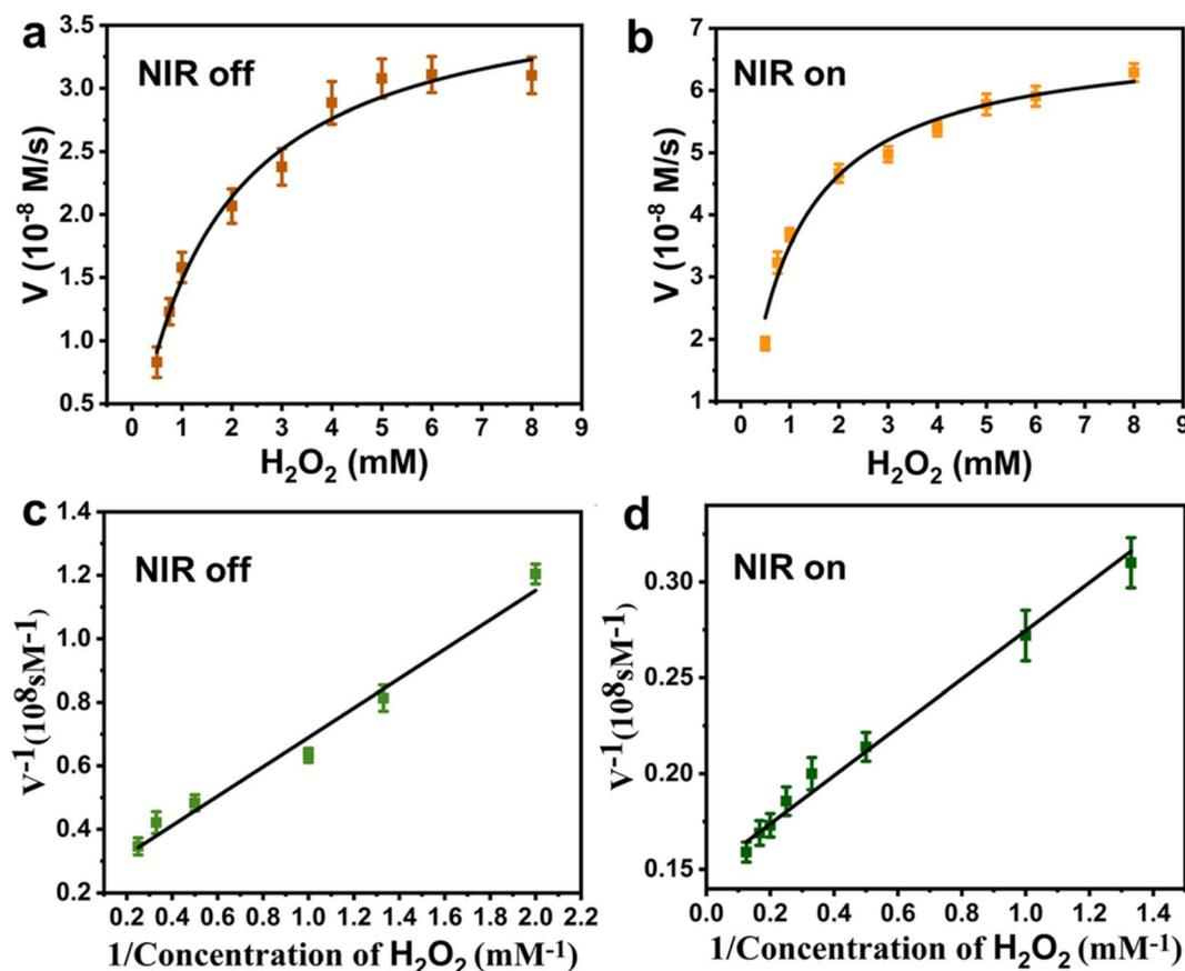
Fig. 5 Steady-state kinetic plots of Pt-MoS<sub>2</sub> using H<sub>2</sub>O<sub>2</sub> as substrate in the absence (a) and presence (b) of 808 nm NIR light irradiation (1 W cm<sup>-2</sup>, 5 min). Double-reciprocal plots of Pt-MoS<sub>2</sub> using H<sub>2</sub>O<sub>2</sub> as substrate in the absence (c) and presence (d) of 808 nm NIR light irradiation (1 W cm<sup>-2</sup>, 5 min).
