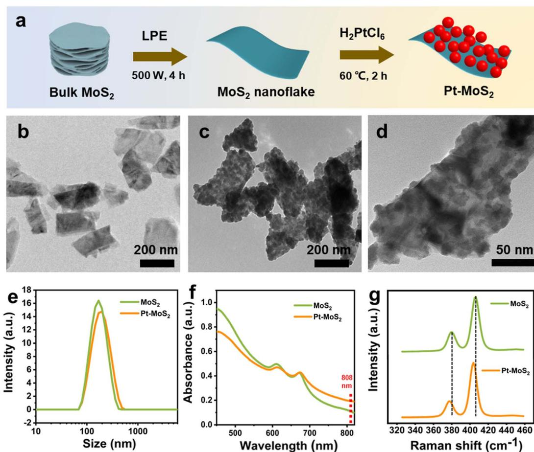
Fig. 1 (a) Schematic illustration for the preparation process of the  $\text{MoS}_2$  nanoflake and Pt- $\text{MoS}_2$  nanocomposite. TEM images of  $\text{MoS}_2$  nanoflake (b) and Pt- $\text{MoS}_2$  nanocomposite (c and d). (e) DLS analysis for hydrodynamic sizes of  $\text{MoS}_2$  and Pt- $\text{MoS}_2$ . (f) UV-vis absorbance spectra of  $\text{MoS}_2$  and Pt- $\text{MoS}_2$  at 100  $\mu\text{g mL}^{-1}$ . (g) Raman spectra of  $\text{MoS}_2$  and Pt- $\text{MoS}_2$ .
