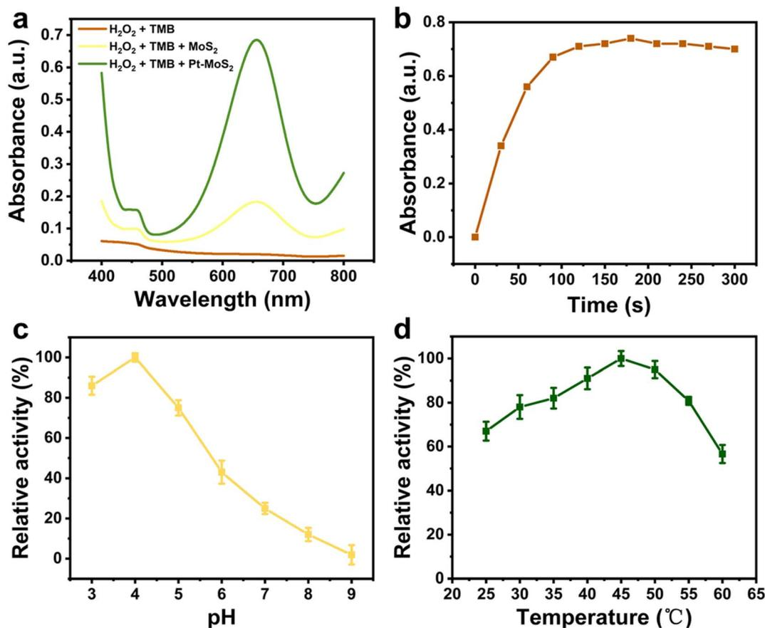
Fig. 4 (a) UV-vis absorption spectra of different H<sub>2</sub>O<sub>2</sub> + TMB solutions containing blank, MoS<sub>2</sub> or Pt–MoS<sub>2</sub> after reaction for 10 min. (b) Time-dependent profiles of Pt–MoS<sub>2</sub> + H<sub>2</sub>O<sub>2</sub> + TMB solutions at the absorbance of 652 nm in 300 s. Effect of pH (c) and temperature (d) on the POD-mimetic catalytic performance.
