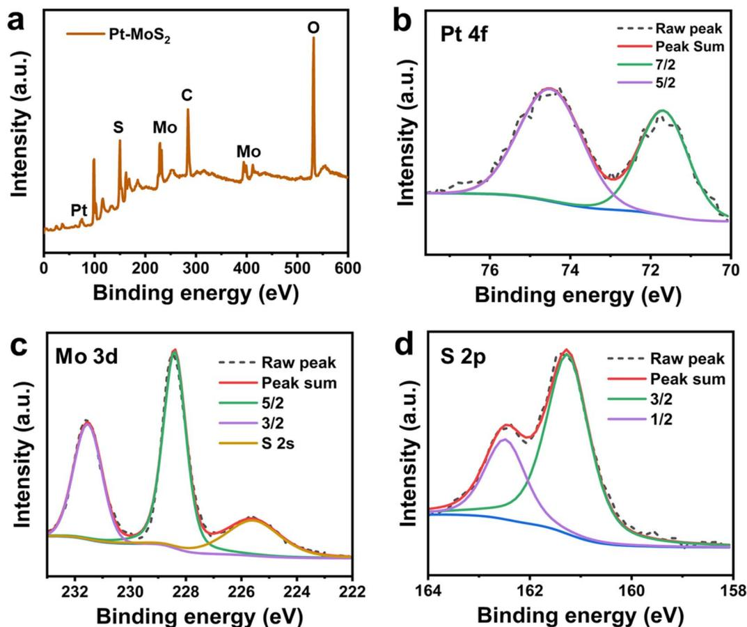
Fig. 2 (a) The XPS survey of Pt–MoS<sub>2</sub>. The high-resolution XPS spectra of Pt 4f (b) Mo 3d (c) and (d) S 2p signals for Pt–MoS<sub>2</sub>.
