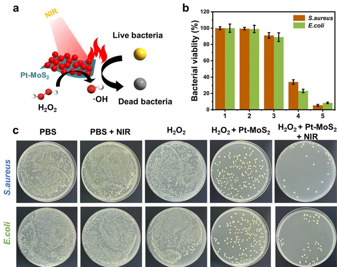
Fig. 6 (a) Scheme for the bactericidal mechanism of Pt-MoS<sub>2</sub> nanozyme after the irradiation of 808 nm NIR laser. (b) Bacterial viabilities of *S. aureus* and *E. coli* after treated by different groups (1: PBS; 2: PBS + NIR; 3: H<sub>2</sub>O<sub>2</sub>; 4: H<sub>2</sub>O<sub>2</sub> + Pt-MoS<sub>2</sub>; 5: H<sub>2</sub>O<sub>2</sub> + Pt-MoS<sub>2</sub> + NIR). (c) Bacterial colonies photographs of *S. aureus* and *E. coli* after treated by different groups.
