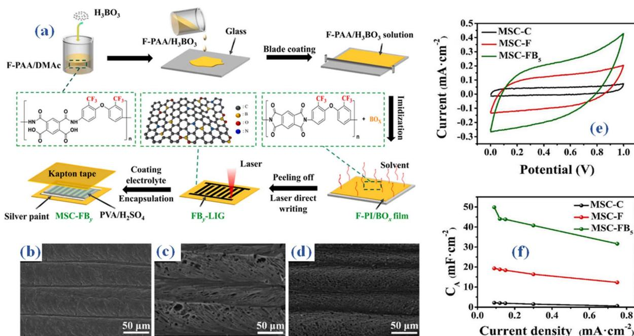
Fig. 3 (a) Schematic representation of F-PI/Bo<sub>x</sub> film fabrication process (b–d) SEM outcomes of fabricated films (e) the CV curves for MSC-C, MSC-F, and MSC-FB<sub>5</sub> (f) areal capacitance at different current densities.<sup>32</sup>
