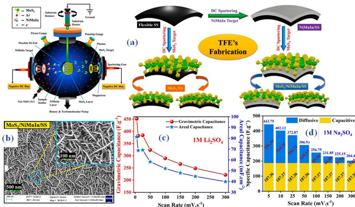
Fig. 7 (a) Method illustration MoS<sub>2</sub> nanowires in thin-film electrodes (TFEs) made *in situ* using the magnetron sputtering process (b) surface morphology outcomes (SEM) (c and d) specific capacitance using 1 M Li<sub>2</sub>SO<sub>4</sub> and 1 M Na<sub>2</sub>SO<sub>4</sub> as electrolyte respectively.<sup>54</sup>
