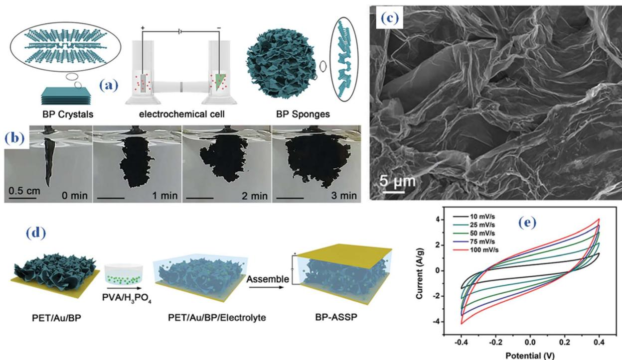
Fig. 9 (a and b) Synthesis method of BP sponges from bulk BP crystals produces ultrathin nanosheets (c) SEM (d) electrolyte synthesis process, made of phosphoric acid and poly(vinyl alcohol) (PVA/H<sub>3</sub>PO<sub>4</sub>) (e) CV.<sup>59</sup>
