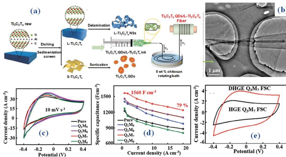
Fig. 4 (a) Schematic representation of L- $\text{Ti}_3\text{C}_2\text{T}_x$  fiber electrode fabrication process (b) SEM outcomes (c) CV curves  $10 \text{ mV s}^{-1}$  (d) the specific capacitance trend against different current densities, (e) CV of delaminated montmorillonite/polyvinyl alcohol (PVA) dimethyl sulfoxide (DMSO) flexible hydrogel (F-MMT/PVA DHGE) electrolyte devices.<sup>35</sup>
