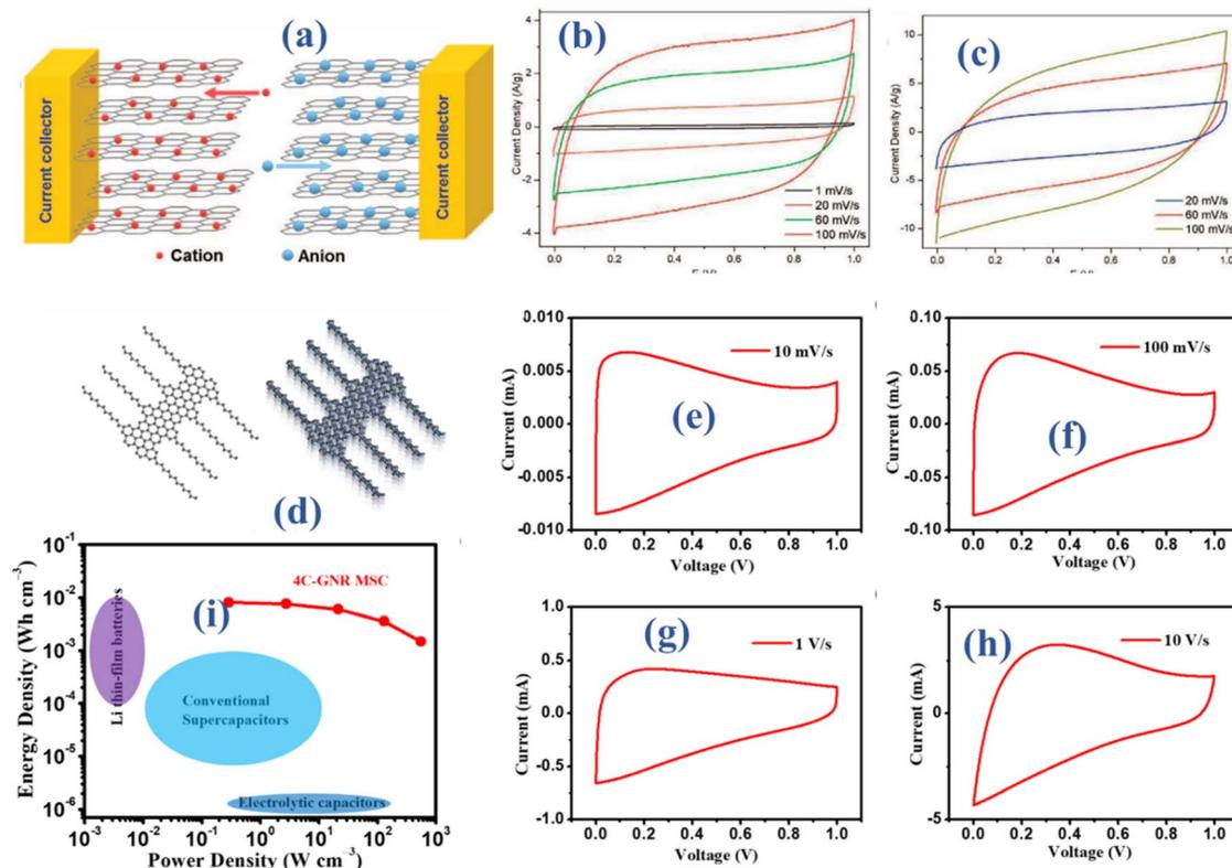
Fig. 2 (a) Schematic illustration of fabricated device (b and c) CV elucidating EDLCs behavior<sup>28</sup> (d) molecular arrangement of the utilized alkyl-substituted graphene nanoribbon (GNR) (e–h) CV at multiple scan rates (i) specific energy and power outcomes.<sup>29</sup>
