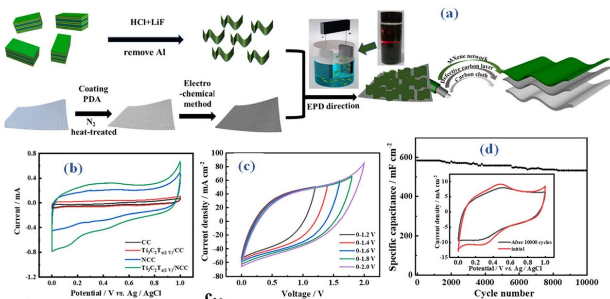
Fig. 6 (a) Method illustration for producing nitrogen-doped superhydrophilic carbon cloth based binder-free  $\text{Ti}_3\text{C}_2\text{T}_x$  (EPD)/ENCC device (b) CV comparison (c) CV of  $\text{Ti}_3\text{C}_2\text{T}_x$  (EPD)/ENCC at different potential windows (d) cyclic life performance with inset revealing CV outcomes before and after 10 k cycles.<sup>48</sup>
