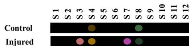
Fig. 3 The response of sensor for analysis of urine samples of control and injured individuals. The analysis was performed in oven at 75 °C for 90 min.
