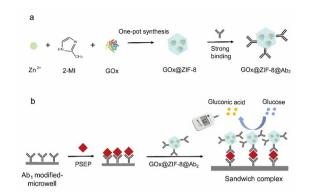
Fig. 1 Illustration of the GOx@ZIF-8@Ab<sub>2</sub> synthesis process (a) and the concept behind PGM immunoassay (b).
