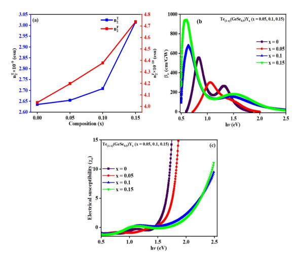
Fig. 10 (a)  $n_z^T$  and  $n_z^F$  variation with the composition, (b) nonlinear absorption the coefficient  $\beta_c$ , (c) electrical susceptibility ( $\chi_c$ ) variation with hv for the studied thin films.
