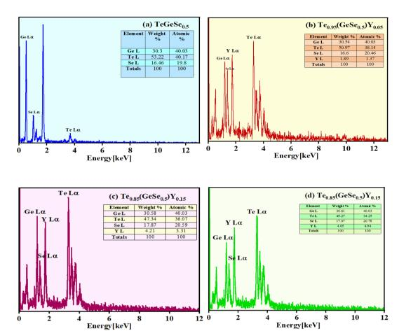
Fig. 3 EDX spectra for the compositional study of the  $Te_{(1-x)}(GeSe_{0.5})Y_x$  thin films (a) x = 0, (b) x = 0.05, (c) x = 0.1, (d) x = 0.15.
