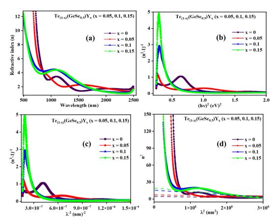
Fig. 7 (a) Variation in 'n', (b)  $(n^2 - 1)^{-1}$  versus  $(hv)^2$  plot, (c)  $(n^2 - 1)^{-1}$  versus  $(\lambda)^{-2}$  plot, and (d)  $n^2$  versus  $(\lambda)^2$  plot for the Te<sub>(1-x)</sub>(GeSe<sub>0.5</sub>)Y<sub>x</sub> thin films.
