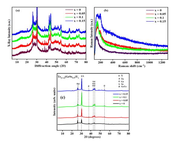
Fig. 1 (a) X-ray diffractograms, (b) Raman spectra, (c) Rietveld refined XRD of  $Te_{(1-x)}(GeSe_{0.5})Y_x$  (x = 0, 0.05, 0.1, 0.15) thin-film samples.
