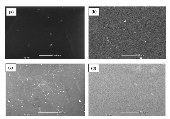
Fig. 2 SEM images for surface morphological study of the  $Te_{(1-x)}$  (GeSe<sub>0.5</sub>) $Y_x$  films. (a) x = 0, (b) x = 0.05, (c) x = 0.1, (d) x = 0.15.
