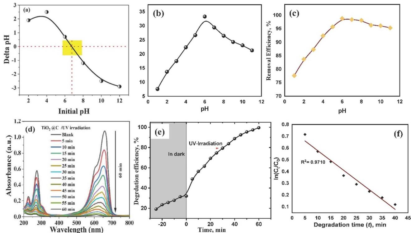
Fig. 4 (a) Zeta potential of  $\text{TiO}_2\text{-C@N}$  photocatalyst in 0.01 M KCl as a function of pH. (b & c) Effect of pH on the removal of MB in the dark and in UV irradiation respectively. (d) Absorption spectra in the degradation process of MB dye in UV light (photodegradation). (e) The impact of duration on the removal efficiency under both dark and UV radiation conditions. (f) First order kinetics for the photocatalytic process.
