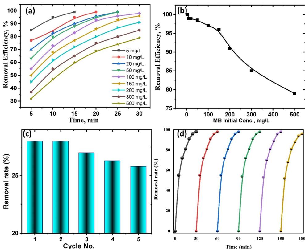
Fig. 6 (a & b) Photodegradation efficiency of MB by  $\text{TiO}_2\text{-C@N}$  as a function of MB initial concentrations at pH 6. Reusability of  $\text{TiO}_2\text{-C@N}$  photocatalyst in the (c) dark, and (d) UV light.
