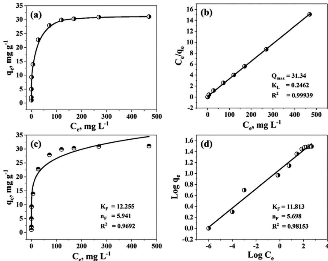
Fig. 5 (a) Adsorption isotherm of MB on the  $\text{TiO}_2\text{-C@N}$  in dark under specific conditions [pH 6,  $w = 10$  mg, contact time 30 min], plot of (b) Langmuir, (c) nonlinear Freundlich, and (d) linear Freundlich.
