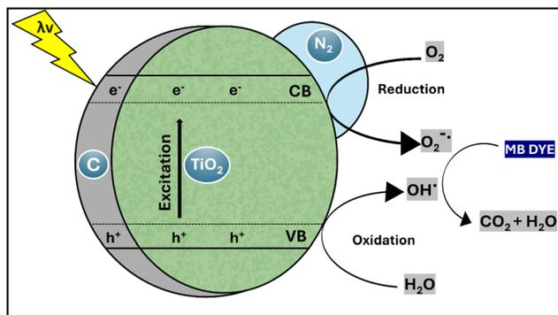
Fig. 7 Photocatalytic degradation diagram of  $\text{TiO}_2\text{-C@N}$  photocatalyst.
