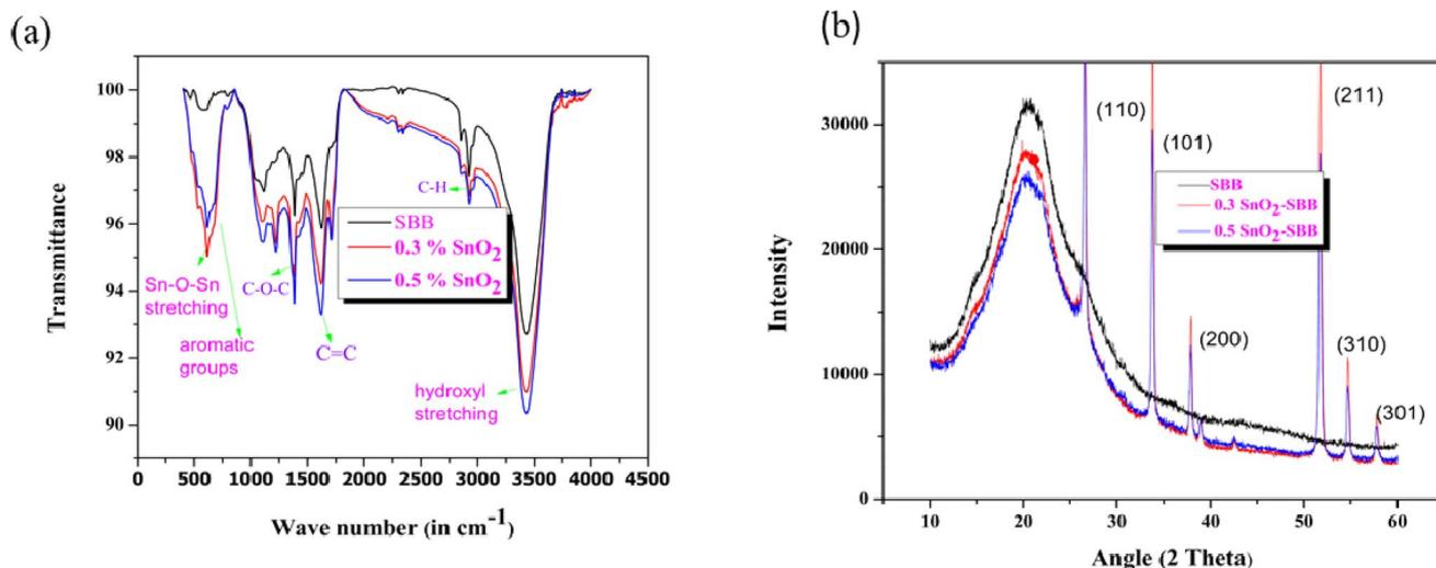
Fig. 4 (a) Comparison of the FTIR spectrum of SBB with  $\text{SnO}_2$ -SBB nanocomposites and (b) XRD patterns of SBB and its corresponding composites.
