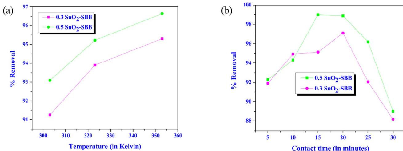
Fig. 7 (a) Alteration of removal (%) with temperature and (b) change in removal (%) with time.
