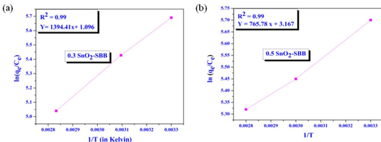
Fig. 8 Thermodynamic isotherm plots between  $\ln(q_e/C_e)$  vs.  $1/T$ . (a) 0.3 SnO<sub>2</sub>-SBB and (b) 0.5 SnO<sub>2</sub>-SBB nanocomposites.
