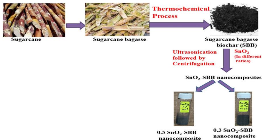
Fig. 1 Synthesis of \text{SnO}_2 -modified sugarcane bagasse biochar ( \text{SnO}_2 -SBB) nanocomposites.
