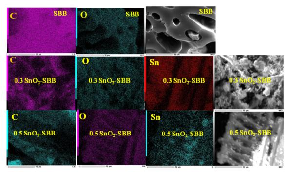
Fig. 2 SEM and elemental mapping images of the SBB/SnO<sub>2</sub> nanocomposites at a magnification of 10 μm.
