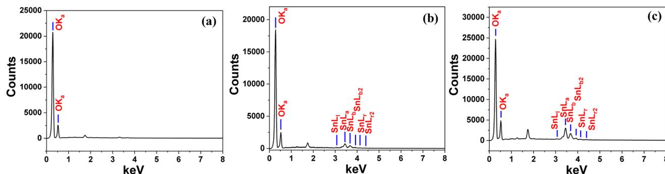
Fig. 3 EDX spectrum of (a) SBB, (b) 0.3 SnO<sub>2</sub>-SBB and (c) 0.5 SnO<sub>2</sub>-SBB nanocomposites.
