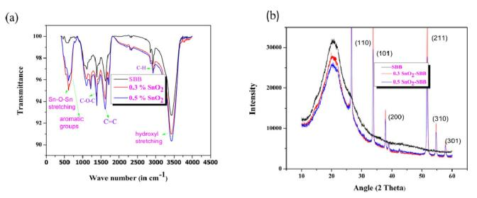
Fig. 4 (a) Comparison of the FTIR spectrum of SBB with SnO<sub>2</sub>-SBB nanocomposites and (b) XRD patterns of SBB and its corresponding composites.
