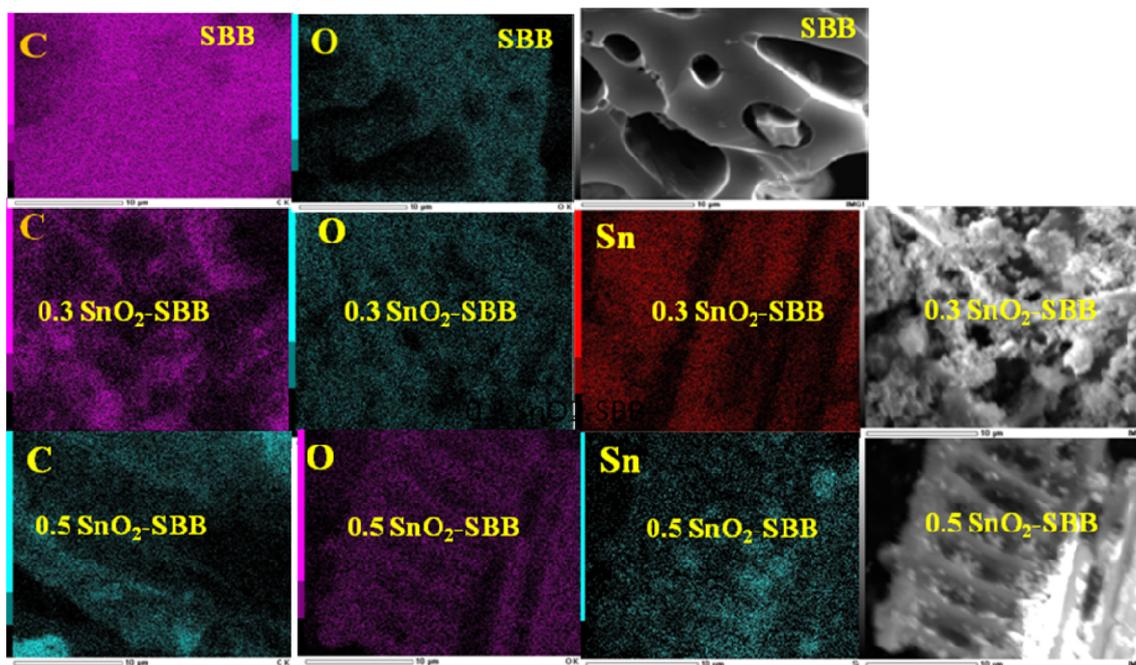
Fig. 2 SEM and elemental mapping images of the SBB/SnO<sub>2</sub> nanocomposites at a magnification of 10 µm.
