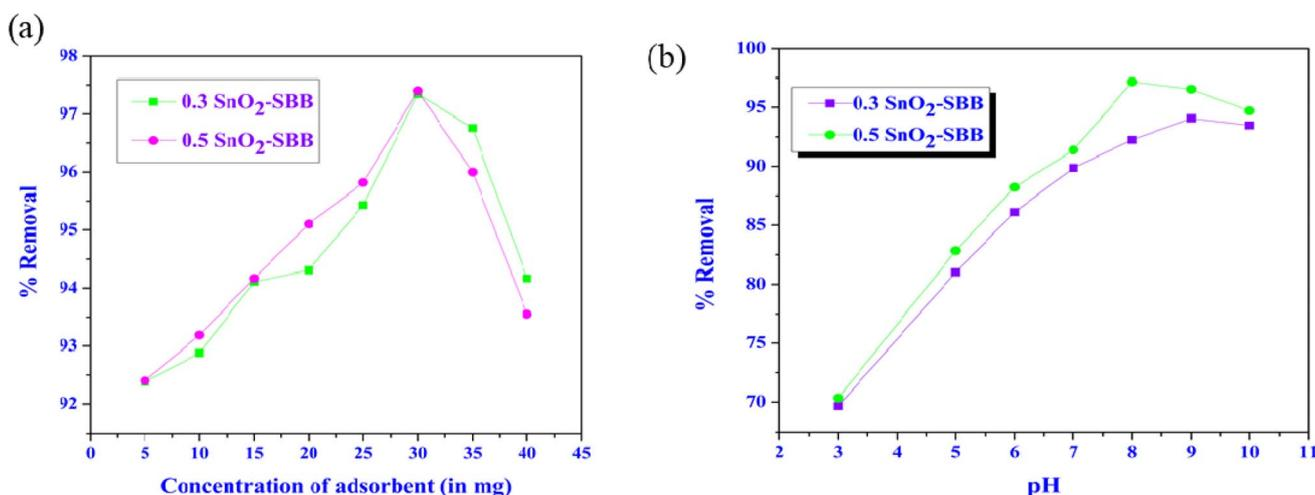
Fig. 6 (a) Removal percentage of malachite green with different adsorbent dosages and (b) variation in the removal percentage of malachite green with variable pH ranges.
