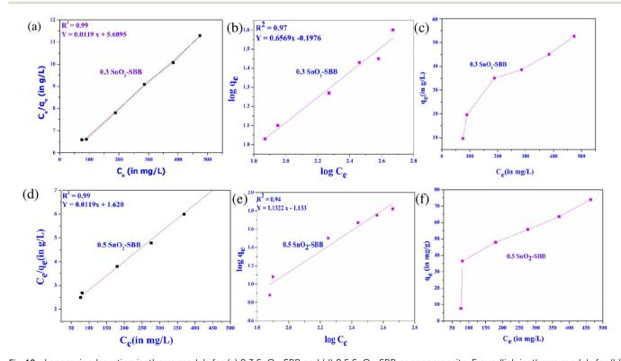
Fig. 10 Langmuir adsorption isotherm models for (a)  $0.3 \, \text{SnO}_2\text{-SBB}$  and (d)  $0.5 \, \text{SnO}_2\text{-SBB}$  nanocomposite. Freundlich isotherm models for (b)  $0.3 \, \text{SnO}_2\text{-SBB}$  and (e)  $0.5 \, \text{SnO}_2\text{-SBB}$  nanocomposite. Plot for adsorption capacity *versus* equilibrium concentration for (c)  $0.3 \, \text{SnO}_2\text{-SBB}$  and (f)  $0.5 \, \text{SnO}_2\text{-SBB}$  nanocomposites.
