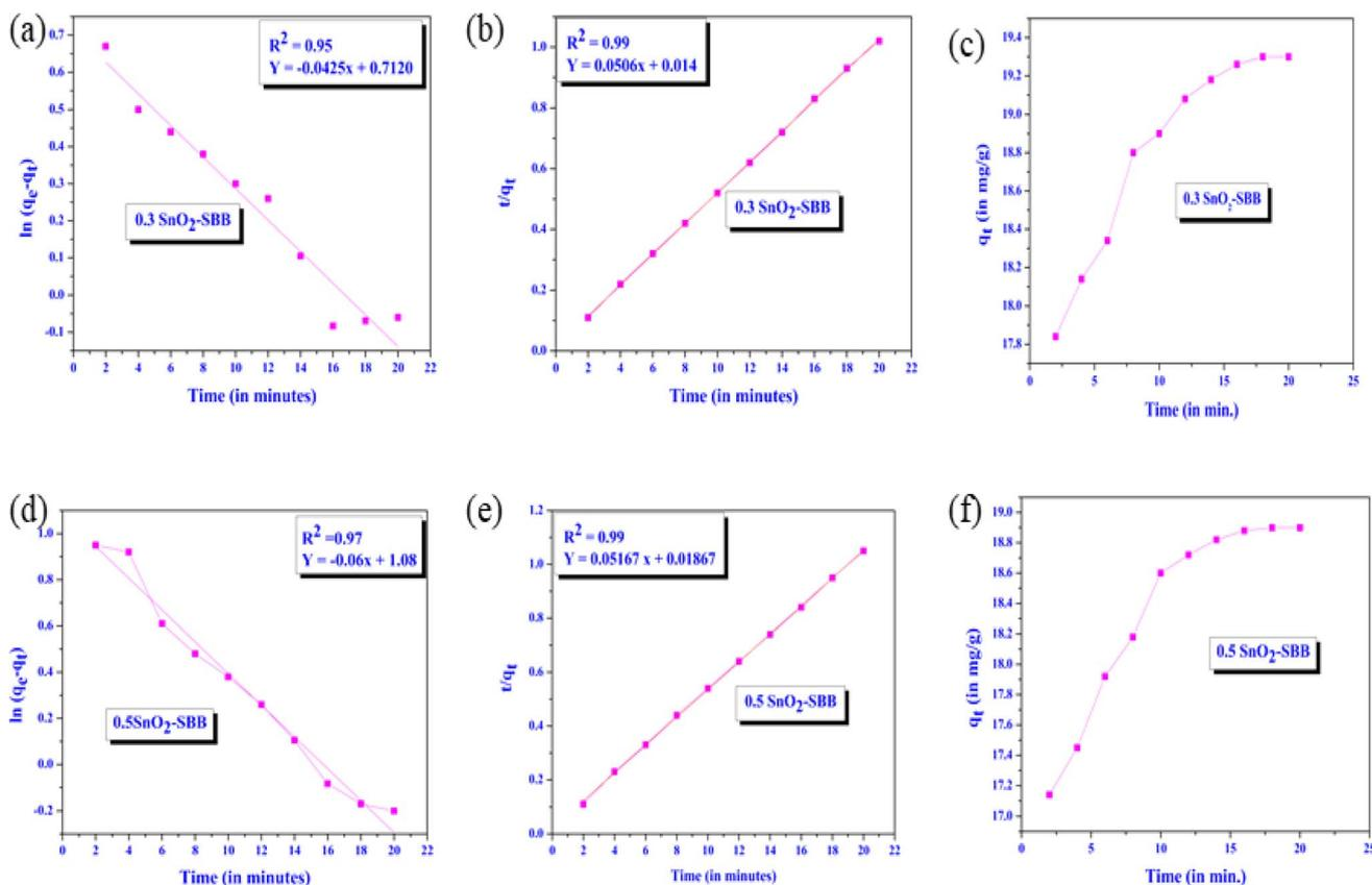
Fig. 9 Pseudo-first-order kinetic curves (linear fitted) of the SnO<sub>2</sub>-SBB nanocomposite (a and d), pseudo-second-order kinetic curves (linear fitted) of SnO<sub>2</sub>-SBB nanocomposite (b and e) and time vs. adsorption capacity curves (c and f).
