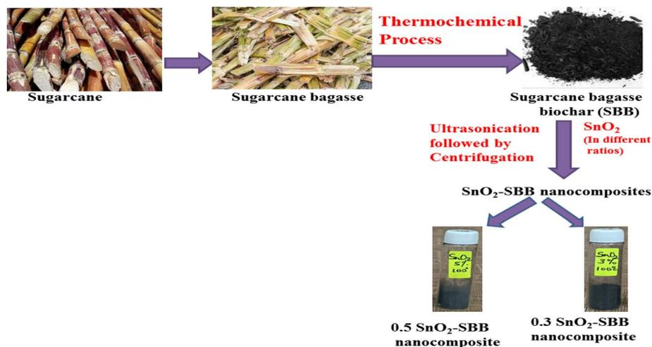
Fig. 1 Synthesis of SnO<sub>2</sub>-modified sugarcane bagasse biochar (SnO<sub>2</sub>-SBB) nanocomposites.
