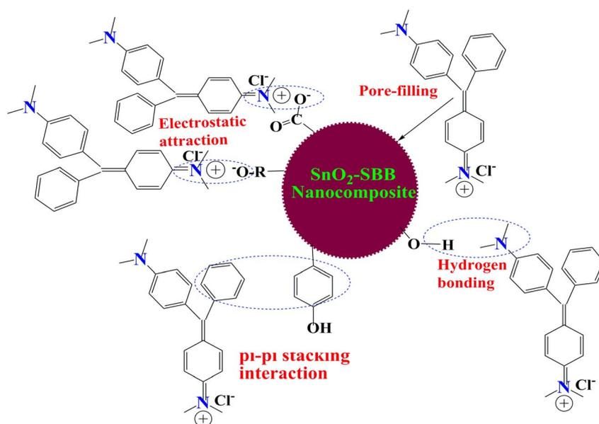
Fig. 11 Plausible adsorption mechanism of SnO<sub>2</sub>-SBB nanocomposites for the removal of MG dye.
