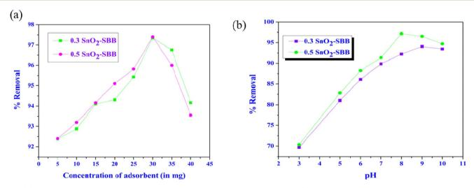
Fig. 6 (a) Removal percentage of malachite green with different adsorbent dosages and (b) variation in the removal percentage of malachite green with variable pH ranges.
