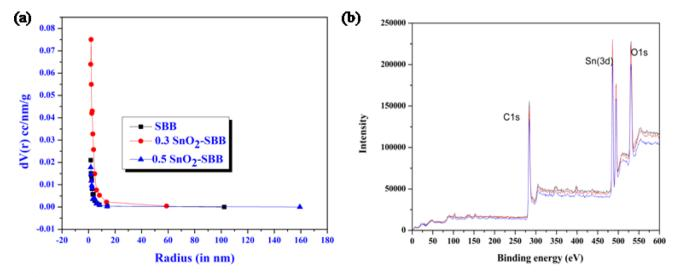
Fig. 5 (a) Plot representing the comparative pore size distribution curve for biochar and composites. (b) XPS spectrum of composite containing important peaks of carbon, oxygen and tin.
