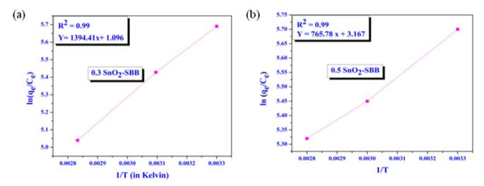
Fig. 8 Thermodynamic isotherm plots between  $\ln(q_e/C_e)$  vs. 1/T. (a) 0.3  $\mathrm{SnO_2}$ -SBB and (b) 0.5  $\mathrm{SnO_2}$ -SBB nanocomposites.
