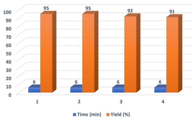
Fig. 8 The reusability of the PC/Fe<sub>3</sub>O<sub>4</sub> nanocomposite.
