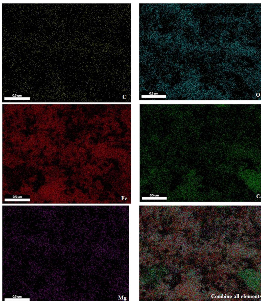
Fig. 3 SEM coupled EDX (SEM mapping) of the PC/Fe<sub>3</sub>O<sub>4</sub> nanocomposite.
