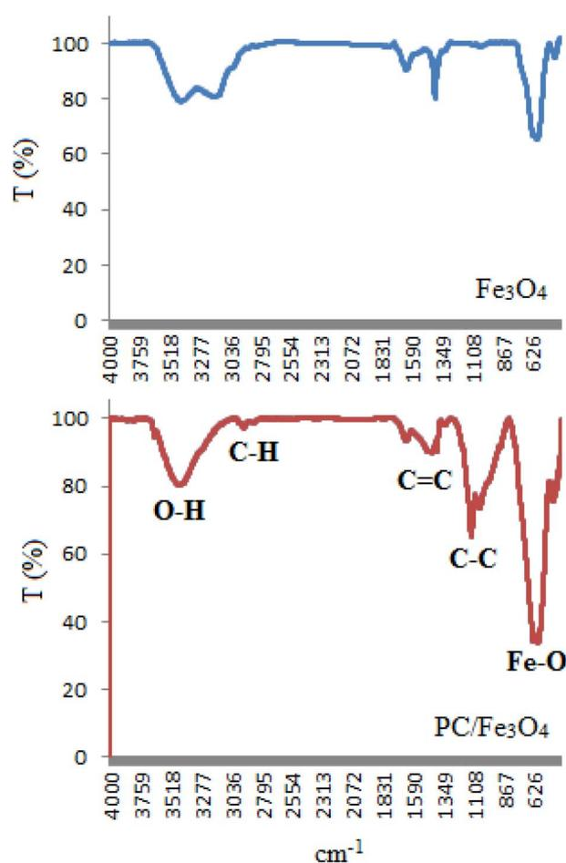
Fig. 1 FT-IR spectrum of the PC/Fe<sub>3</sub>O<sub>4</sub> nanocomposite in comparison with Fe<sub>3</sub>O<sub>4</sub>.
