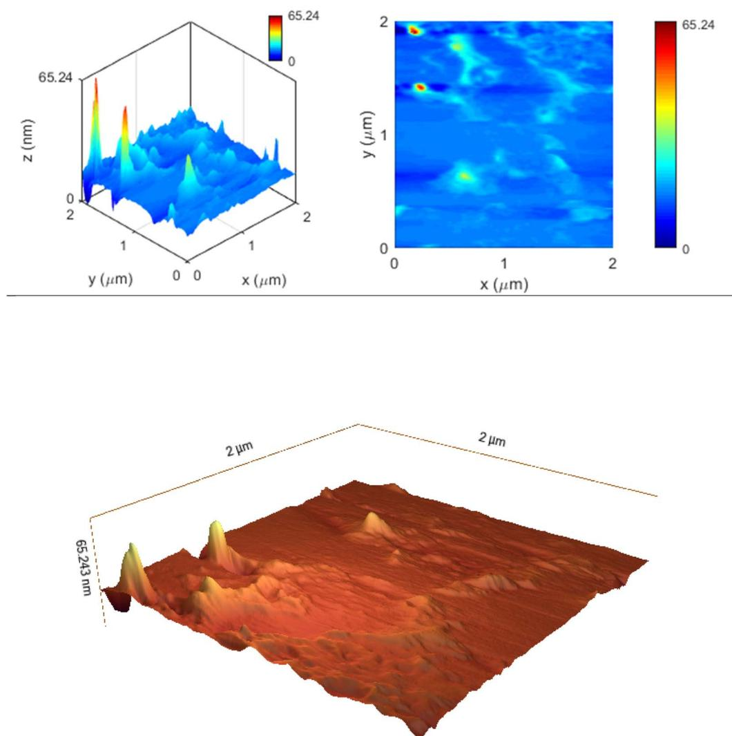
Fig. 5 Atomic force microscopy (AFM) analysis of the PC/Fe<sub>3</sub>O<sub>4</sub> nanocomposite.
