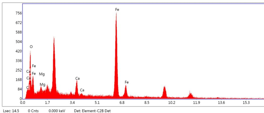
Fig. 2 Energy-dispersive X-ray spectroscopy (EDX) of the PC/Fe<sub>3</sub>O<sub>4</sub> nanocomposite.
