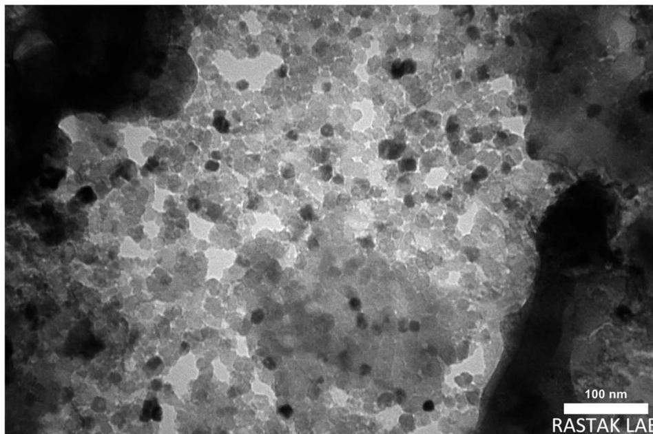
Fig. 6 TEM image of the PC/Fe<sub>3</sub>O<sub>4</sub> nanocomposite.
