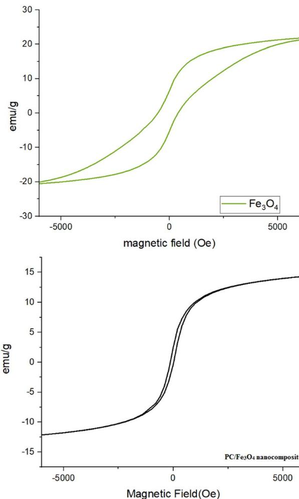
Fig. 7 Vibrating sample magnetometer (VSM) analysis of the PC/Fe<sub>3</sub>O<sub>4</sub> nanocomposite compared with Fe<sub>3</sub>O<sub>4</sub>.
