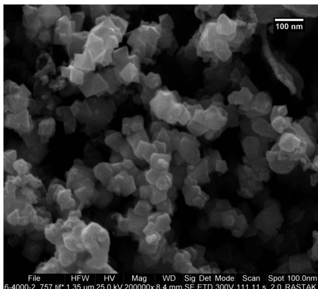
Fig. 4 SEM image of the PC/Fe<sub>3</sub>O<sub>4</sub> nanocomposite.
