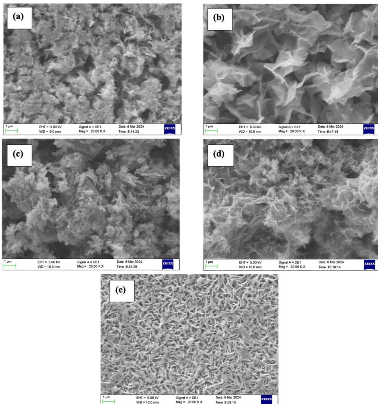
Fig. 12 SEM images of the electrodes processed in (a) Na<sub>2</sub>SO<sub>4</sub>, (b) NaCl, (c) Li<sub>2</sub>SO<sub>4</sub>, (d) K<sub>2</sub>SO<sub>4</sub>, and (e) MgSO<sub>4</sub> for 500 CV cycles at 50 mV s<sup>-1</sup>.
