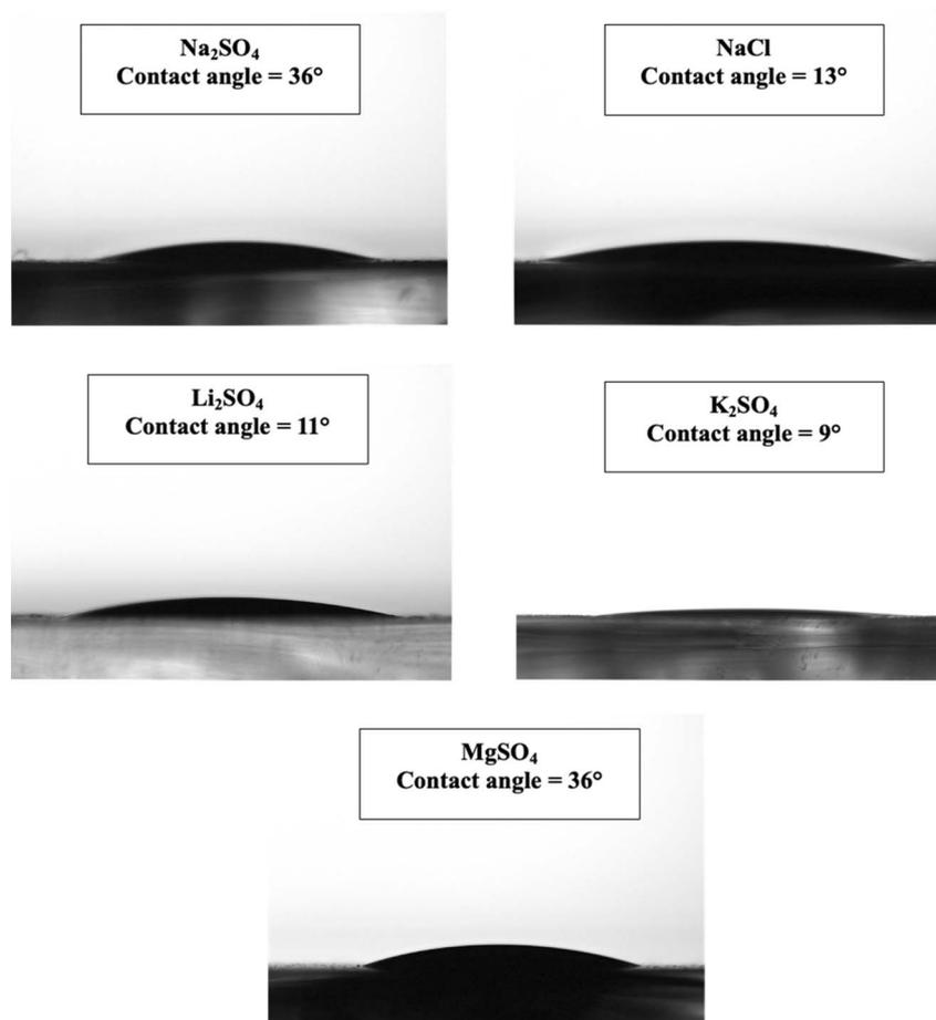
Fig. 13 Contact angle measurements of the electrodes processed in (a)  $\text{Na}_2\text{SO}_4$ , (b) NaCl, (c)  $\text{Li}_2\text{SO}_4$ , (d)  $\text{K}_2\text{SO}_4$  and (e)  $\text{MgSO}_4$  for 500 CV cycles at  $50 \text{ mV s}^{-1}$ .
