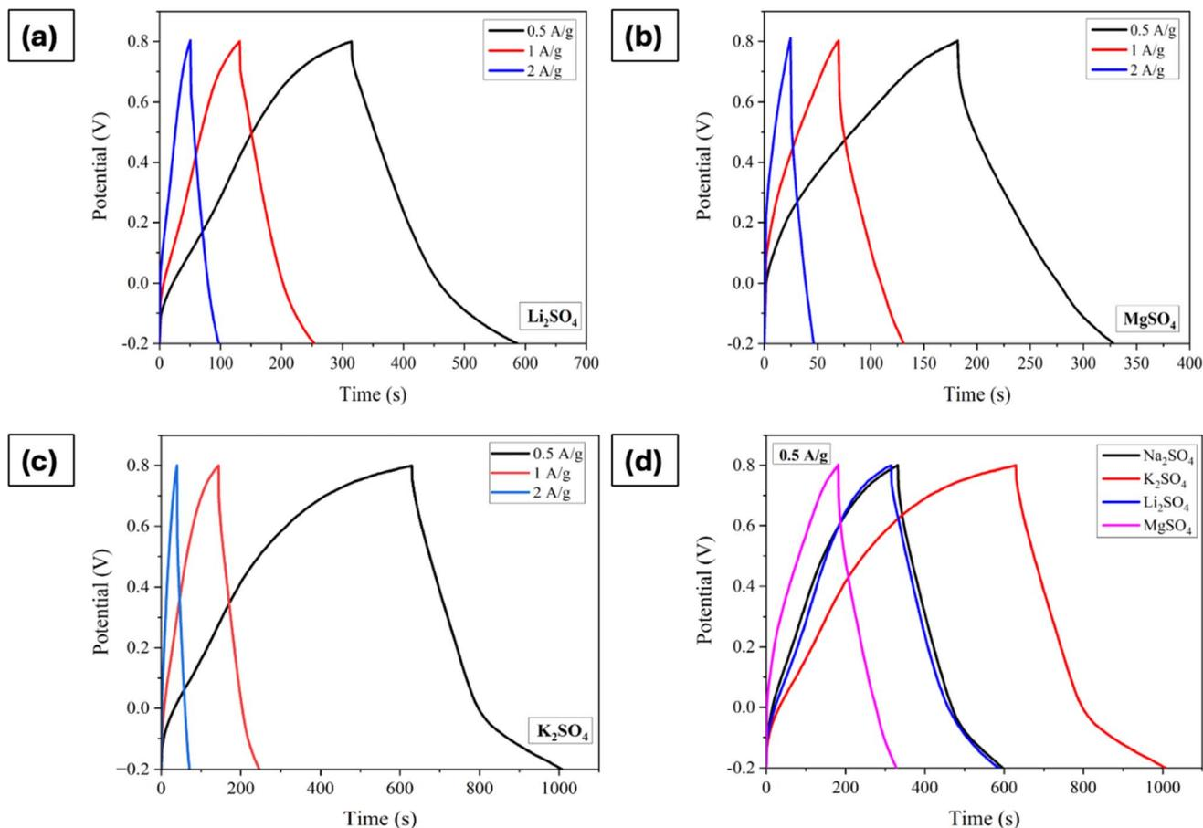
Fig. 7 GCD curves of  $\text{Mn}_3\text{O}_4$  thin film electrode in (a)  $\text{Li}_2\text{SO}_4$ , (b)  $\text{MgSO}_4$ , (c)  $\text{K}_2\text{SO}_4$ , and (d) comparison of GCDs at a current density of  $0.5 \text{ A g}^{-1}$ .
