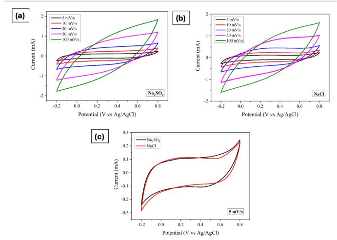
Fig. 2 Cyclic voltammograms of  $Mn_3O_4$  thin film electrode in (a)  $Na_2SO_4$ , and (b) NaCl. (c) Comparison of CVs at a scan rate of 5 mV s<sup>-1</sup>.
