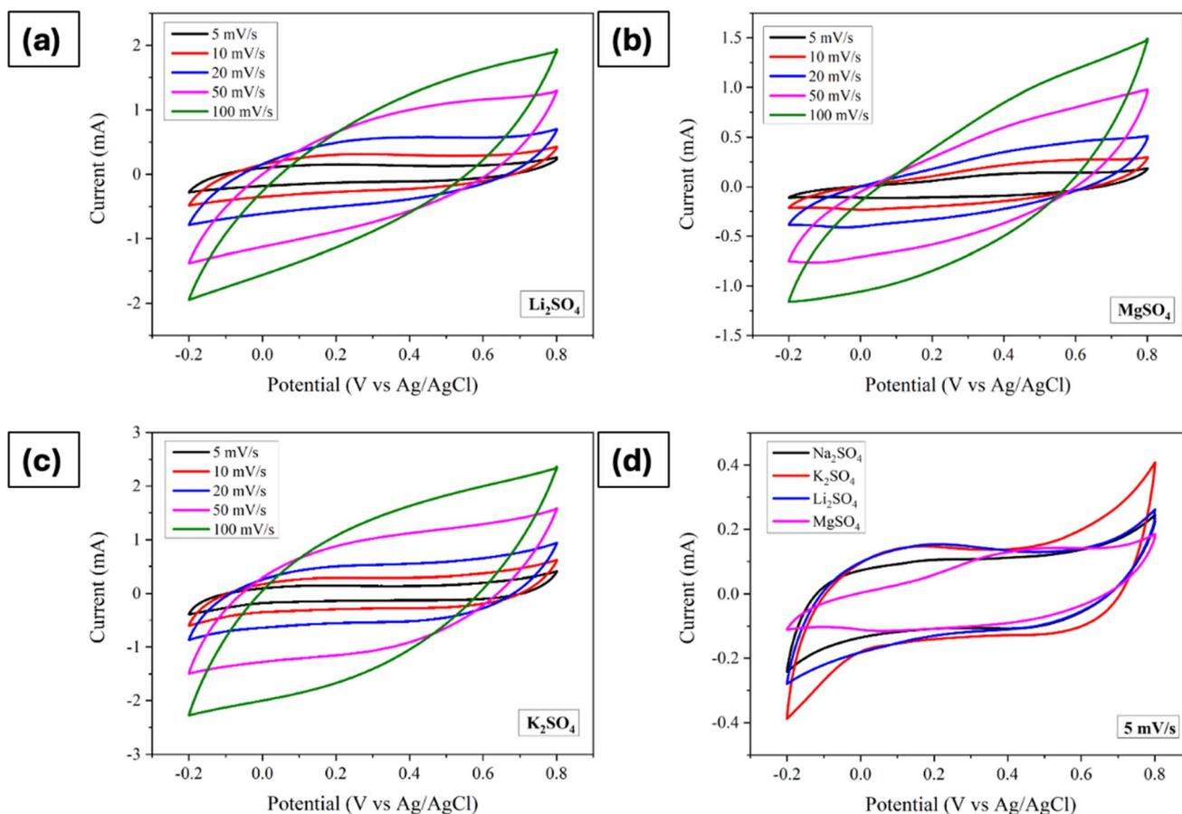
Fig. 5 Cyclic voltammograms of  $\text{Mn}_3\text{O}_4$  thin film electrode in (a)  $\text{Li}_2\text{SO}_4$ , (b)  $\text{MgSO}_4$ , (c)  $\text{K}_2\text{SO}_4$ , and (d) comparison of CVs at a scan rate of  $5 \text{ mV s}^{-1}$ .
