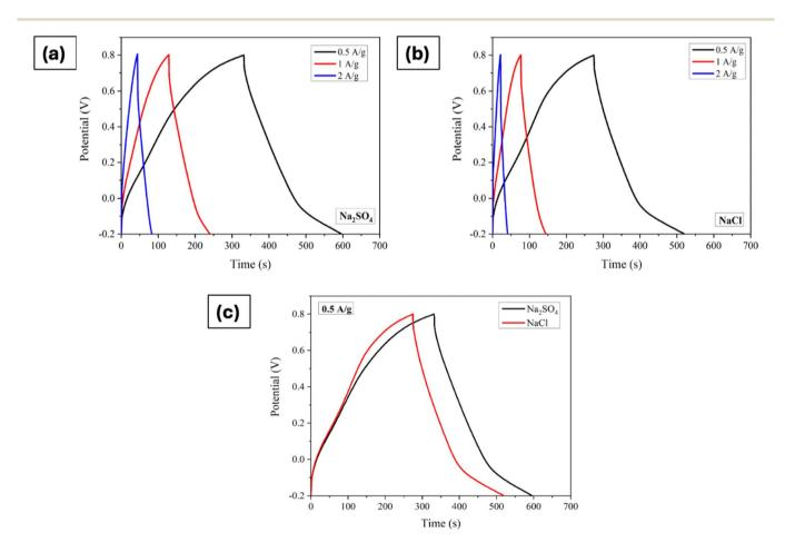
Fig. 4 Galvanostatic charge/discharge curves of  $Mn_3O_4$  thin film electrode in (a)  $Na_2SO_4$ , and (b) NaCl. (c) Comparison of GCDs at a current density of 0.5A  $g^{-1}$ .
