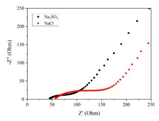
Fig. 3 Nyquist plots of Mn<sub>3</sub>O<sub>4</sub> thin film in Na<sub>2</sub>SO<sub>4</sub> and NaCl.
