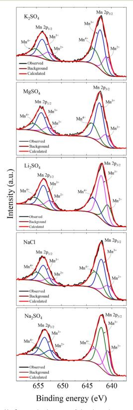
Fig. 11 Mn 2p core level spectra of the electrodes processed in different electrolytes.
