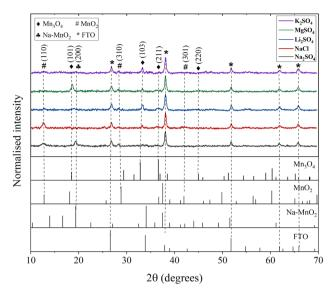
Fig. 8  $\,$  XRD patterns of  $\rm Mn_3O_4$  thin films after cycling in different electrolytes.
