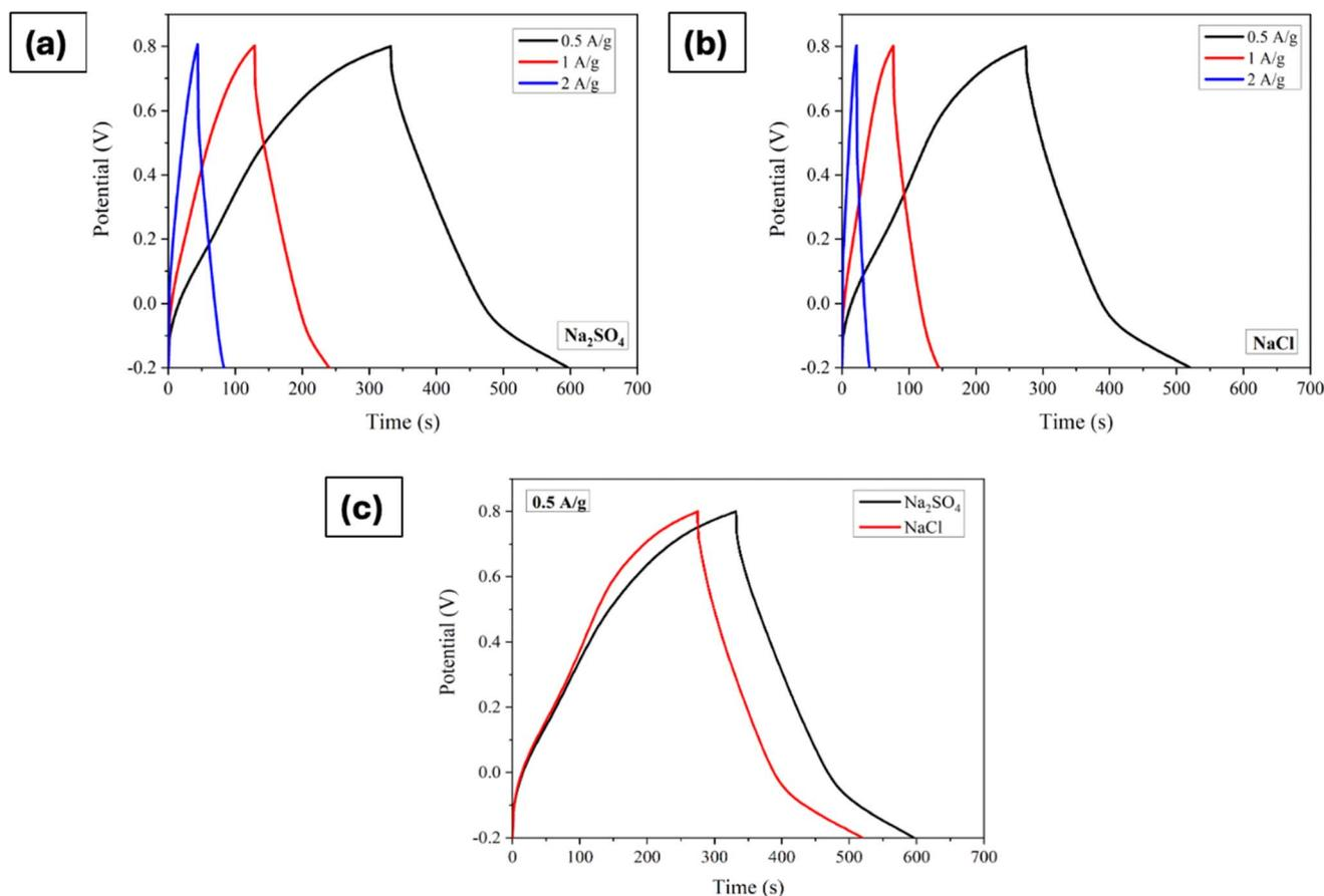
Fig. 4 Galvanostatic charge/discharge curves of  $\text{Mn}_3\text{O}_4$  thin film electrode in (a)  $\text{Na}_2\text{SO}_4$ , and (b)  $\text{NaCl}$ . (c) Comparison of GCDs at a current density of  $0.5 \text{ A g}^{-1}$ .
