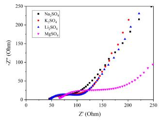
Fig. 6 Nyquist plots of  $\mathrm{Mn_3O_4}$  thin film in electrolytes with different cations.
