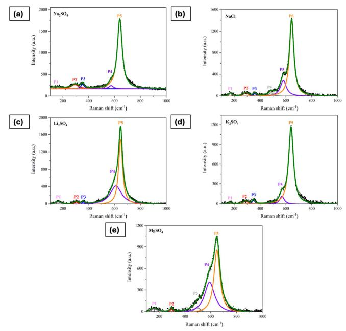
Fig. 9 Raman spectra of electrode processed in (a)  $Na_2SO_4$ , (b) NaCl, (c)  $Li_2SO_4$ , (d)  $K_2SO_4$ , and (e)  $MgSO_4$  for 500 CV cycles at 50 mV s<sup>-1</sup>.
