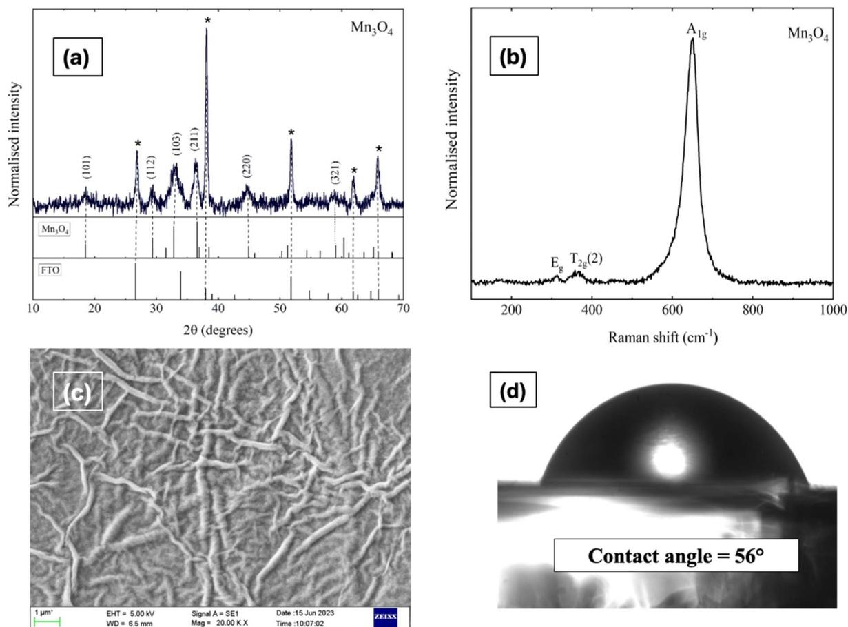
Fig. 1 (a) X-ray diffractogram, (b) Raman spectra, (c) SEM micrograph (magnification: 20KX), and (d) contact angle measurement of Mn<sub>3</sub>O<sub>4</sub> thin film electrode.
