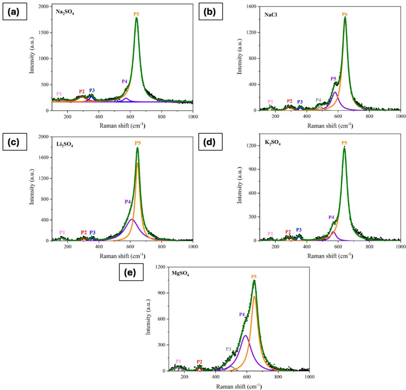
Fig. 9 Raman spectra of electrode processed in (a)  $\text{Na}_2\text{SO}_4$ , (b)  $\text{NaCl}$ , (c)  $\text{Li}_2\text{SO}_4$ , (d)  $\text{K}_2\text{SO}_4$ , and (e)  $\text{MgSO}_4$  for 500 CV cycles at  $50 \text{ mV s}^{-1}$ .
