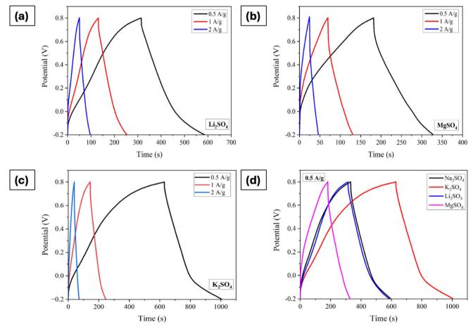
Fig. 7 GCD curves of Mn<sub>3</sub>O<sub>4</sub> thin film electrode in (a) Li<sub>2</sub>SO<sub>4</sub>, (b) MgSO<sub>4</sub>, (c) K<sub>2</sub>SO<sub>4</sub>, and (d) comparison of GCDs at a current density of 0.5 A g<sup>-1</sup>.
