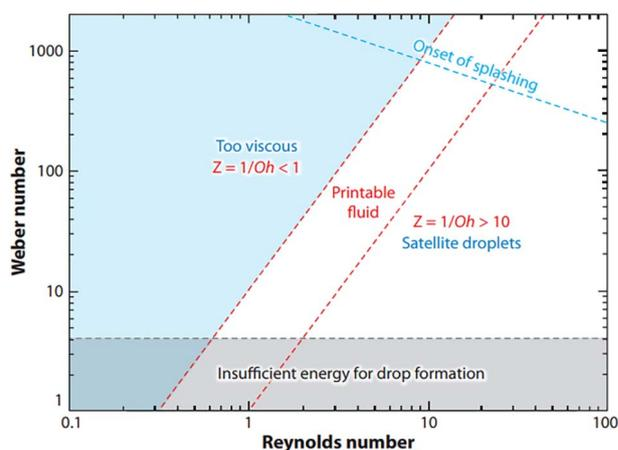
Fig. 16 The allows stable printing range.<sup>41</sup>
