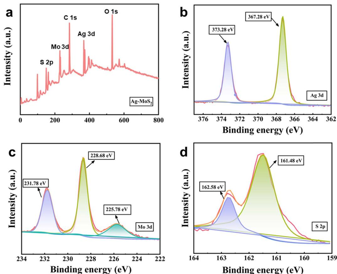
Fig. 2 (a) The XPS survey of Ag–MoS<sub>2</sub> hybrid material. The high-resolution XPS spectra of Ag 3d (b) Mo 3d (c) and (d) S 2p signals for Ag–MoS<sub>2</sub>.
