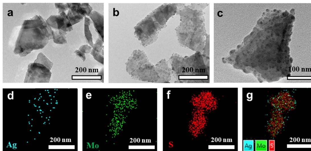
Fig. 1 (a) Typical TEM image for the prepared MoS<sub>2</sub> nanosheet. (b and c) Typical TEM images for the prepared Ag–MoS<sub>2</sub> nanocomposite. EDS elemental mapping results of Ag (d), Mo (e), S (f) and overlapping (g).
