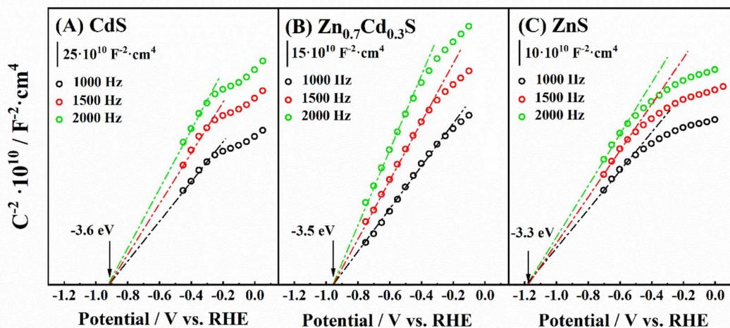
Fig. 4 Mott–Schottky obtained by measuring the capacitance at 1000, 1500 and 2000 Hz in a 0.1 M  $\text{Na}_2\text{SO}_3$  solution by EIS for (A) ZnS, (B) CdS and (C)  $\text{Zn}_{0.7}\text{Cd}_{0.3}\text{S}$ .
