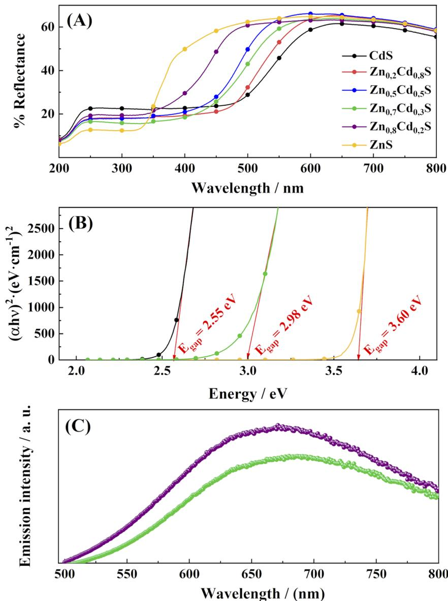
Fig. 3 (A) Diffuse reflectance spectra of the Zn<sub>1-x</sub>Cd<sub>x</sub>S solid-state photocatalysts, with x = 0 to 1. (B) Tauc plot for determining the bandgap for Zn<sub>0.7</sub>Cd<sub>0.3</sub>S, CdS and ZnS. (C) Photoluminescence spectra for Zn<sub>0.7</sub>Cd<sub>0.3</sub>S (green dots) and Zn<sub>0.8</sub>Cd<sub>0.2</sub>S (purple dots) samples obtained under excitation at 440 nm, corresponding to the mean bandgap separation energy of both samples.
