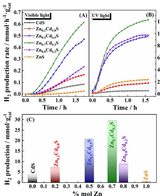
Fig. 7 Hydrogen production rate vs. time for the  $\text{Zn}_{1-x}\text{Cd}_x\text{S}$  catalysts with different zinc contents using (A) visible and (B) UV light. (C) Maximum hydrogen production rate of  $\text{Zn}_{1-x}\text{Cd}_x\text{S}$  vs. zinc content, using UV radiation.
