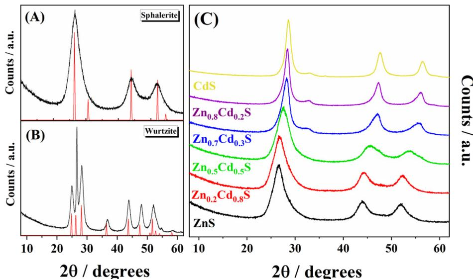
Fig. 1 X-ray diffraction patterns for (A) experimental (black) and reference (red) (ICSD #81925) CdS with sphalerite structure. (B) Experimental (black) and reference (red) CdS wurtzite structure (ICSD #154187) (C) X-ray diffraction patterns of the synthesized  $Zn_{1-x}Cd_xS$ , with  $x$  values ranging from 0 to 1.
