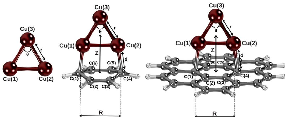
Fig. 1 Complexes under investigation at the equilibrium geometries (see Section 2 and the ESI† for the computational details). Z is defined as the distance between the centers of mass of Cu<sub>3</sub> and the benzene and coronene molecules, lying along the plotted axis.
