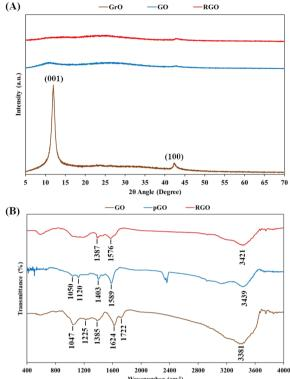
Fig. 4 (A) XRD patterns of graphite oxide (GrO), graphene oxide (GO) and reduced graphene oxide (RGO). (B) FTIR spectra of graphene oxide (GO), partially reduced graphene oxide (pGO) and reduced graphene oxide (RGO).
