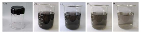
Fig. 3 As-prepared RGO hydrogel (A) and dispersions of RGO in water at concentrations of 9 ppm (B), 7 ppm (C), 5 ppm (D) and 3 ppm (E).
