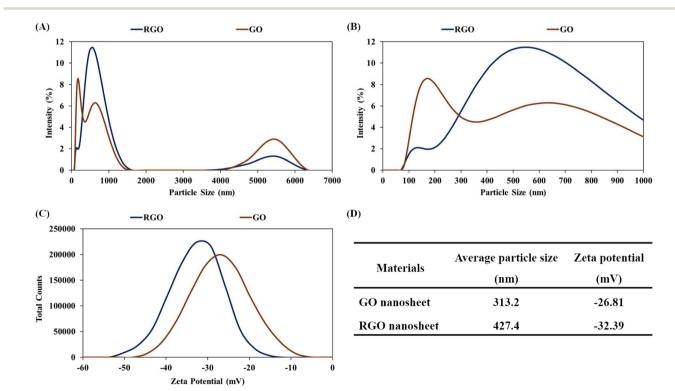
Fig. 8 (A) Particle size analysis of GO and RGO nanosheets in water solutions (concentration of 7 ppm). (B) Expended view of the particle size distribution in the range of 0-1000 nm. (C) Graph of the zeta potentials of the GO and RGO nanosheets. (D) Summary of average particle size and zeta potential of the GO and RGO nanosheets.
