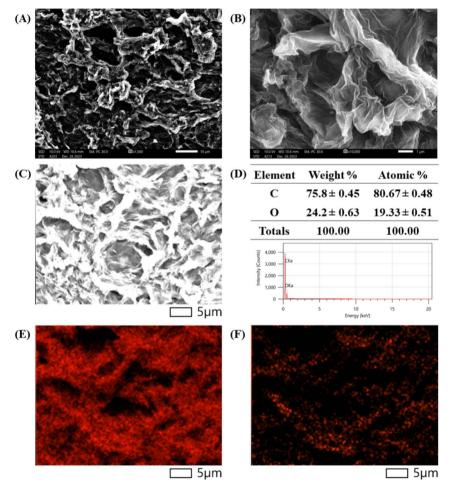
Fig. 7 (A and B) SEM images of the three-dimensional assembly of the RGO hydrogel with scale bars of 10  $\mu$ m and 1  $\mu$ m, respectively. (C) SEM image of the RGO structure in EDS analysis. (D) EDS spectrum and elemental composition of carbon and oxygen in the RGO structure. (E and F) Elemental mapping of carbon atoms and oxygen atoms, respectively, on the RGO structure.
