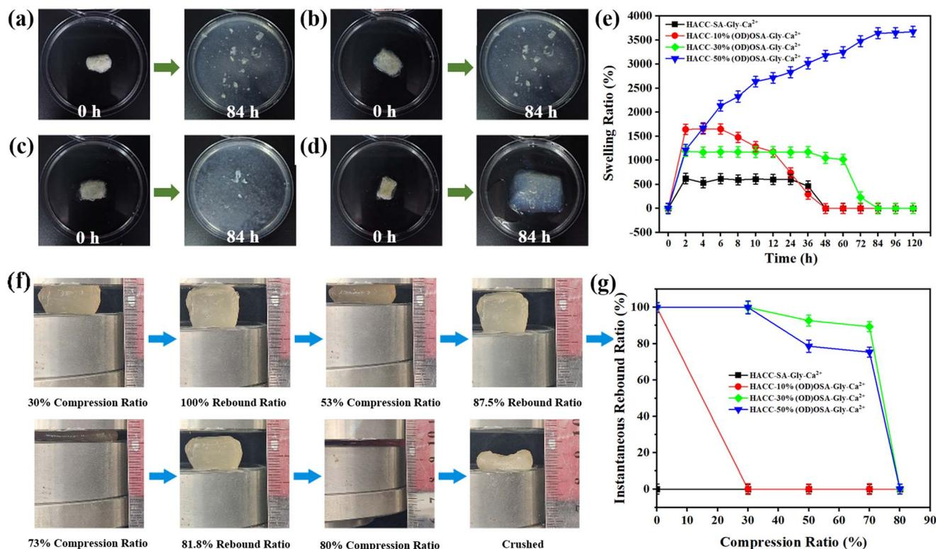
Fig. 7 (a) HACC-SA-Gly-Ca<sup>2+</sup>, (b) HACC-10%(OD)OSA-Gly-Ca<sup>2+</sup>, (c) HACC-30%(OD)OSA-Gly-Ca<sup>2+</sup>, and (d) HACC-50%(OD)OSA-Gly-Ca<sup>2+</sup> dry gels were soaked for 84 h, respectively; (e) swelling rate curves of the four kinds of hydrogels; (f) the process of HACC-50%(OD)OSA-Gly-Ca<sup>2+</sup> hydrogel compression experiment; (g) variation of compressive rebound of the four kinds of hydrogels.
