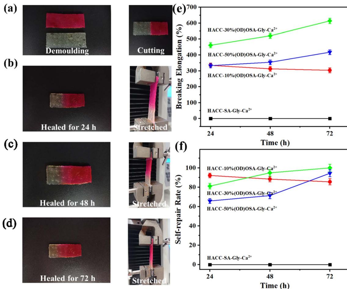
Fig. 6 (a)–(d) Self-healing process and tensile test of the HACG-50%(OD)OSA-Gly-Ca<sup>2+</sup> hydrogel after self-healing; (e) elongation of four kinds of hydrogels after a period (72 h) of self-healing; (f) self-repair rate of four kinds of hydrogels after a period (72 h) of self-healing.
