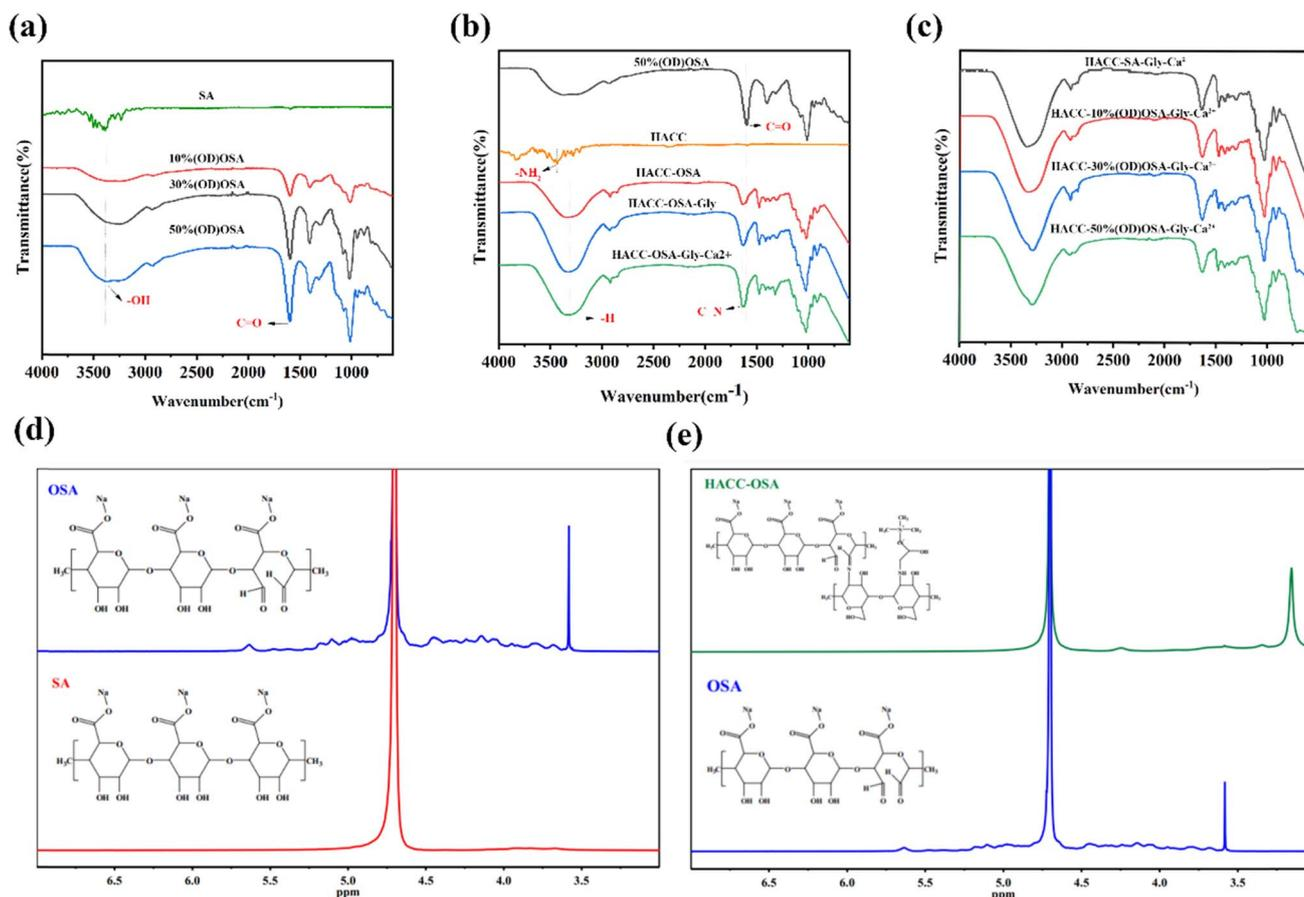
Fig. 2 (a–c) FTIR spectra of (a) SA, 10%(OD)OSA, 30%(OD)OSA, and 50%(OD)OSA; (b) hydrogels of 50(OD)%OSA, HACC, HACC-50%(OD)OSA, HACC-50%(OD)OSA-Gly, and HACC-50%(OD)OSA-Gly-Ca<sup>2+</sup>; (c) and the self-healing hydrogels of HACC-SA-Gly-Ca<sup>2+</sup>, HACC-10%(OD)OSA-Gly-Ca<sup>2+</sup>, HACC-30%(OD)OSA-Gly-Ca<sup>2+</sup>, HACC-50%(OD)OSA-Gly-Ca<sup>2+</sup>. (d) and (e) The <sup>1</sup>H NMR spectra of (d) SA and OSA; (e) HACC-OSA and OSA.
