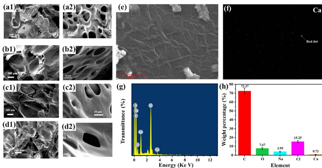
Fig. 3 SEM images of (a) HACC-SA-Gly-Ca<sup>2+</sup>, (b) HACC-10%(OD)OSA-Gly-Ca<sup>2+</sup>, (c) HACC-30%(OD)OSA-Gly-Ca<sup>2+</sup>, and (d) HACC-50%(OD)OSA-Gly-Ca<sup>2+</sup> hydrogels; (e) SEM image with local magnification of 8000× of the HACC-50%(OD)OSA-Gly-Ca<sup>2+</sup> hydrogel; (f) calcium distribution, indicated by red dot; (g) EDS analysis diagram of HACC-50%(OD)OSA-Gly-Ca<sup>2+</sup> hydrogel; (h) elemental quantitative analysis.
