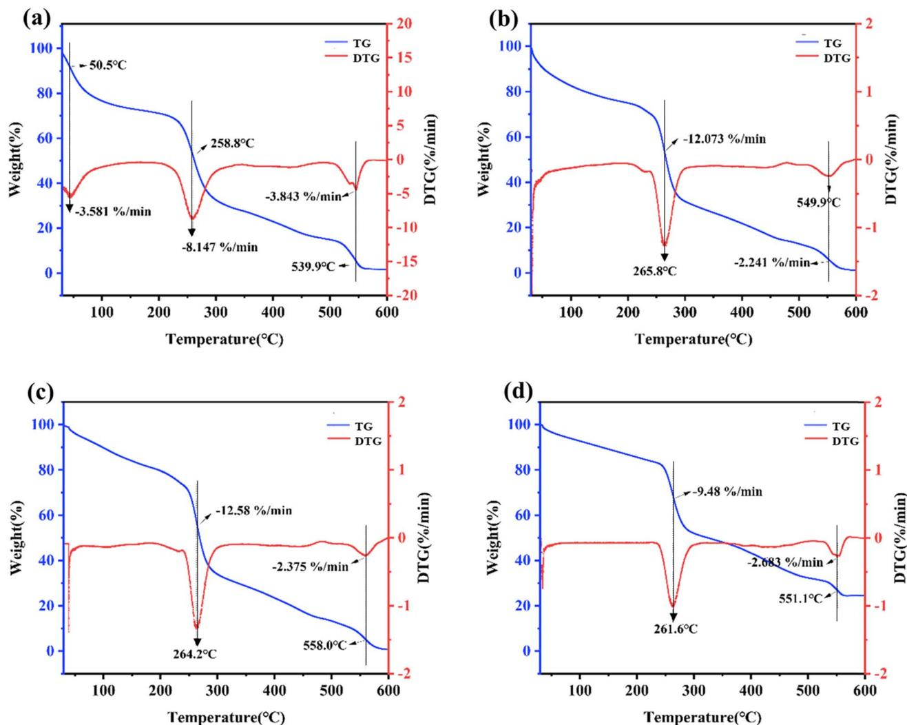
Fig. 4 TG and DTG curves of the four different kinds of hydrogels: (a) HACC-SA-Gly- $\text{Ca}^{2+}$ ; (b) HACC-10%(OD)OSA-Gly- $\text{Ca}^{2+}$ ; (c) HACC-30%(OD)OSA-Gly- $\text{Ca}^{2+}$ ; (d) HACC-50%(OD)OSA-Gly- $\text{Ca}^{2+}$ .
