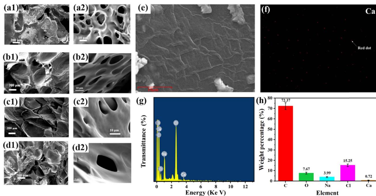
Fig. 3 SEM images of (a) HACC-SA-Gly-Ca<sup>2+</sup>, (b) HACC-10%(OD)OSA-Gly-Ca<sup>2+</sup>, (c) HACC-30%(OD)OSA-Gly-Ca<sup>2+</sup>, and (d) HACC-50%(OD)OSA-Gly-Ca<sup>2+</sup> hydrogels; (e) SEM image with local magnification of 8000 $\times$  of the HACC-50%(OD)OSA-Gly-Ca<sup>2+</sup> hydrogel; (f) calcium distribution, indicated by red dot; (g) EDS analysis diagram of HACC-50%(OD)OSA-Gly-Ca<sup>2+</sup> hydrogel; (h) elemental quantitative analysis.
