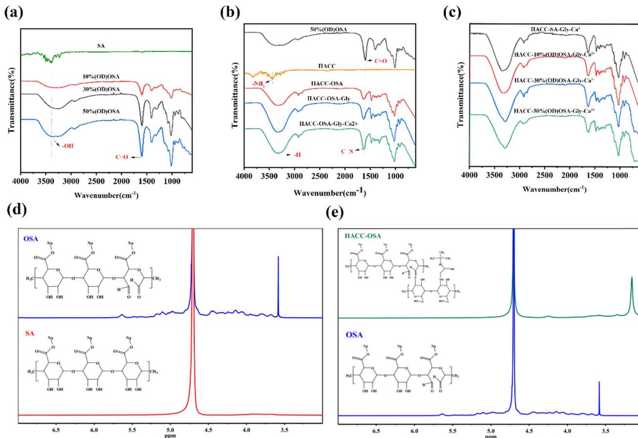
Fig. 2 (a–c) FTIR spectra of (a) SA, 10%(OD)OSA, 30%(OD)OSA, and 50%(OD)OSA; (b) hydrogels of 50(OD)%OSA, HACC, HACC-50%(OD)OSA, HACC-50%(OD)OSA-Gly, and HACC-50%(OD)OSA-Gly-Ca<sup>2+</sup>; (c) and the self-healing hydrogels of HACC-SA-Gly-Ca<sup>2+</sup>, HACC-10%(OD)OSA-Gly-Ca<sup>2+</sup>, HACC-30%(OD)OSA-Gly-Ca<sup>2+</sup>, HACC-50%(OD)OSA-Gly-Ca<sup>2+</sup>. (d) and (e) The <sup>1</sup>H NMR spectra of (d) SA and OSA; (e) HACC-OSA and OSA.
