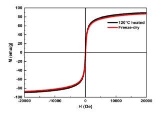
Fig. 5 Magnetic hysteresis loops of SPIONs with freeze-dry and 120  $^{\circ}$  C. heated
