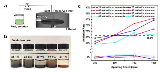
Fig. 1 (a) Schematic illustration of MFR. (b) Photos of products with different oxidation rates obtained at different conditions (from left to right, the samples are 4, 3, 5, 15, and 14). (c) The oxidation rates of products obtained under different spinning speeds, feeding concentrations and with/ without ammonia.
