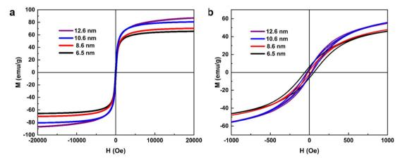
(a) Magnetic hysteresis loop of SPIONs with different sizes. (b) Magnification of the hysteresis loop near zero fields of (a).
