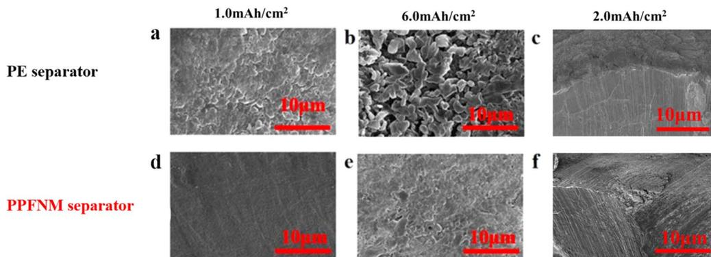
Fig. 3 Li–Li electrode of a battery using PE separator and PPFNM separator, at a current density of 2.0 mA cm<sup>-2</sup>, SEM images of the surface and cross-section (c and f) of 1.0 mA h cm<sup>-2</sup> (a and d) and 6.0 mA h cm<sup>-2</sup> (b and e) were deposited, respectively.
