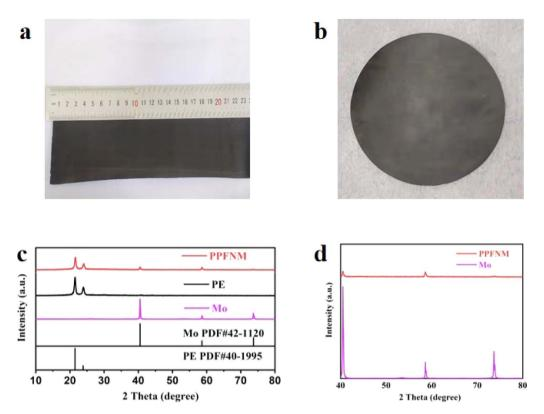
Fig. 1 (a and b) PPFNM separator, (c and d) XRD pattern of PPFNM separator.
