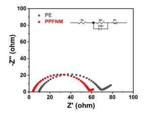
Fig. 6 EIS diagram for Li-Li symmetric cells using PE separator and PPFNM separator
