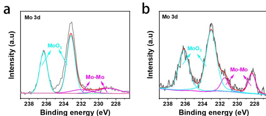
Fig. 10 (a and b) XPS spectra of separator Mo 3d before and after cycling.
