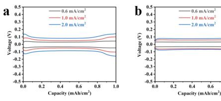
Charge and discharge curves of Li-Li symmetric cells using PE separator (a) and PPFNM separator (b).
