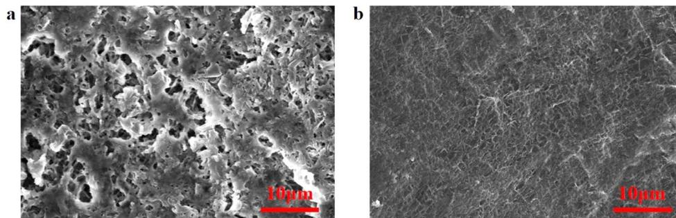
Fig. 7 Li–Li symmetric cell using PE separator (a) and PPFNM separator (b) at  $2.0 \text{ mA cm}^{-2}$ ,  $2.0 \text{ mA h cm}^{-2}$ , SEM image of a lithium electrode sheet after 70 cycles.
