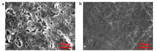
Fig. 7 Li-Li symmetric cell using PE separator (a) and PPFNM separator (b) at 2.0 mA cm<sup>-2</sup>, 2.0 mA h cm<sup>-2</sup>, SEM image of a lithium electrode sheet after 70 cycles.
