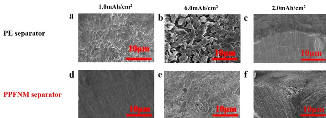
Fig. 3 Li–Li electrode of a battery using PE separator and PPFNM separator, at a current density of  $2.0 \text{ mA cm}^{-2}$ , SEM images of the surface and cross-section (c and f) of  $1.0 \text{ mA h cm}^{-2}$  (a and d) and  $6.0 \text{ mA h cm}^{-2}$  (b and e) were deposited, respectively.
