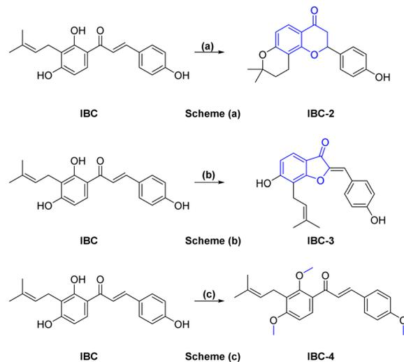
Scheme 1 Reagents and conditions: (a) 10% aq. NaOH, MeOH : H<sub>2</sub>O (1 : 1), 4 h, rt, then 50% H<sub>2</sub>SO<sub>4</sub> dropwise, yield 60%; (b) Hg(OAc)<sub>2</sub>, pyridine, reflux at 110 °C, 5 h, yield 70%; (c) CH<sub>3</sub>I, NaH, DMF, 0 °C–rt, 3 h, yield 75%.
