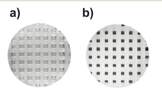
Fig. 3 Microscope picture of 3D Insert  $^{\text{TM}}$  polycaprolactone (PCL) scaffolds with (a) offset and (b) aligned fibres.
