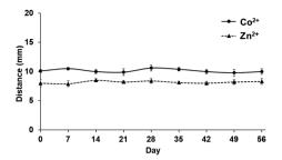
Fig. 6 Stability study of the predeposited reagent on DµPADs stored at ambient temperature for the determination of  $Co^{2+}$  and  $Zn^{2+}$ .
