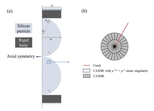
Fig. 10 Two-particle model: (a) schematic of the axisymmetric model with geometric parameters, and (b) the mesh refinement near the crack tip.
