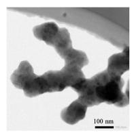
Fig. 1 TEM image of silicon nanoparticles.
