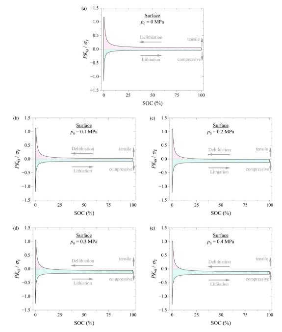
Fig. 6 Variation of hoop stress at the surface of the spherical electrode with SOC during a lithiation-delithiation cycle under the action of different compressions of (a) 0, (b) 0.1, (c) 0.2, (d) 0.3, and (e) 0.4 MPa. The pink region corresponds to the tensile state, and the cyan region corresponds to the compressive state.
