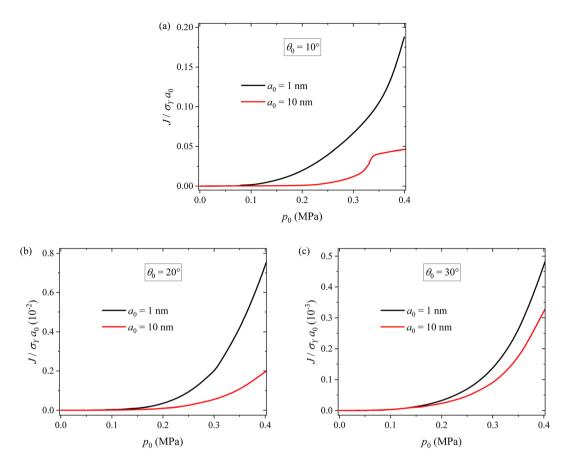
Fig. 9 Variations of *J*-integral at the crack tip with external pressure for two different crack sizes and three different inclination angles of (a)  $\theta_0 = 10^\circ$ , (b)  $\theta_0 = 20^\circ$  and (c)  $\theta_0 = 30^\circ$ .
