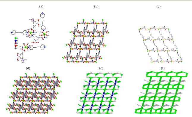
Fig. 5 Structure of 5. (a) Coordination environment at nickel( $\square$ ) atoms. (b) Three-dimensional framework along the c axis. (c) Two-dimensional metal-organic network along the b axis. (d) 3D + 2D interpenetrated frameworks along the c axis. (e) Topological representation of the framework along the c axis. (f) Two 3D + 2D interpenetrated frameworks shown by different colours (green and gray).
