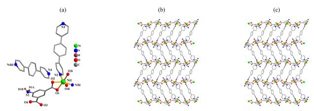
Fig. 4 Structure of 4. (a) Coordination environment at the nickel(II) atom. (b) The two-dimensional layer viewed along the a axis. (c) Sheet exhibiting a **new** topology, viewed along the a axis.
