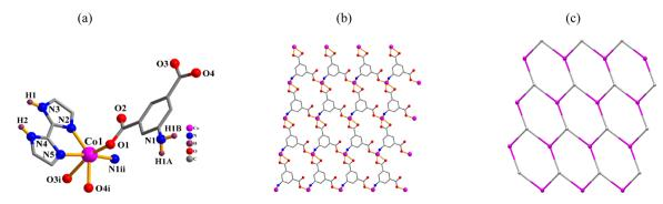
Fig. 1 Structure of CP 1. (a) Coordination environment at cobalt( $\square$ ) atom. (b) The two-dimensional layer viewed along the c axis. (c) The sheet exhibiting a **hcb** topology, observed along the c axis.
