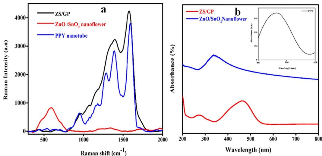
Fig. 2 Raman and UV-visible spectra of PPY nanotubes, ZnO/SnO<sub>2</sub> nanoflower, and ZS/GP nanocomposites.
