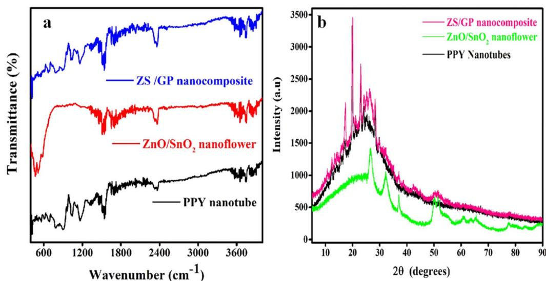
Fig. 1 (a) FTIR and (b) XRD spectra of PPY nanotubes, ZnO/SnO<sub>2</sub> nanoflower, and ZS/GP nanocomposites.
