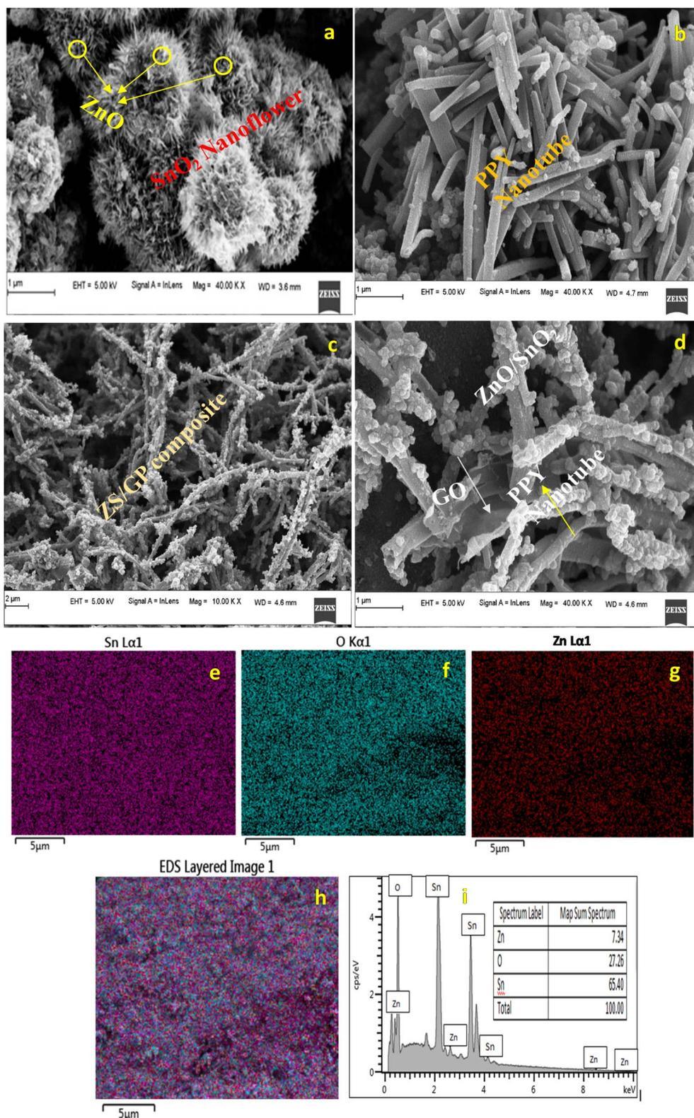
Fig. 3 FE-SEM images of PPY nanotubes (a), ZnO/SnO<sub>2</sub> nanoflower (b), and ZS/GP nanocomposites at different resolutions (c and d), and EDS layered images of ZnO/SnO<sub>2</sub> nanoflower and elemental analysis (e–i).
