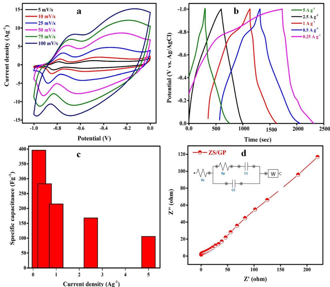
Fig. 5 (a) CV curves of ZS/GP nanocomposite at different scan rates from 5 to  $100 \text{ mV s}^{-1}$ , (b) GCD curves of ZS/GP nanocomposite at different current densities, (c) specific capacitance variation of ZS/GP at various current densities, and (d) Nyquist plots of ZnO/SnO<sub>2</sub> nanoflower (ZS/GP) nanocomposites with equivalent circuits.
