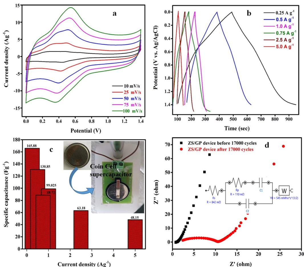
Fig. 6 (a) Cyclic voltammety curves of ASCs ZS/GP device at different scan rates from  $10 \text{ mV s}^{-1}$  to  $100 \text{ mV s}^{-1}$ , (b) GCD curves of ZS/GP device at different current densities, (c) specific capacitance variation of ASCs ZS/GP device at various current densities, and (d) Nyquist plots with equivalent circuit for the ZS/GP ASCs device.
