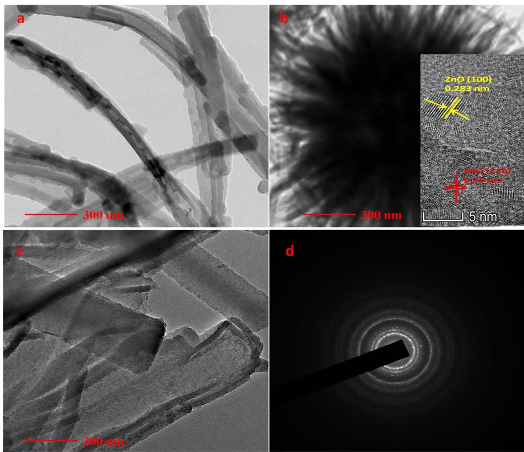
Fig. 4 TEM images of PPY nanotubes (a), ZnO/SnO<sub>2</sub> nanoflower (b), ZS/GP nanocomposites (c), and SAED pattern of ZS/GP nanocomposite (d).
