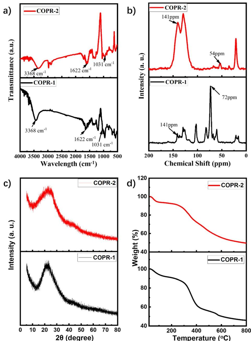
Fig. 1 Physical characterization of COPR-1 and COPR-2: (a) FTIR of COPR-1 and COPR-2. (b) Solid state  $^{13}\text{C}$  NMR of COPR-1 and COPR-2. (c) PXRD of COPR-1 and COPR-2. (d) TGA of COPR-1 and COPR-2.
