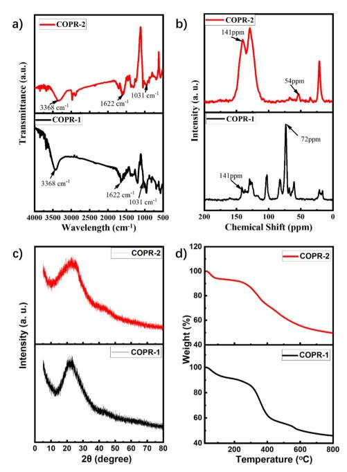
Fig. 1 Physical characterization of COPR-1 and COPR-2: (a) FTIR of COPR-1 and COPR-2. (b) Solid state <sup>13</sup>C NMR of COPR-1 and COPR-2. (c) PXRD of COPR-1 and COPR-2. (d) TGA of COPR-1 and COPR-2.
