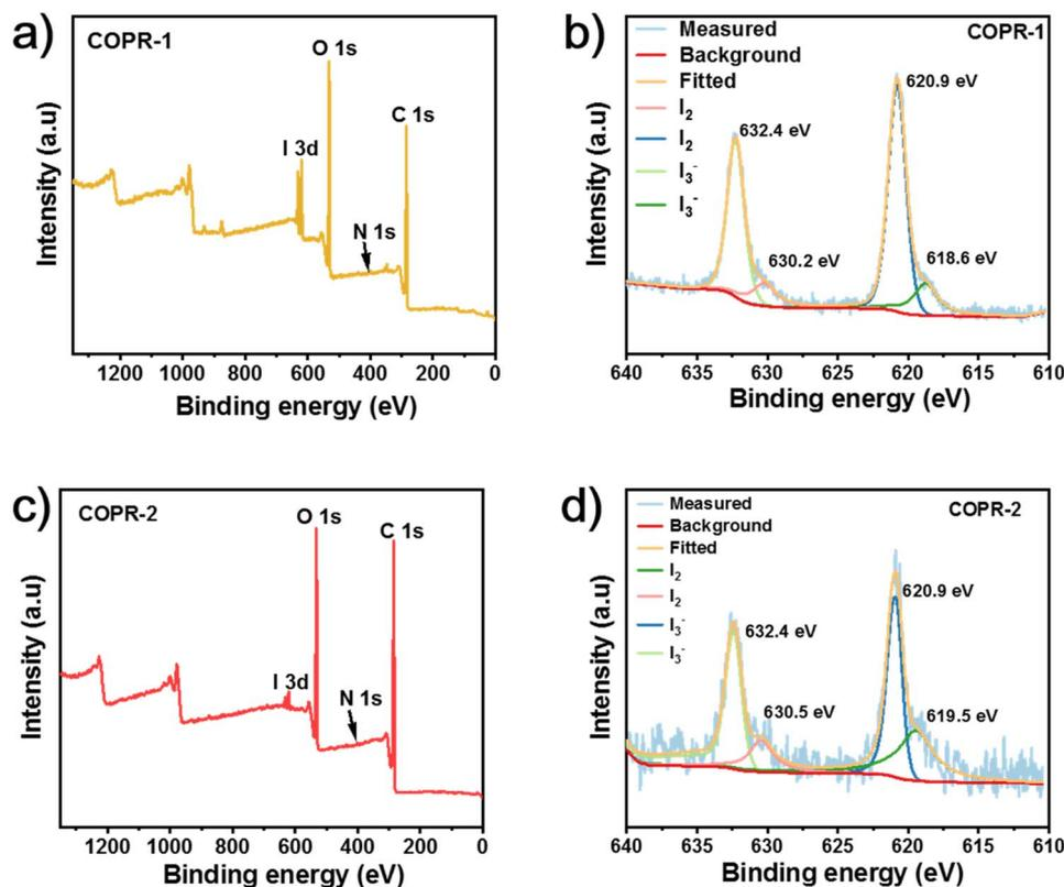
Fig. 4 (a) XPS survey spectra of COPR-1 after iodine adsorption. (b) XPS I3d spectra of COPR-1 after iodine adsorption. (c) XPS survey spectra of COPR-2 after iodine adsorption. (d) XPS I3d spectra of COPR-2 after iodine adsorption.
