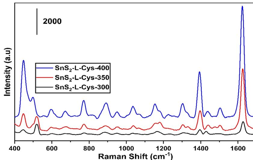
Fig. 11 SERS spectrum of SnS<sub>2</sub>-L-Cys annealed at different temperatures ranging from 300 to 400 °C.
