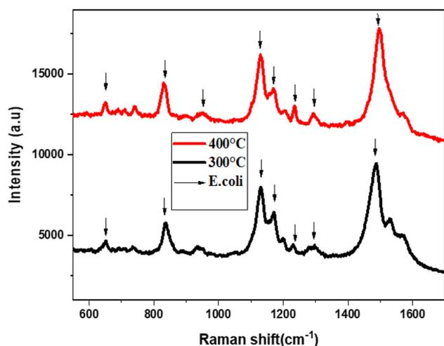
Fig. 7 The Raman spectra of *E. coli* using MoS<sub>2</sub>-L-Cys as SERS substrate annealed at temperatures 300 °C and 400 °C.
