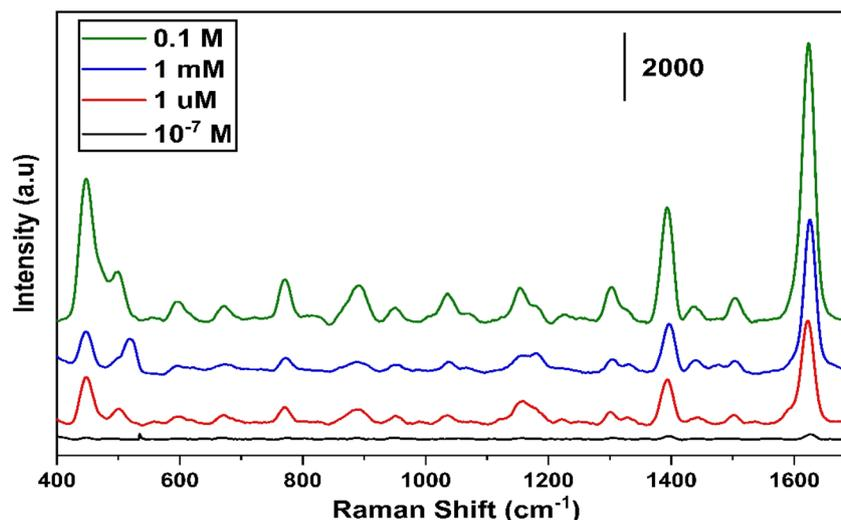
Fig. 12 Different concentrations of MB ranging from 0.1–10<sup>-7</sup> M measured on SnS<sub>2</sub> sample annealed at 400 °C.
