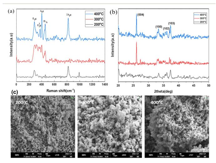
Fig. 2 (a) Raman spectroscopy, (b) XRD, and (c) SEM analysis of annealed  $MoS_2$  nanoparticles at various temperatures ranging from 200 to 400 °C.
