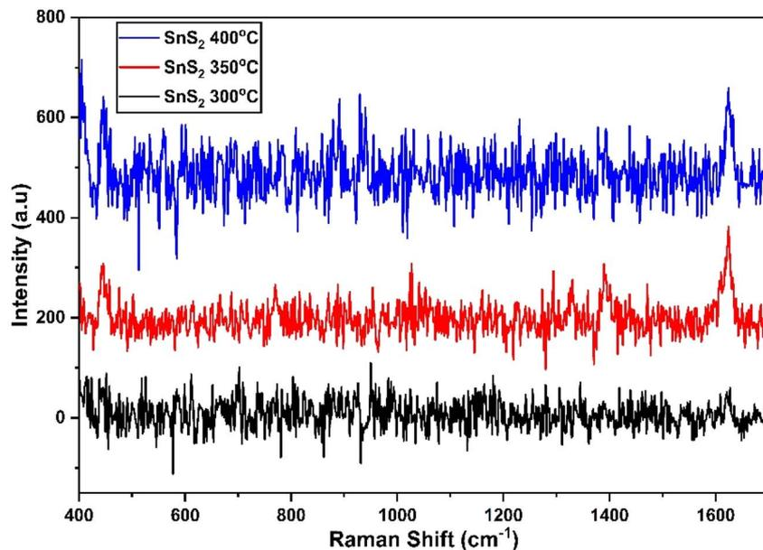
Fig. 9 SERS spectrum of SnS<sub>2</sub> annealed at temperatures ranging from 300 to 400 °C.
