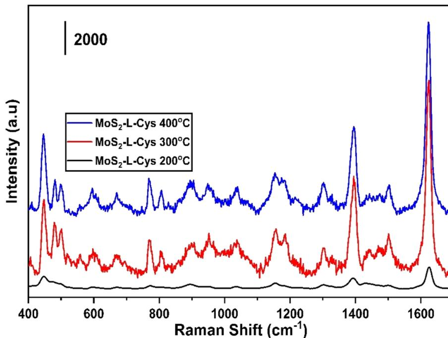
Fig. 5 The Raman spectra of MB using MoS<sub>2</sub>-L-Cys as SERS substrate annealed at temperatures 200 °C, 300 °C and 400 °C.
