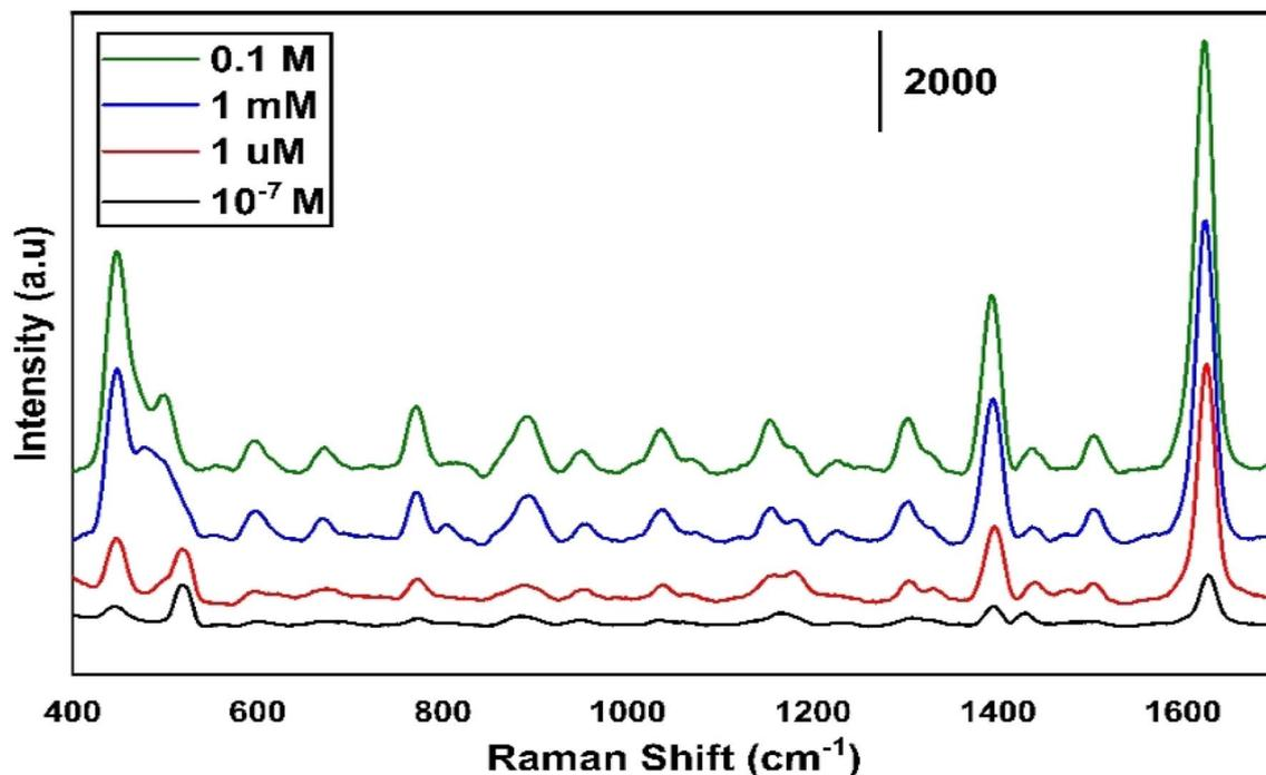
Fig. 6 Different concentration of MB ranging from 0.1–10<sup>-7</sup> M measured on MoS<sub>2</sub> sample annealed at 300 °C.
