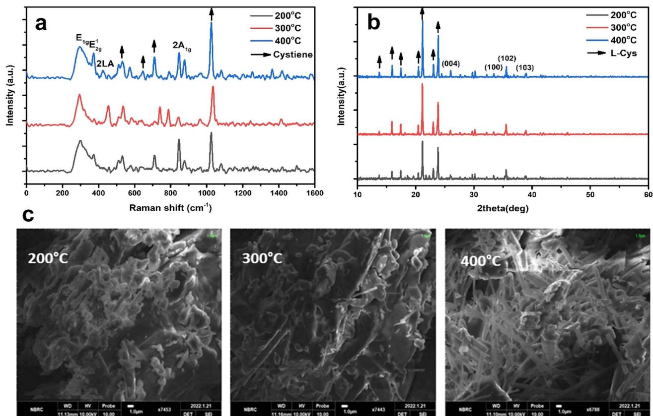
Fig. 4 (a)–(c) Raman spectroscopy data, XRD patterns, and SEM images of the MoS<sub>2</sub>-L-Cys NPs annealed at temperatures ranging from 200 to 400 °C. (a) Raman spectrum (b) XRD pattern (c) SEM images.
