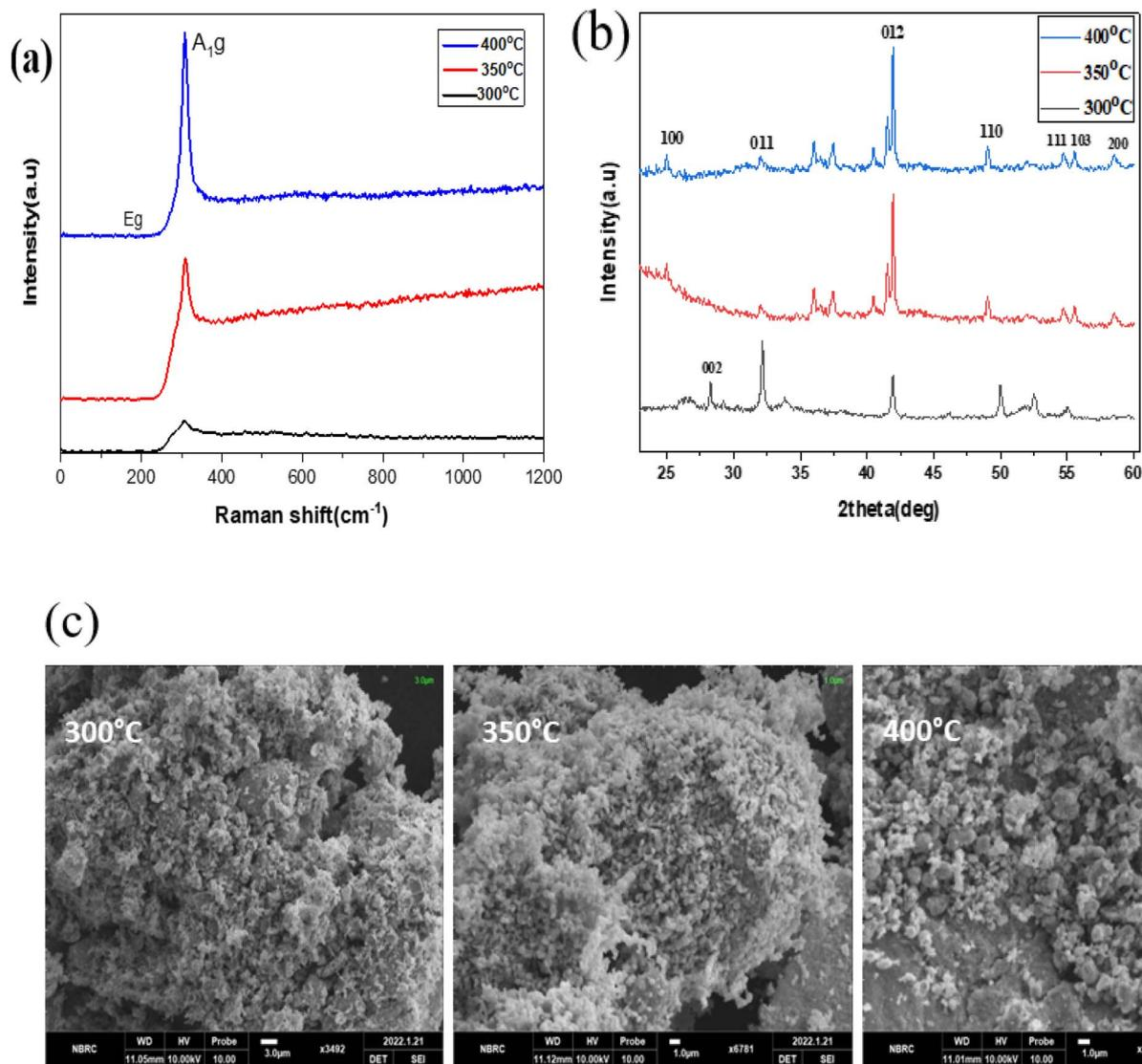
Fig. 8 (a)–(c) XRD, Raman spectroscopy data, and SEM images of the SnS<sub>2</sub> NPs annealed at different temperatures ranging from 300 to 400 °C.
