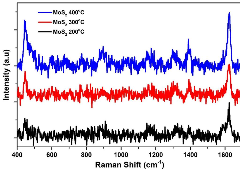
Fig. 3 SERS spectrum of MoS<sub>2</sub> annealed at temperatures ranging from 200 to 400 °C.
