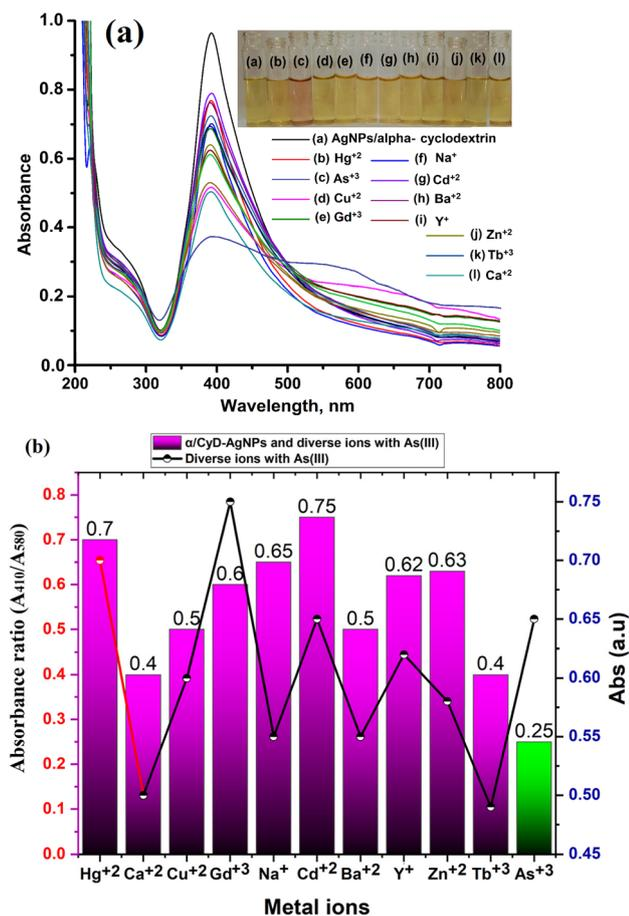
Fig. 9 (a) Photographic image of glass vials containing solution mixtures of dispersed  $\alpha$ /CyD-AgNPs and  $\alpha$ /CyD-AgNPs after the addition of different metal ions with their UV-Vis spectra using a colorimetric probe at pH 4.0 for 5 min reaction time at room temperature and (b) bar and line plots showing the absorbance ratio for the calculation of the tolerance for the respective metal ions.
