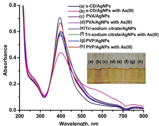
Fig. 2 Images of glass vials containing  $\alpha$ /CyD-AgNPs and  $\alpha$ /CyD-AgNPs with As(III) (a and b), PVA-capped AgNPs and PVA-capped AgNPs with As(III) (c and d), citrate-capped AgNPs and citrate-capped AgNPs with As(III) (e and f), CTAB-capped AgNPs and CTAB-capped AgNPs with As(III) (g and h), and their respective UV-Vis absorption spectra.
