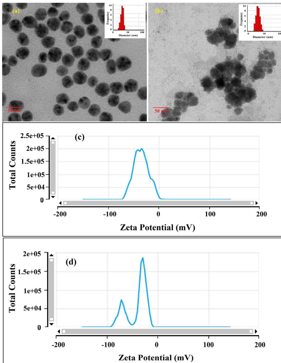
Fig. 4 TEM images of the dispersed  $\alpha$ /CyD-AgNPs (a) and aggregated  $\alpha$ /CyD-AgNPs after the addition of As(III) (b) with histogram plot (inset); zeta potential spectra of the dispersed  $\alpha$ /CyD-AgNPs (c) and aggregated  $\alpha$ /CyD-AgNPs after the addition of As(III) (d).
