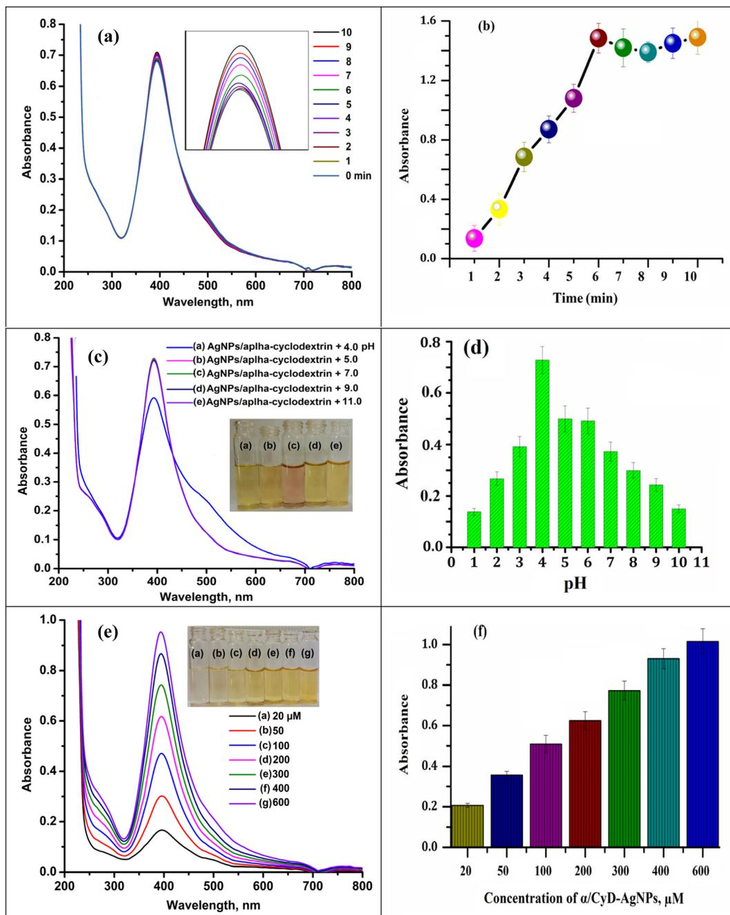
Fig. 10 Optimized conditions: (a and b) effect of the reaction time, (c and d) effect of pH and (e and f) effect of the concentration of  $\alpha$ /CyD-AgNPs for the detection of As(III) using UV-Vis spectrophotometry.
