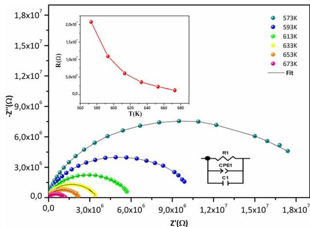
Fig. 7 Nyquist plot of  $\text{Sr}_2(\text{Sn}_{0.33}\text{Sb}_{0.33}\text{In}_{0.33})_2\text{O}_6$  at different temperatures and equivalent circuit of fitting data for the system. The resistance plot as a function of temperature in inset.
