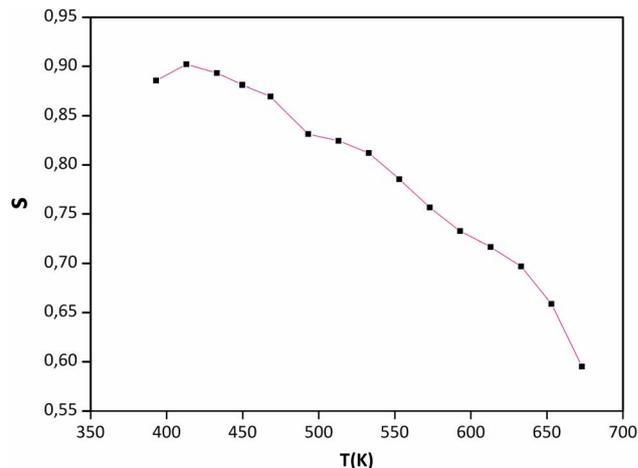
Fig. 9 Temperature dependence of " $s$ " for  $\text{Sr}_2(\text{Sn}_{0.33}\text{Sb}_{0.33}\text{In}_{0.33})_2\text{O}_6$ .
