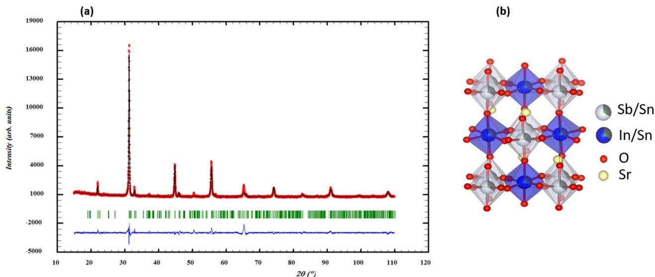
Fig. 1 (a) Rietveld refinement of XRD pattern of  $\text{Sr}_2(\text{Sn}_{0.33}\text{Sb}_{0.33}\text{In}_{0.33})_2\text{O}_6$  double perovskite (the black line corresponds to the experimental value, the red solid line is the fitted value, and the blue solid line is the difference between the experimental value and the fitted value). (b) The crystal structure of  $\text{Sr}_2(\text{Sn}_{0.33}\text{Sb}_{0.33}\text{In}_{0.33})_2\text{O}_6$  double perovskite.
