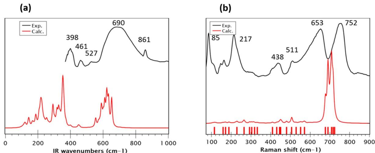
Fig. 3 Comparison between experimental and theoretical (a) infrared and (b) Raman spectra of  $\text{Sr}_2(\text{Sn}_{0.33}\text{Sb}_{0.33}\text{In}_{0.33})_2\text{O}_6$ . The precise positions of the calculated frequencies are depicted as sticks for clarity and precision.
