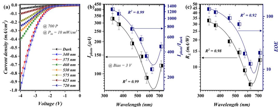
Fig. 4 Opto-electrical features of the fabricated photodetector at 700 pulses as a function of wavelength; (a)  $I$ - $V$  profile, (b)  $I_{\text{photo}}$  and  $I_{\text{photo}}/I_{\text{dark}}$  ratio, and (c)  $R_{\lambda}$  and EQE.
