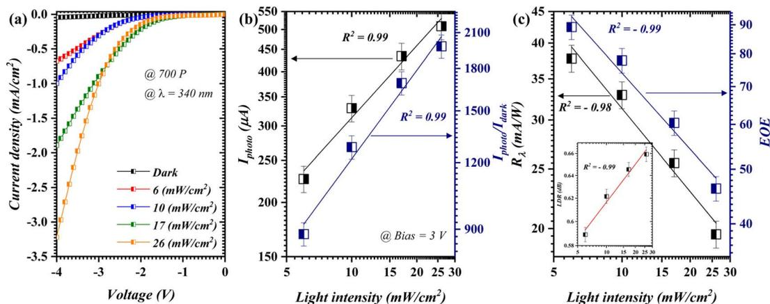
Fig. 5 Opto-electrical features of the fabricated photodetector at 700 pulses as a function of incident power; (a)  $I$ - $V$  profile, (b)  $I_{\text{photo}}$  and  $I_{\text{photo}}/I_{\text{dark}}$  ratio, and (c)  $R_{\lambda}$  and EQE.
