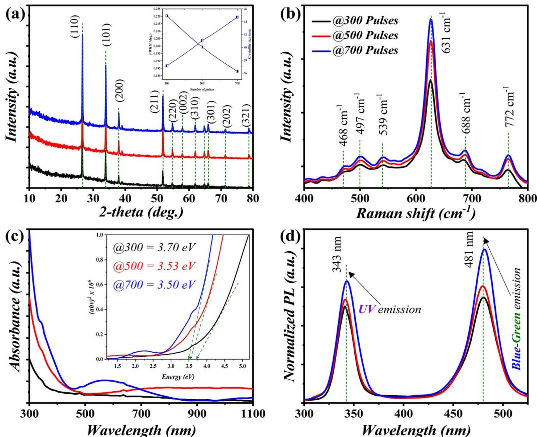
Fig. 1 (a) XRD patterns, (b) Raman spectra, (c) absorption spectra, and (d) PL spectra of the fabricated SnO<sub>2</sub> as a function of the number of pulses.
