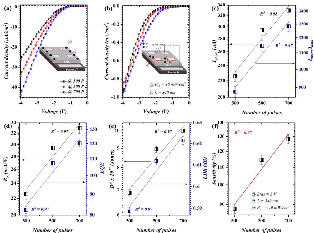
Fig. 3 Opto-electrical features of devices by means of laser pulses: (a) dark  $I$ - $V$ , (b) illuminated  $I$ - $V$ , (c)  $I_{\text{photo}}$  and  $I_{\text{photo}}/I_{\text{dark}}$  ratio, (d)  $R_{\lambda}$  and EQE, (e)  $D^*$  and LDR, and (f)  $S$  %; figure of merits were attained at 3 V, 340 nm, and  $10 \text{ mW cm}^{-2}$ .
