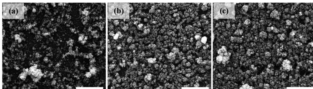
Fig. 2 FE-SEM features of the deposited SnO<sub>2</sub> layer/s using (a) 300, (b) 500, and (c) 700 laser pulses (scale bar = 1 μm).
