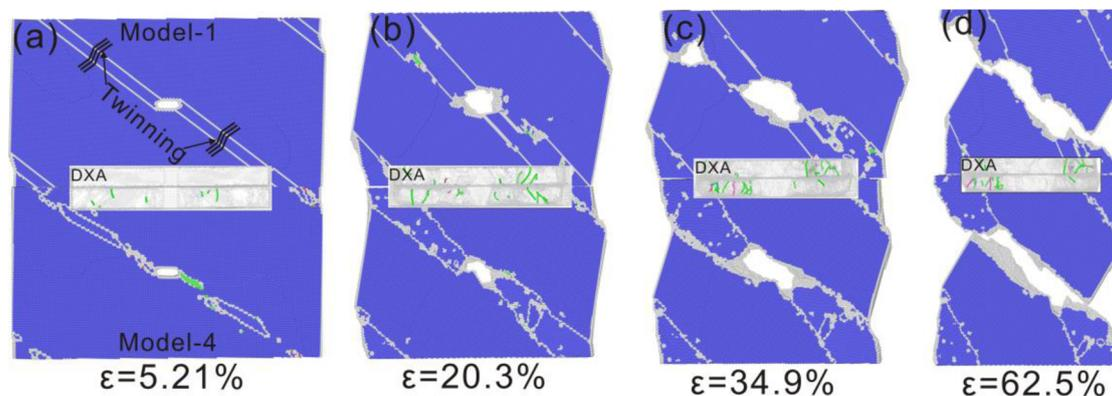
Fig. 11 Crack propagation in Model-14. The color of the atom is due to CNA, where blue is BCC, green is FCC, and white is an unknown structure, with dislocation analysis in the middle.
