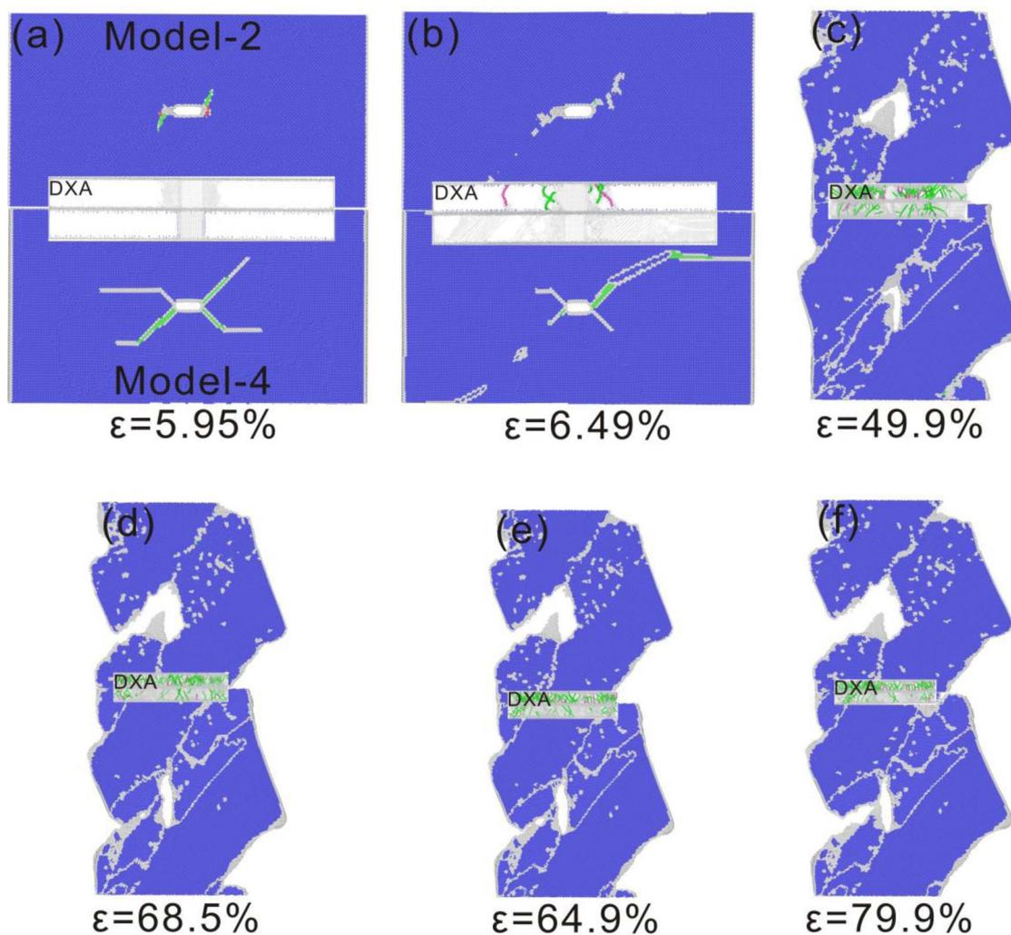
Fig. 13 Crack propagation in Model-24. The color of the atom is due to CNA, where blue is BCC, green is FCC, and white is an unknown structure, with dislocation analysis in the middle.
