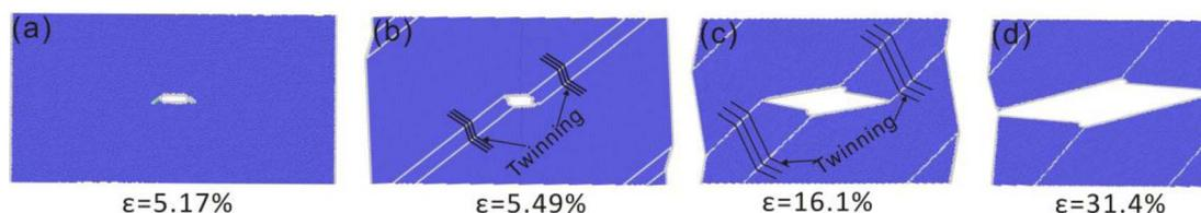
Fig. 4 Crack propagation process of Model-1. The color of the atoms is made up of CNA, where blue is the BCC atom, green is the FCC atom, and white is the atom of unknown structure.
