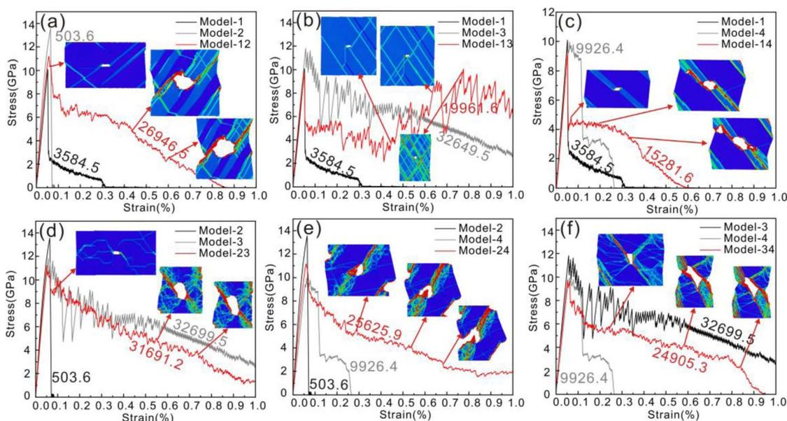
Fig. 8 Stress-strain curve of the combined model.
