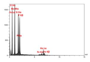
Fig. 4 EDX analysis of Ho<sub>3</sub>Fe<sub>5</sub>O<sub>12</sub>@FPS MNPs
