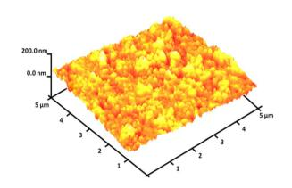
Fig. 6 Three-dimensional AFM images of Ho<sub>3</sub>Fe<sub>5</sub>O<sub>12</sub>@FPS MNPs.
