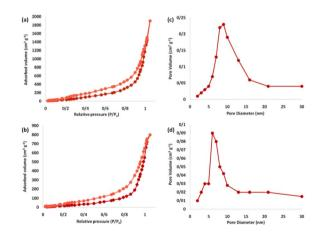
Fig. 7 Adsorption–desorption isotherms of (a) FPS and (b)  ${\rm Ho_3Fe_5-O_{12}@FPS}$  MNPs, and BJH pore size distributions of (c) FPS and (d)  ${\rm Ho_3Fe_5O_{12}@FPS}$  MNPs.
