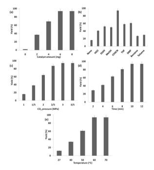
Fig. 9 Synthesis of the polymer using  ${\rm Ho_3Fe_5O_{12}@FPS}$  NPs with various (a) catalyst amounts, (b) solvents, (c) pressures of carbon dioxide, (d) times, and (e) temperatures.
