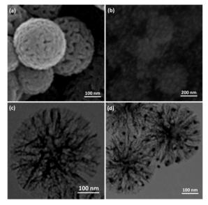
Fig. 1 FESEM illustrations of (a) FPS and (b) Ho<sub>3</sub>Fe<sub>5</sub>O<sub>12</sub>@FPS; (c) TEM illustrations of FPS and (d) Ho<sub>3</sub>Fe<sub>5</sub>O<sub>12</sub>@FPS.
