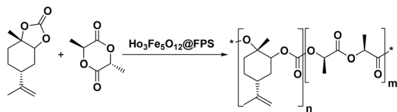
Scheme 2 \text{Ho}_3\text{Fe}_5\text{O}_{12} @FPS-catalyzed synthesis of the polymer.
