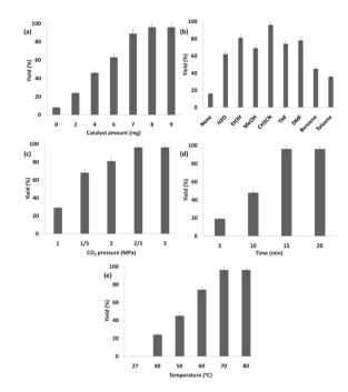
Fig. 8 Effects of catalyst amount (a), solvents (b), the pressure of carbon dioxide (c), time (d) and temperature (e) on the catalyzed cyclic carbonate synthesis.
