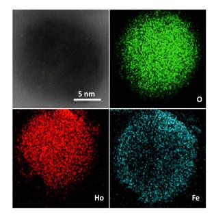
Fig. 2 TEM mapping of Ho<sub>3</sub>Fe<sub>5</sub>O<sub>12</sub> covering the overall state, Fe, O, and Ho.
