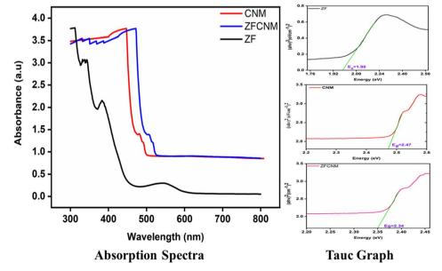
Fig. 5 The UV-visible DRS spectra and Tauc graphs of synthesized (a) ZF, (b) CNM, and (c) ZFCNM.
