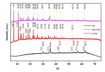
Fig. 3 XRD spectra of ZF, CNM, and ZFCNM.
