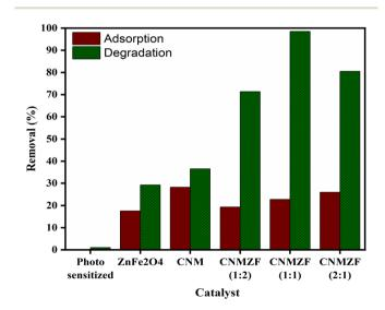
Fig. 1 Adsorption and photocatalytic removal of CR dye (10 mg  $L^{-1}$ ) with different CNMZF compositions compared to bare photocatalysts, conducted under dark and visible light (50 W) conditions for 75 minutes.
