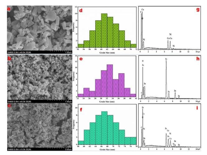
FESEM images (a-c), histograms for grain size (d-f), and EDX (g-i) of synthesized samples (i) CNM, (ii) ZF, and (iii) ZFCNM.
