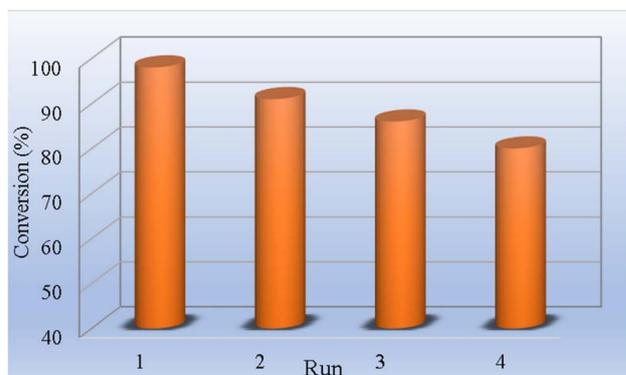
Fig. 8 Recycling data for MnSalop-GO·NH<sub>2</sub> as catalyst in the epoxidation of cyclooctene with H<sub>2</sub>O<sub>2</sub> : NaHCO<sub>3</sub>.
