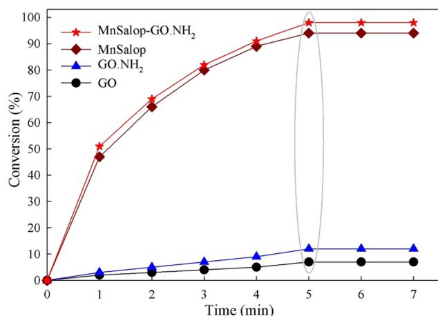
Fig. 7 Conversion–time curves for epoxidation of cyclooctene with GO, GO·NH<sub>2</sub>, MnSalop and MnSalop-GO·NH<sub>2</sub>. Reaction condition: the molar ratios for catalyst : olefin : H<sub>2</sub>O<sub>2</sub> : NaHCO<sub>3</sub> are (2 : 27 : 270 : 27); GO and GO·NH<sub>2</sub> (100 mg); EtOH (4 mL).
