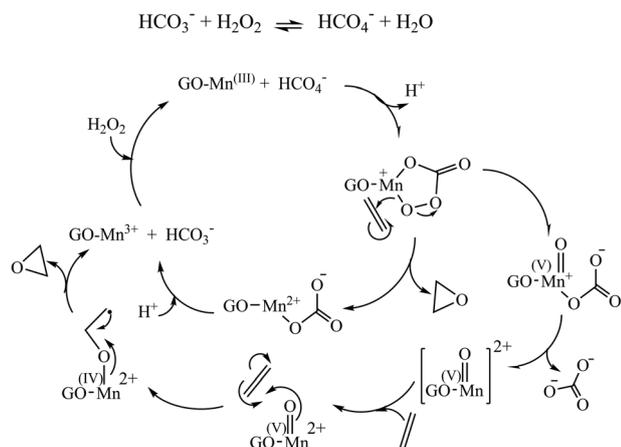
Scheme 3 Proposed mechanism for the epoxidation of alkene with H<sub>2</sub>O<sub>2</sub>/NaHCO<sub>3</sub> by MnSalop-GO·NH<sub>2</sub>.
