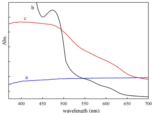
Fig. 1 DR UV-Vis spectra of: (a) GO, (b) MnSalop and (c) MnSalop-GO·NH<sub>2</sub>.
