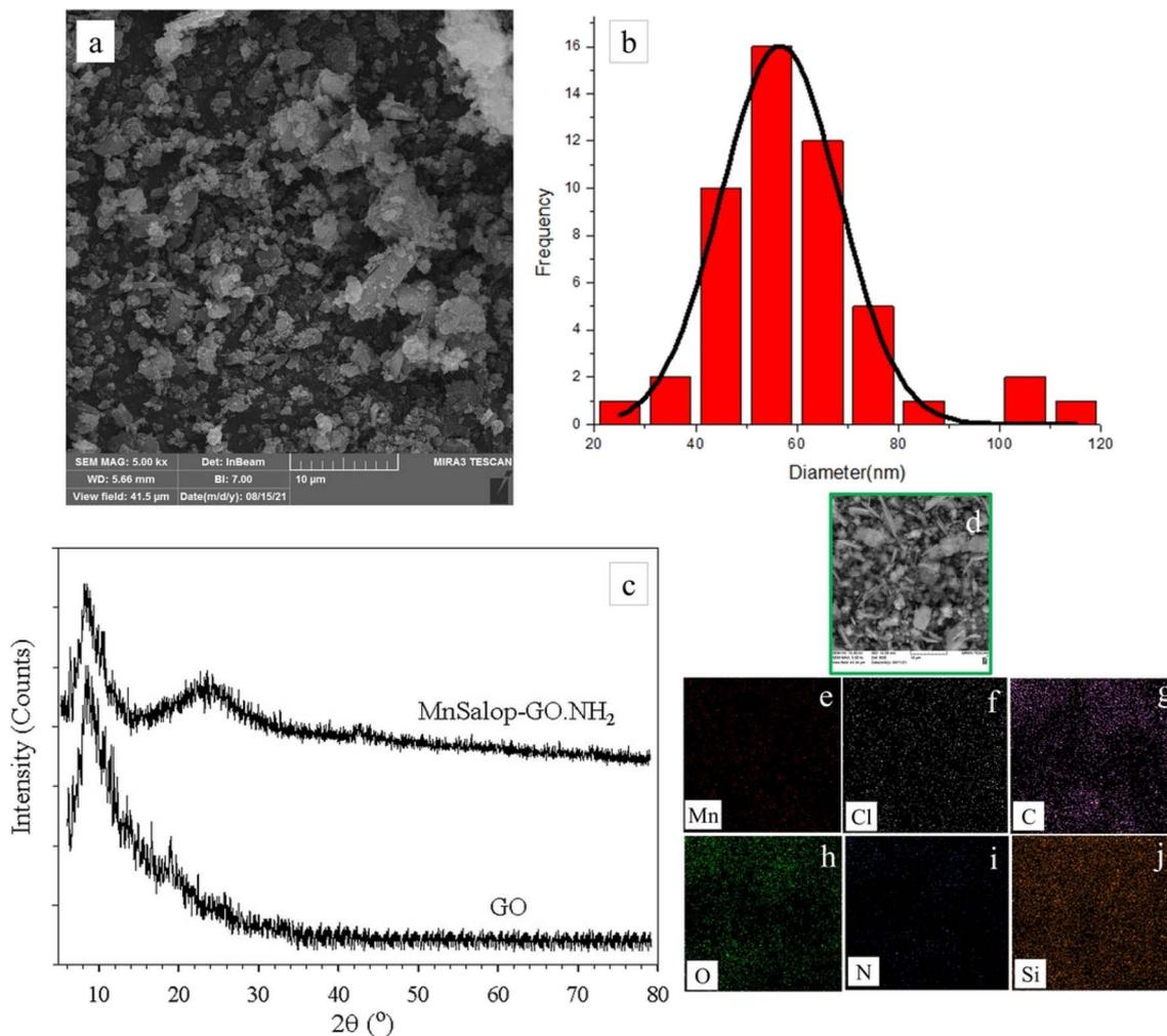
Fig. 3 (a) FE-SEM image of MnSalop-GO·NH<sub>2</sub>, (b) histogram of the particle size of MnSalop-GO·NH<sub>2</sub>, (c) XRD patterns of GO and MnSalop-GO·NH<sub>2</sub> and (d–j) elemental mapping image of the sample separated once.
