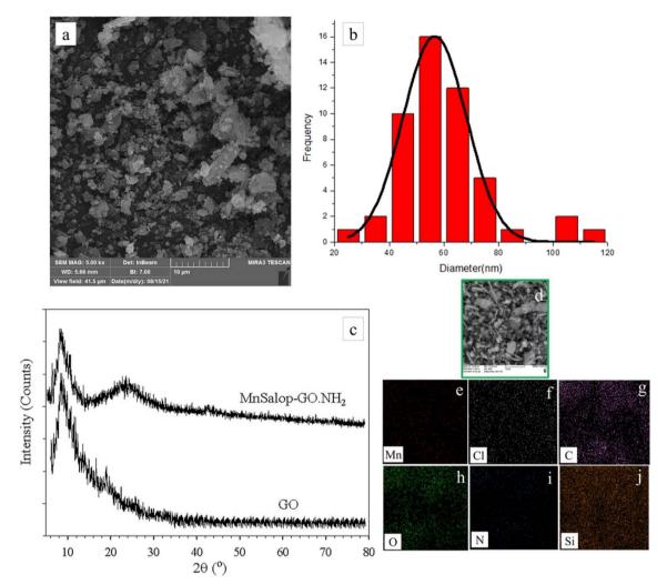
Fig. 3 (a) FE-SEM image of MnSalop-GO·NH<sub>2</sub>, (b) histogram of the particle size of MnSalop-GO·NH<sub>2</sub>, (c) XRD patterns of GO and MnSalop-GO·NH<sub>2</sub> and (d-j) elemental mapping image of the sample separated once.
