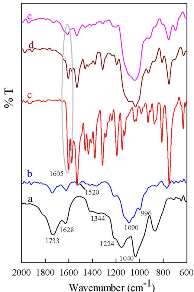
Fig. 2 FT-IR spectra of (a) GO, (b) GO·NH<sub>2</sub>, (c) MnSalop, (d) MnSalop-GO·NH<sub>2</sub> and (e) recovered MnSalop-GO·NH<sub>2</sub>.
