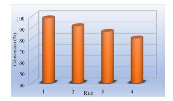
Fig. 8 Recycling data for MnSalop-GO·NH $_2$  as catalyst in the epoxidation of cyclooctene with  $H_2O_2$ : NaHCO $_3$ .
