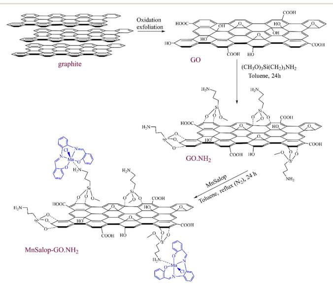
Scheme 2 Schematic illustration for the preparation of MnSalop-GO·NH<sub>2</sub>
