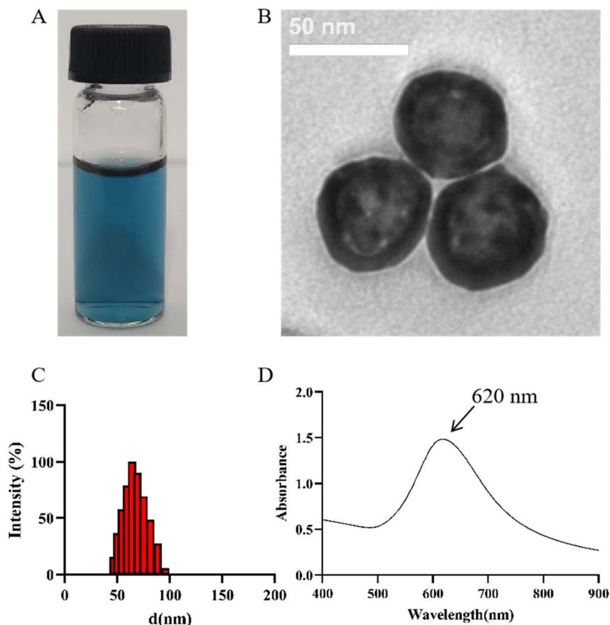
Fig. 2 Characterization of PVP@HG NPs. Appearance (A) and TEM image (B) of PVP@HG NPs. (Scale bar = 50 nm); (C) the diameter of PVP@HG NPs; (D) the absorbance spectra of PVP@HG NPs.
