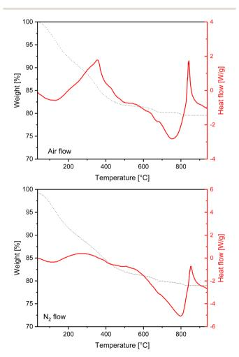
Fig. 7 TGA (black dotted line) and DSC (red continuous line) curves of P11b measured under air flow (top) and under nitrogen flow (bottom).
