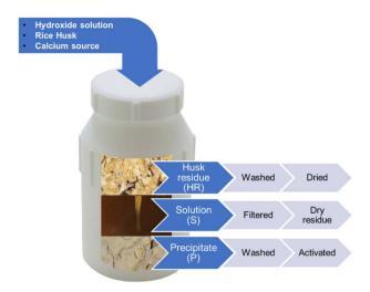
Fig. 1 A schematic representation of the chemical process for the valorisation of rice husk based biomass
