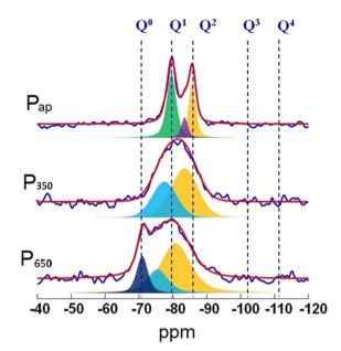
Fig. 12  $^{29}$ Si MAS NMR spectra of P11b as prepared ( $P_{ap}$ ), after thermal treatment at 350 °C (P<sub>350</sub>), and after thermal treatment at 650 °C (P<sub>650</sub>).
