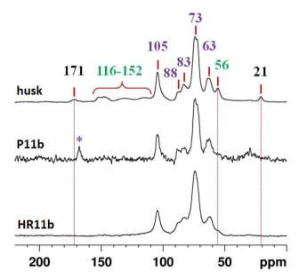
Fig. 10 <sup>13</sup>C CPMAS NMR spectra of rice husk, P11b and HR11b.
