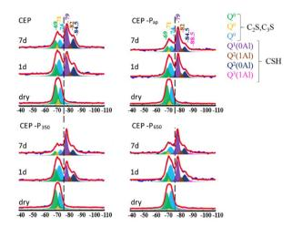
Fig. 15 <sup>29</sup>Si SS-NMR spectra measured on the paste samples before hydration, after 1 day and after 7 days.
