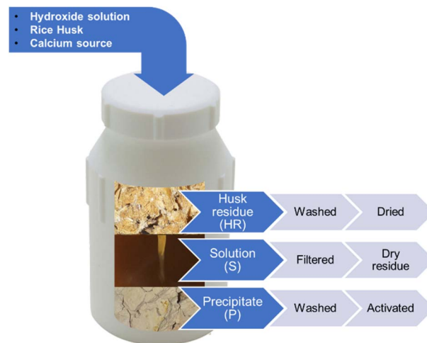
Fig. 1 A schematic representation of the chemical process for the valorisation of rice husk based biomass.
