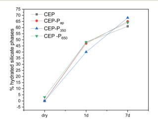
Fig. 16 Plot of the % of silicate hydrated phases (C–S–H) on the total silicate phases vs. hydration time, from  $^{29}$ Si SS-NMR data.
