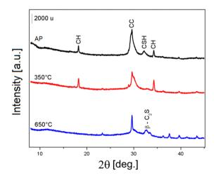
Fig. 11 PXRD pattern of P11b as prepared ( $P_{ap}$  – black), after thermal treatment at 350 °C ( $P_{350}$  – red), and after thermal treatment at 650 °C ( $P_{650}$  – blue).  $CH = Ca(OH)_2$  portlandite  $C\bar{C} = CaCO_3$  calcite;  $CSH = CaCO_3$ calcium silicate hydrate;  $\beta$ -C<sub>2</sub>S = anhydrous  $\beta$ -dicalcium silicate.
