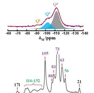
Fig. 3  $^{29}$ Si MAS (top) and  $^{13}$ C CPMAS (bottom) NMR spectra of raw rice husk. In violet, the signals of cellulose, in black those of hemicellulose, and in green those of lignin.
