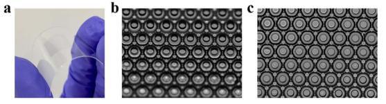
Fig. 6 Oil films patterned on curved and flexible substrates are subjected to repeated bent tests to showcase their flexibility and durability. (a) Photograph of a transparent and flexible device with patterned oil films on its surface. (b) Image showing the oil films while being bent with a curvature of 0.14 mm<sup>-1</sup>. (c) Image showing the oil films in a flat state after undergoing 100 cycles of repeated bending tests with a curvature of 0.33 mm<sup>-1</sup>.
