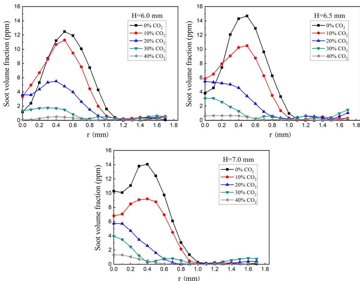
Fig. 3 Radial distributions of soot volume fraction at different flame heights (6.0, 6.5 and 7.0 mm) in flames with different CO<sub>2</sub> dilution rates at 10 atm (experimental results).
