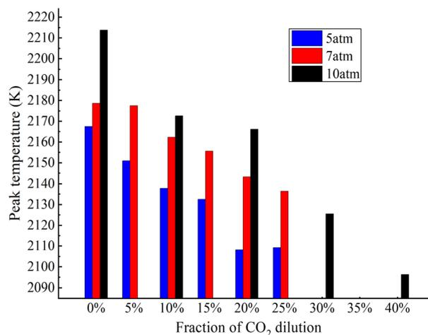
Fig. 9 Peak temperature of flames at 5, 7 and 10 atm with different dilution ratio of CO<sub>2</sub> (experimental results).
