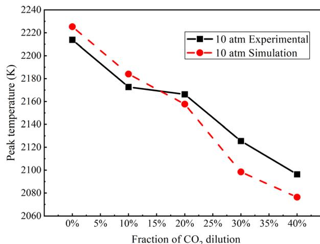
Fig. 8 Peak flame temperature at 10 atm with different dilution ratios of CO<sub>2</sub> (experimental and simulation results).
