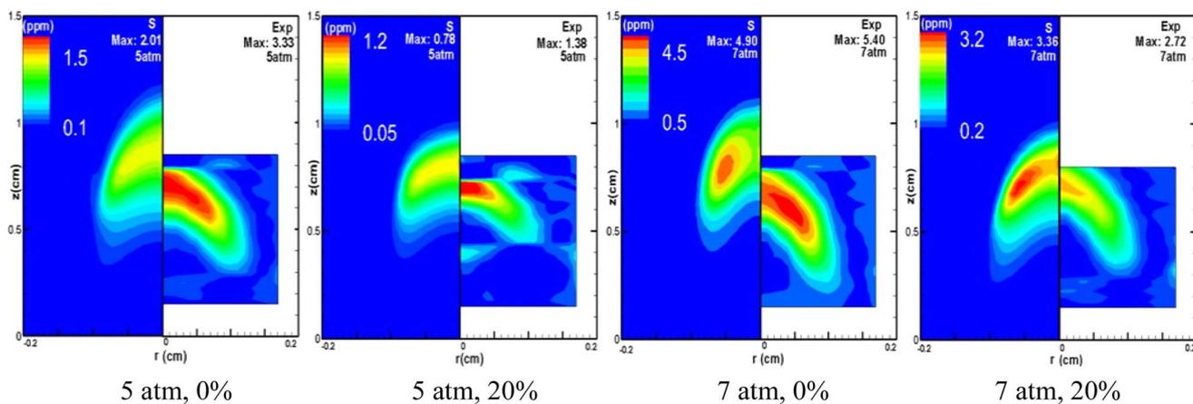
Fig. 7 The distribution of soot volume fraction in CH<sub>4</sub> flames at CO<sub>2</sub> dilution ratios of 0% and 20% under pressures of 5 and 7 atm (with the left side labeled "S" for simulation results, and the right side labeled "Exp" for experimental results).
