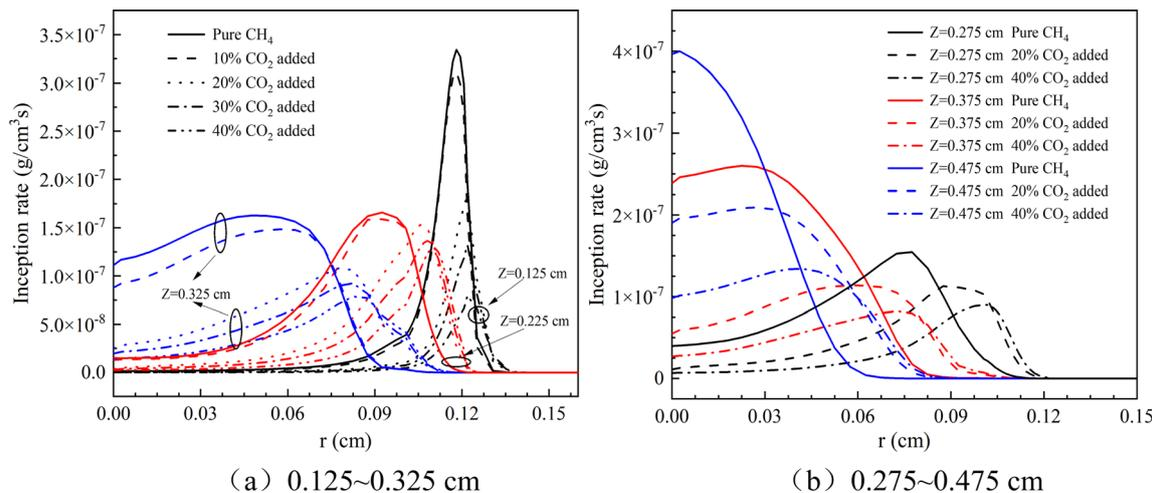
Fig. 12 Soot nucleation inception rate at different flame heights with different dilution ratios of CO<sub>2</sub> at 10 atm. Soot nucleation inception rates at varying flame heights (a) 0.125 to 0.325 cm and (b) 0.275 to 0.475 cm with different CO<sub>2</sub> dilution ratios at 10 atm.
