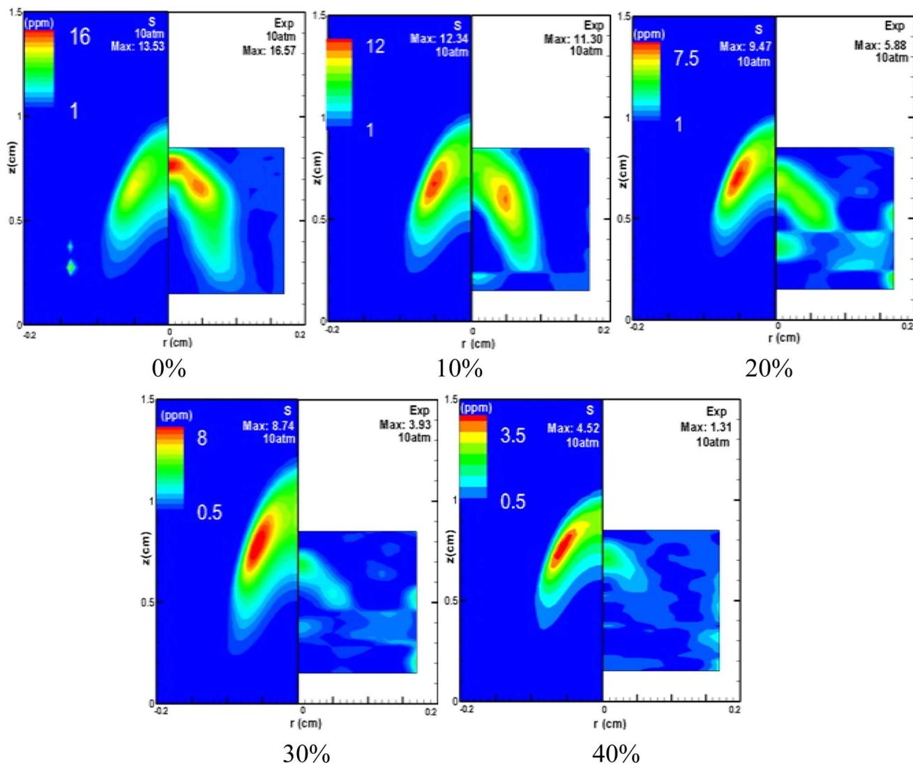
Fig. 6 The distribution of soot volume fraction in a CH<sub>4</sub> flame with CO<sub>2</sub> dilution ratios ranging from 0% to 40% at 10 atm (with the left side labeled "S" representing simulation results, and the right side labeled "Exp" representing experimental results).
