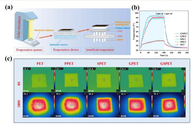
Fig. 4 Experimental setup for solar-powered interfacial evaporation. (b) The temperature rise and fall of dry PET, PPET, GPET, SPET and GSPET samples under one sun solar illumination. (c) Infrared images of PET, PPET, GPET, SPET and GSPET surfaces at the initial sate and equilibrium state after 180 s irradiation.
