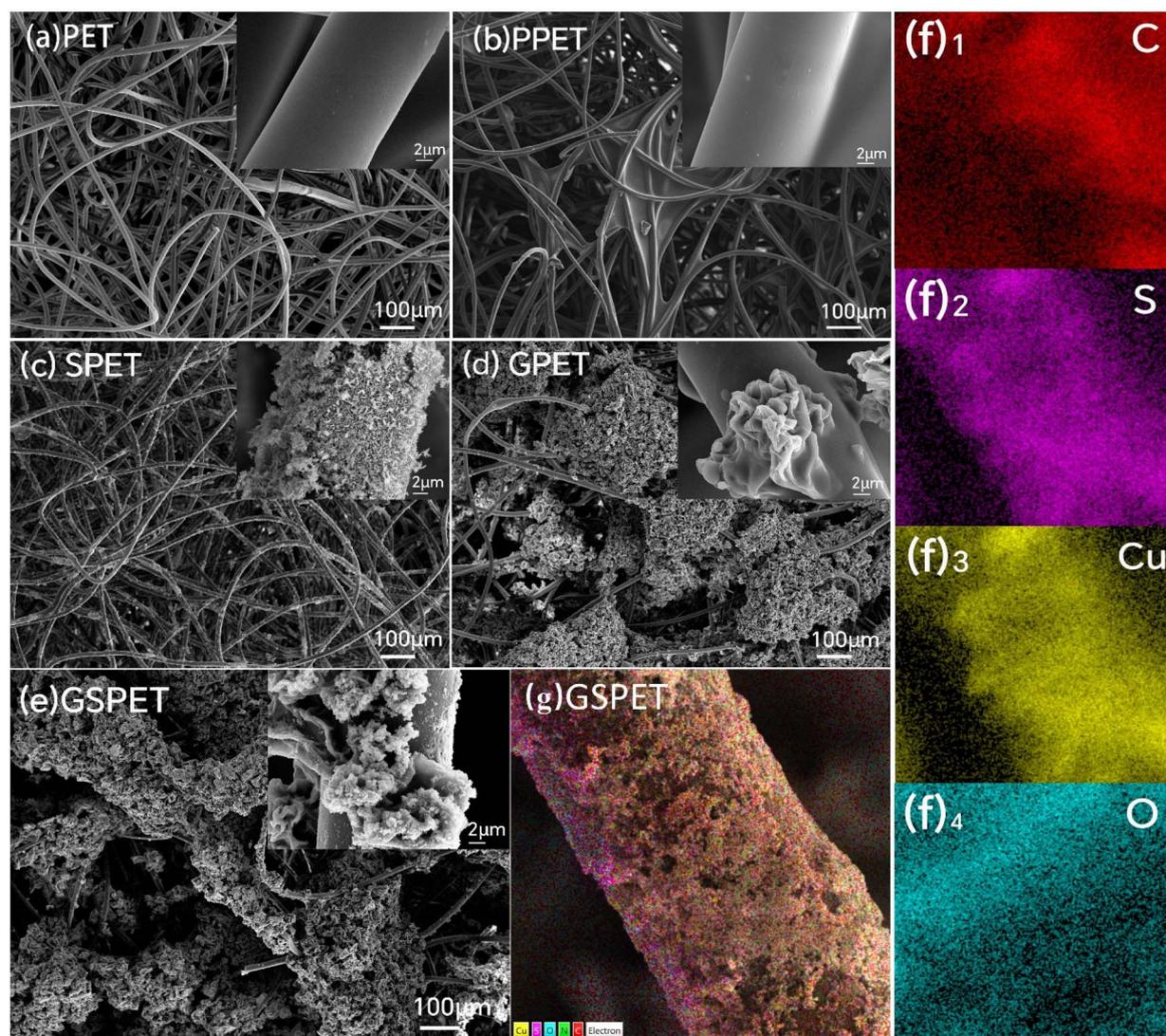
Fig. 2 SEM images of (a) PET, (b) PPET (PVA@PET), (c) SPET ( $\text{Cu}_x\text{S}$ @PET), (d) GPET (GO@PET), and (e) GSPET ( $\text{Cu}_x\text{S}/\text{GO}$ @ES) surfaces at different magnifications. Elemental distributions (f1)–(f4) and elemental content analysis plots (g) of GSPET.
