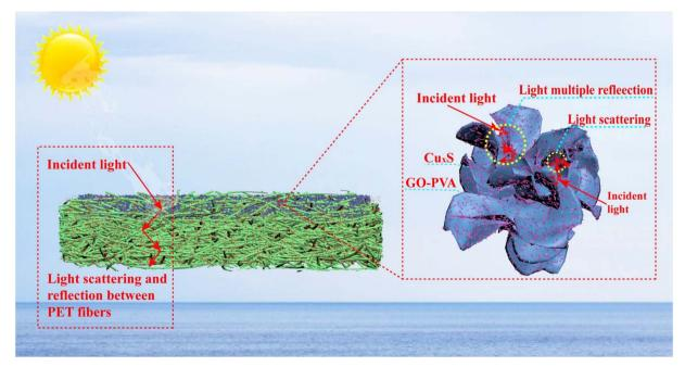
Fig. 6 Schematic of solar steam generation mechanism for the solar evaporator based on the GSPET.
