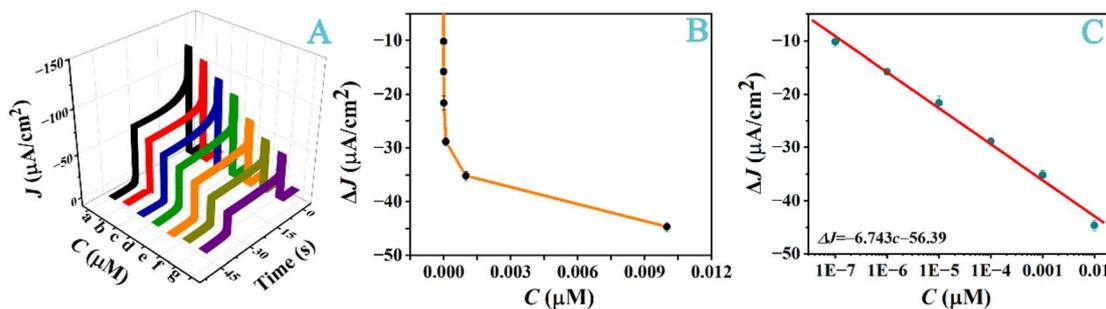
Fig. 5 (A) Photocurrent responses of the PEC sensor to different concentrations of TROJAN (a: blank and baseline current and b to g: 10 nM to 0.1 pM and their corresponding currents). (B)  $\Delta J$  plotted against concentration. (C)  $\Delta J$  plotted as a function of  $\log C$ . The error bars are relative standard deviations (RSDs) of three replicates.
