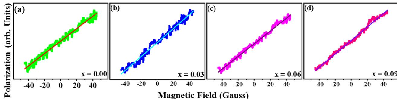
Fig. 7 Magnetoelectric coupling/variation of electric polarization w.r.t. applied magnetic field with NFO contents (a)  $x = 0.00$ , (b)  $x = 0.03$ , (c)  $x = 0.06$  and (d)  $x = 0.09$  in  $(1 - x)[0.7\text{BFO} + 0.3\text{MMO}] + x\text{NFO}$  triphasic composites.
