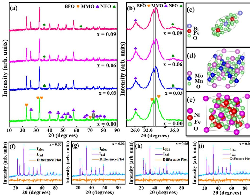
Fig. 2 (a) XRD patterns of  $(1-x)[0.7\text{BFO} + 0.3\text{MMO}] + x\text{NFO}$  with  $x = 0.00, 0.03, 0.06,$  and  $0.09$  phase-fractions, (b) BFO twin peaks, crystal structures of (c) BFO, (d) MMO, and (e) NFO, Rietveld refinement patterns for (f)  $x = 0.0$ , (g)  $x = 0.03$ , (h)  $x = 0.06$ , and (i)  $x = 0.09$  composites.
