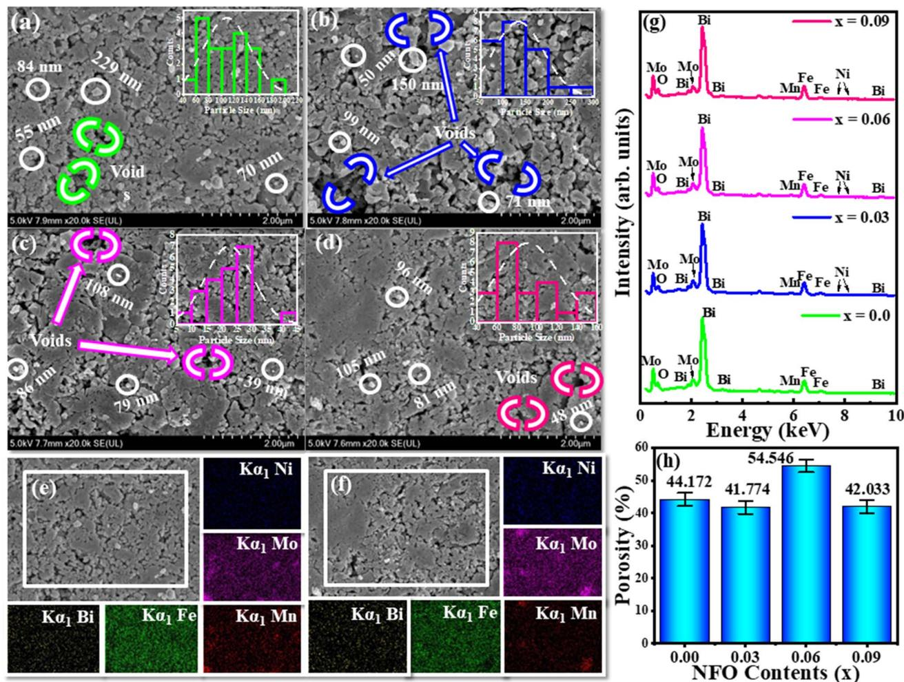
Fig. 3 FESEM images of  $(1-x)[0.7\text{BFO} + 0.3\text{MMO}] + x\text{NFO}$  triphasic composites for  $x =$  (a) 0.00, (b) 0.03, (c) 0.06 and (d) 0.09, X-ray mapping for  $x =$  (e) 0.00 and (f) 0.09, (g) EDX pattern and (h) percentage porosities for all concentrations.
