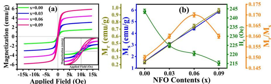
Fig. 5 (a) MH loops of  $(1-x)[0.7\text{BFO} + 0.3\text{MMO}] + x\text{NFO}$  triphasic composites for  $x = 0.00, 0.03, 0.06$  and  $0.09$ , (b) saturation magnetization ( $M_s$ ), remanence magnetization ( $M_r$ ), squareness ratio ( $M_r/M_s$ ) and coercive field ( $H_c$ ) w.r.t. substitution contents ( $x$ ).
