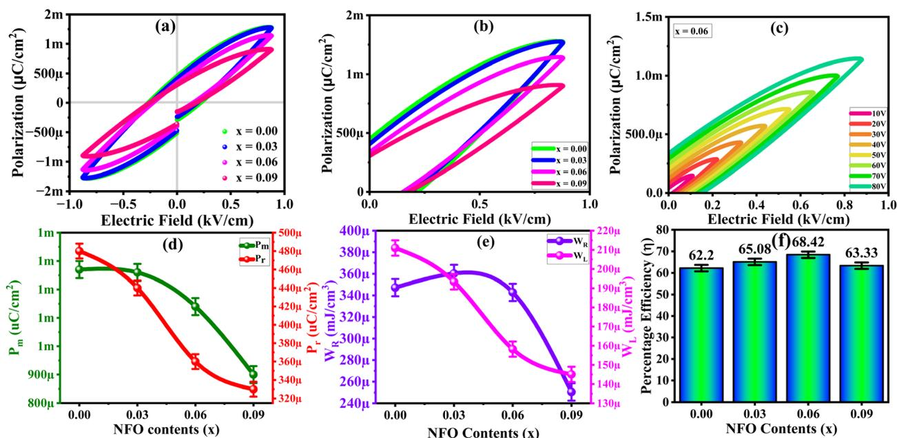
Fig. 6 (a) Polarization ( $P$ ) vs. electric field ( $E$ ), (b) estimation of energy density by charge–discharge region, (c) charge–discharge observation at various strengths of electric field, (d) saturation/maximum polarization ( $P_m$ ) and remanence polarization ( $P_r$ ) for different NFO contents ( $x$ ), (e) recoverable energy density ( $W_R$ ) and lost energy density ( $W_L$ ) for different concentrations of NFO, and (f) energy storage efficiency for various NFO contents ( $x$ ).
