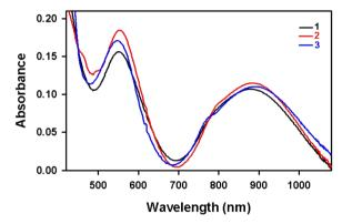
Fig. 1 UV-vis absorption spectra of complexes 1-3 (10  $\times$  10<sup>-3</sup> M) recorded in acetonitrile at room temperature.
