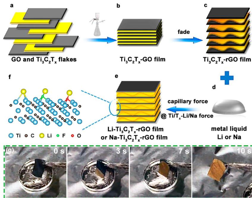
Fig. 6 (a–f) Schematic diagram of Li/Na– $\text{Ti}_3\text{C}_2\text{T}_x$ -rGO preparation; (g) wetting process of  $\text{Ti}_3\text{C}_2\text{T}_x$ -rGO.<sup>65</sup> Copyright 2019, American Chemical Society.
