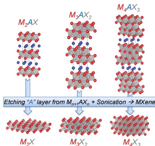
Fig. 1 Structures of MAX phases and their derived pristine MXene monosheets. M is a transition metal, *e.g.*, Ti; A is an element from group 13 or 14, *e.g.*, Al. X is C, N, or their combination.<sup>24</sup> Copyright 2013, Wiley-VCH.
