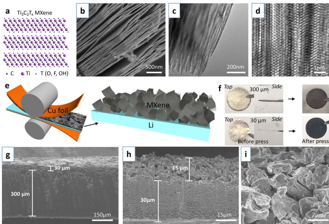
Fig. 5 (a-d) Atomic structure, SEM, TEM, and high-resolution images of  $\text{Ti}_3\text{C}_2\text{T}_x$  MXene; (e) fabrication process of MXene-Li electrode; (f) digital photographs of lithium sheets; (g-i) SEM images of MXene-Li electrode.<sup>63</sup> Copyright 2020, American Chemical Society.
