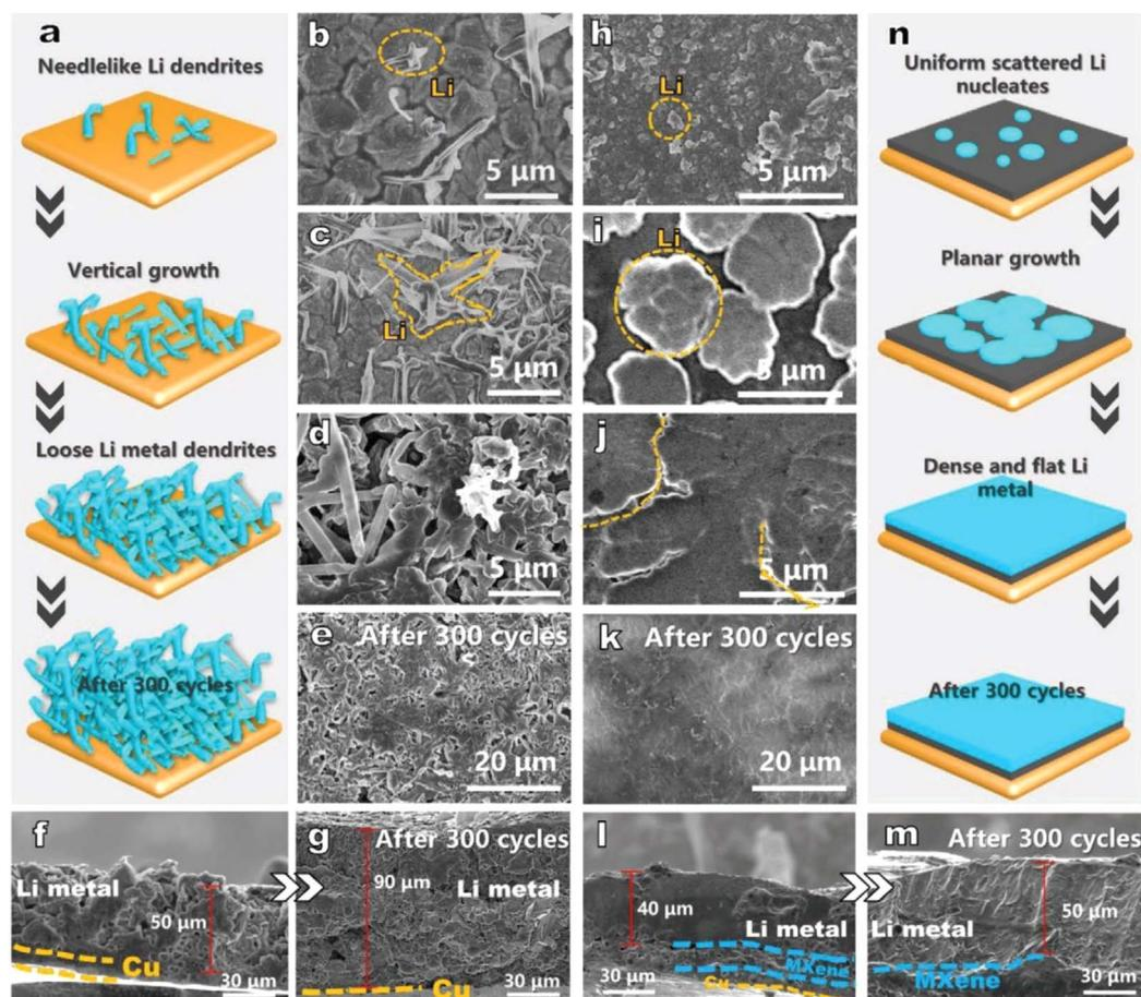
Fig. 3 Schematic representation of lithium deposition on (a) copper foil and (n) Ti<sub>3</sub>C<sub>2</sub>T<sub>x</sub> substrate; morphological evolution of (b–g) copper foil and (h–m) Ti<sub>3</sub>C<sub>2</sub>T<sub>x</sub>. Reproduced with permission from ref. 61. Copyright 2021, Wiley-VCH.
