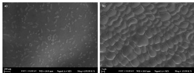
Fig. 2 Surface images of the  $\text{BaF}_2$  compound obtained by SEM, scale bars: (a) 200 nm, (b) 1  $\mu\text{m}$ .
