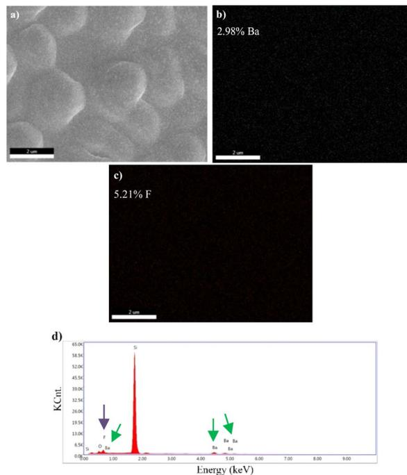
Fig. 6 SEM-EDS analysis results of 100 nm thick  $\text{BaF}_2$  compound. (a) SEM image of the surface topography, EDS mappings of (b) Ba, (c) F elements in  $\text{BaF}_2$  coating deposited on silicon substrate, (d) EDS spectrum of the area shown in (a) (scale bar is 2  $\mu\text{m}$ ). F element's and Ba element's EDS peaks are represented by purple and green arrows respectively.
