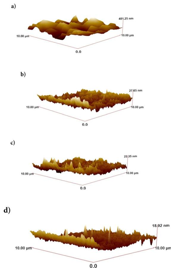
Fig. 1 AFM images of samples coated on quartz glasses in  $10 \times 10 \mu\text{m}^2$  scanning areas: (a)  $\text{BaF}_2$ , (b)  $\text{MgF}_2$ , (c)  $\text{Ba}_x\text{Mg}_{1-x}\text{F}_2$  ( $x > 0.5$ ) and (d)  $\text{Ba}_x\text{Mg}_{1-x}\text{F}_2$  ( $x < 0.5$ ).
