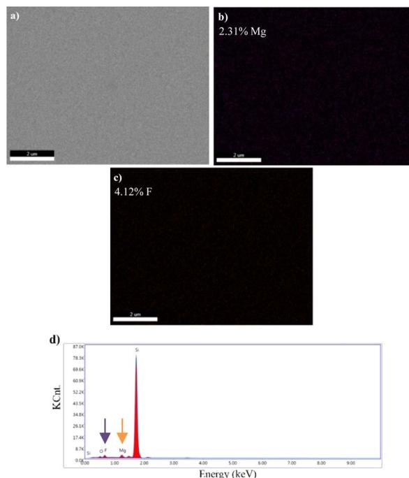
Fig. 7 SEM-EDS analysis results of 100 nm thick  $\text{MgF}_2$  compound. (a) SEM image of the surface topography, EDS mappings of (b) Mg, (c) F elements in  $\text{MgF}_2$  coating deposited on silicon substrate, (d) EDS spectrum of the area shown in (a) (scale bar is 2  $\mu\text{m}$ ). F element's and Mg element's EDS peaks are represented by purple and orange arrows respectively.
