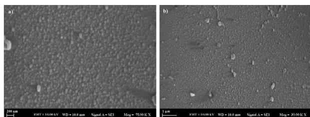
Fig. 4 Surface images of  $\text{Ba}_x\text{Mg}_{1-x}\text{F}_2$  (barium-rich,  $x > 0.5$ ) alloy obtained by SEM, scale bars: (a) 200 nm, (b) 1  $\mu\text{m}$ .
