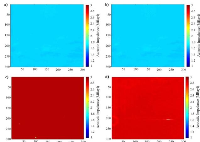
**Fig. 10** Two-dimensional acoustic impedance maps of (a)  $\text{BaF}_2$  compound, (b)  $\text{MgF}_2$  compound, (c)  $\text{Ba}_x\text{Mg}_{1-x}\text{F}_2$  alloy ( $x > 0.5$ ) and (d)  $\text{Ba}_x\text{Mg}_{1-x}\text{F}_2$  alloy ( $x < 0.5$ ), recorded by 80 MHz SAM. The scanning area is 4.8 mm  $\times$  4.8 mm with 300  $\times$  300 sampling points. The colour bar represents the variation in acoustic impedance values.
