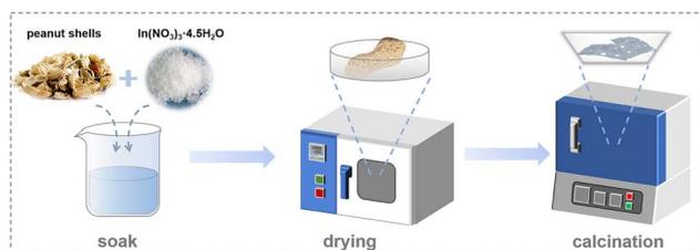
Fig. 1 Schematic diagram of the preparation process for the K-In<sub>2</sub>O<sub>3</sub> porous sheets.
