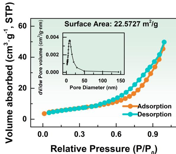
Fig. 5 N<sub>2</sub> isothermal adsorption/desorption isotherms (the inset shows the BJH pore size distribution plot).
