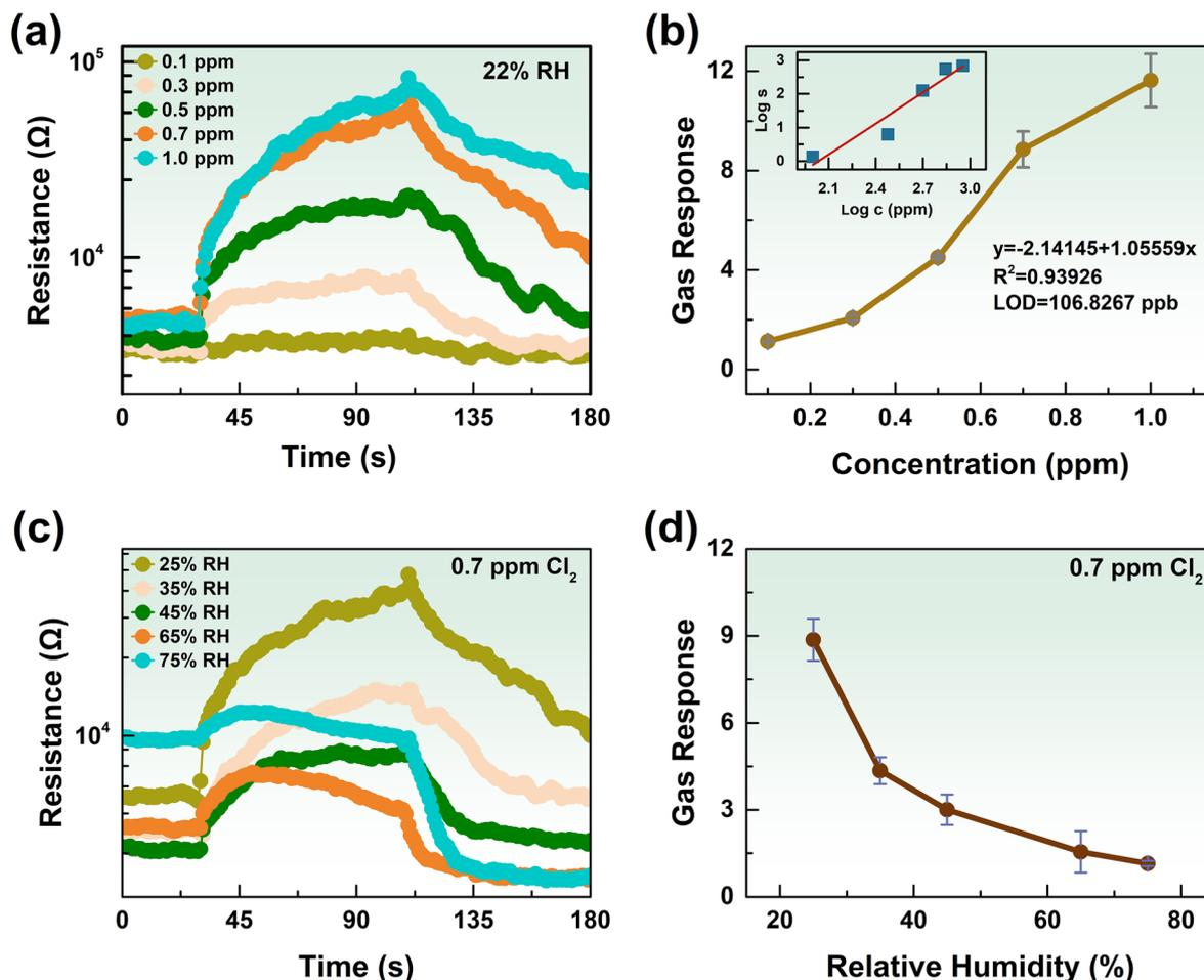
Fig. 7 (a) Dynamic resistance curves and (b) sensitivity to a series of concentrations of  $\text{Cl}_2$  at 240 °C (the inset of (b) is the double logarithmic curve); (c) dynamic resistance curves and (d) response value to 0.7 ppm  $\text{Cl}_2$  at different levels of humidity.
