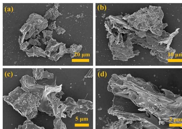
Fig. 3 SEM image of the K-In<sub>2</sub>O<sub>3</sub> porous sheets.
