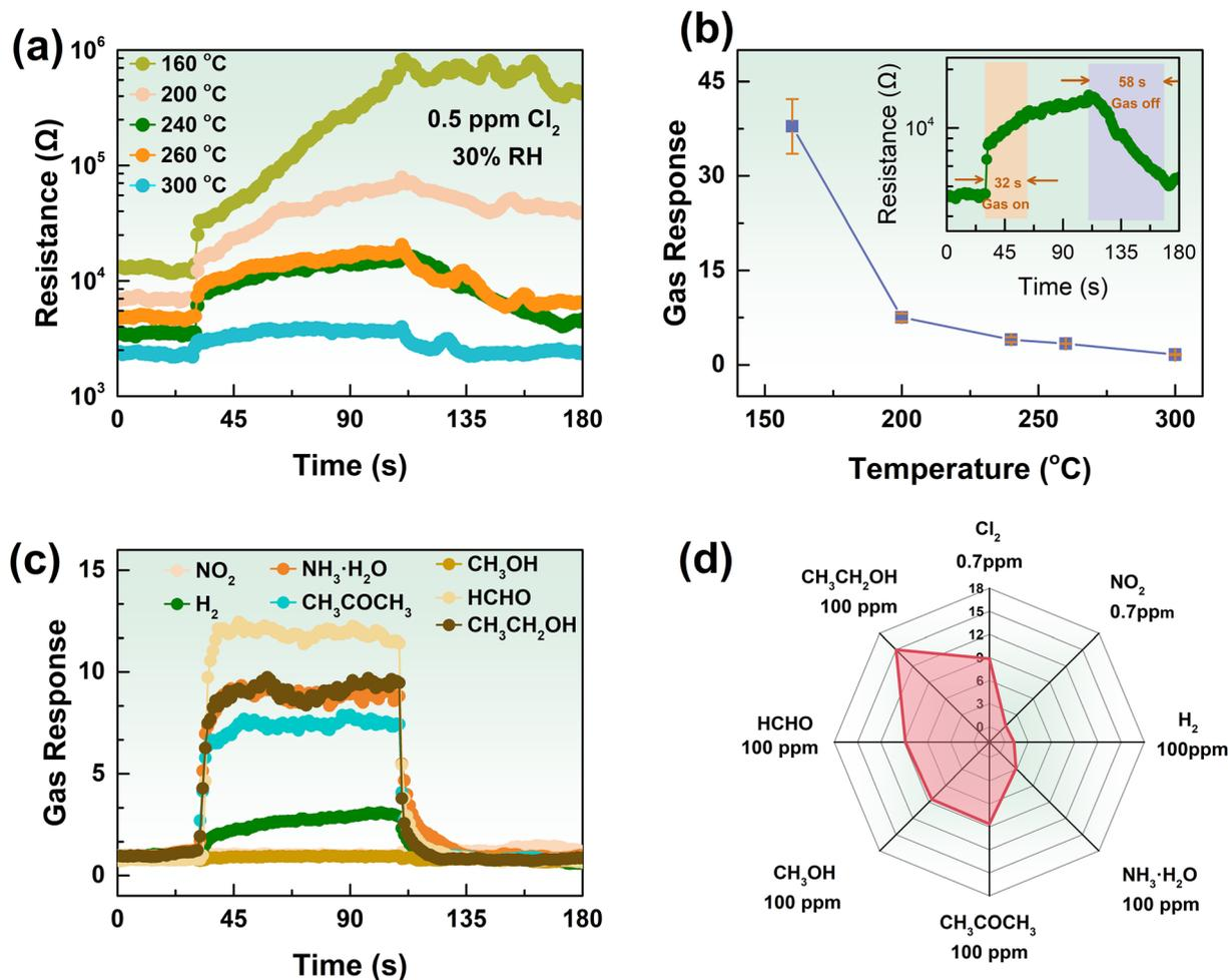
Fig. 6 (a) Dynamic resistance curves and (b) sensitivity to 0.5 ppm Cl<sub>2</sub> at various working temperatures (the inset of (b) is the response/recovery time curve); (c) dynamic response curves and (d) response values to various gases by the K-In<sub>2</sub>O<sub>3</sub> porous sheet sensor.
