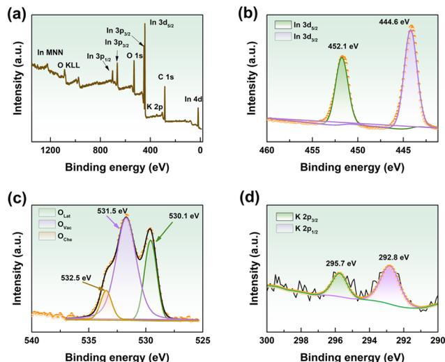
Fig. 4 XPS survey spectra of the K-In<sub>2</sub>O<sub>3</sub> porous sheets: (a) fully scanned spectra, (b) In 3d, (c) O 1s, and (d) K 2p.
