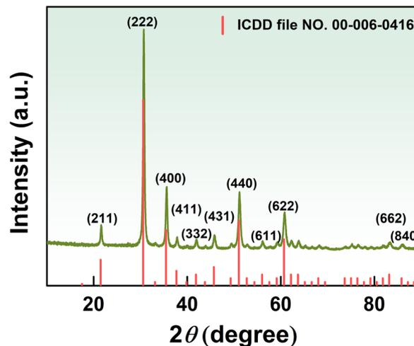
Fig. 2 XRD pattern of the K-In<sub>2</sub>O<sub>3</sub> porous sheets.
