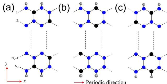
Fig. 2 The unit cells of three types of zigzag edge  $\text{SiP}_3$  NRs terminated with (a) PP-PP, (b) PSi-SiP and (c) PP-PSi edges. The edge atoms are passivated by hydrogen atoms (white color balls). The number of zigzag chains, *i.e.*,  $N_z$  determines the width of the NRs along the *y*-direction. The periodicity is considered along the *x*-direction.
