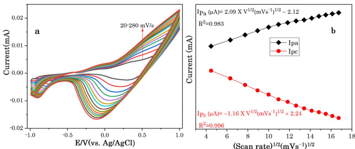
Fig. 6 (a) CVs of  $\text{Cu}_7\text{S}_4$  at different scan rates from 20 to 280  $\text{mV s}^{-1}$  in a 0.1 M NaOH solution in the presence of 60  $\mu\text{M}$  glucose, (b) the corresponding plots of anodic and cathodic peak currents.
