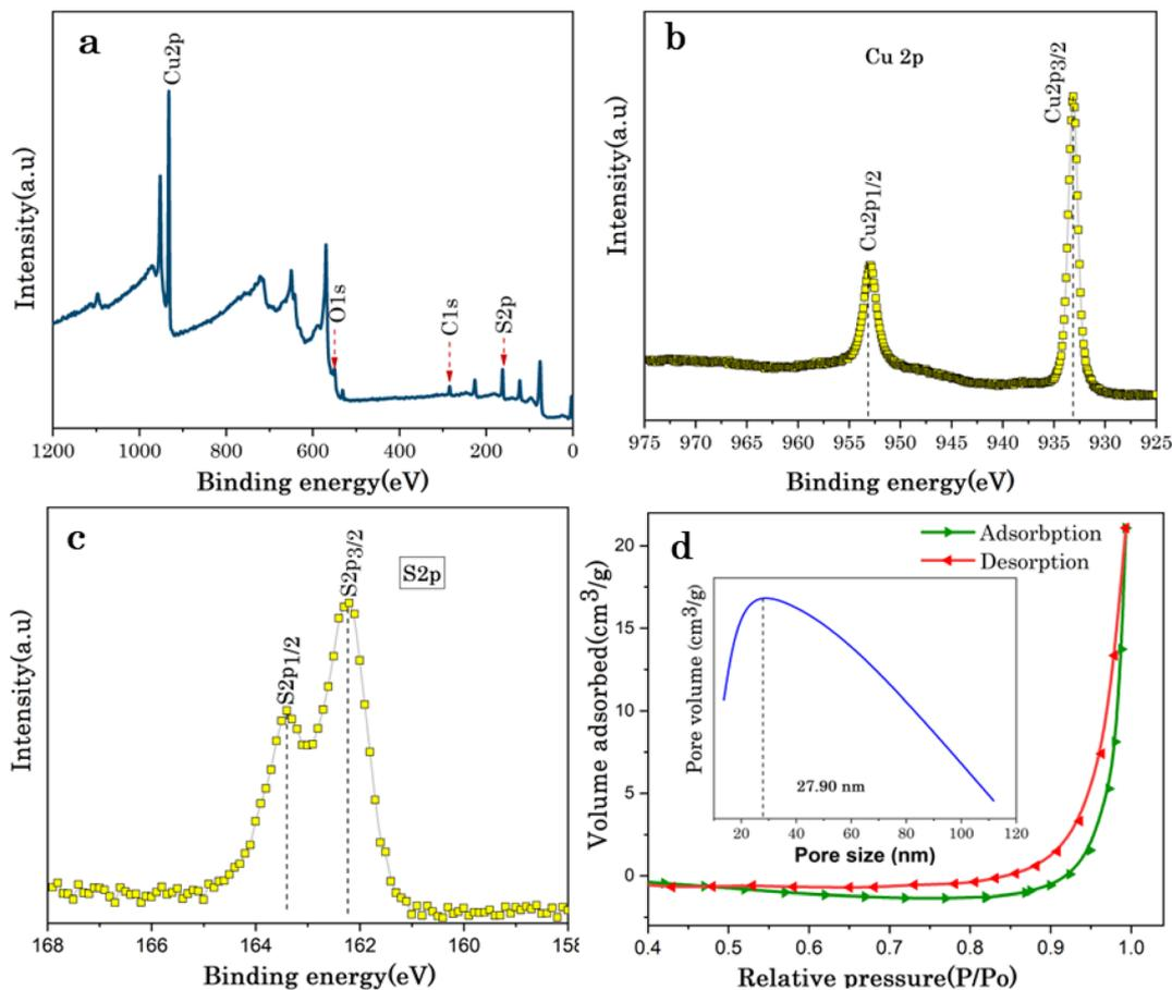
Fig. 3 (a) Wide scan XPS survey of  $\text{Cu}_7\text{S}_4$  hollow nanotubes; XPS spectrum (b) Cu 2p, (c) S 2p; (d) nitrogen ( $\text{N}_2$ ) adsorption/desorption isotherms (insert pore size distribution curve of  $\text{Cu}_7\text{S}_4$  hollow nanotubes).
