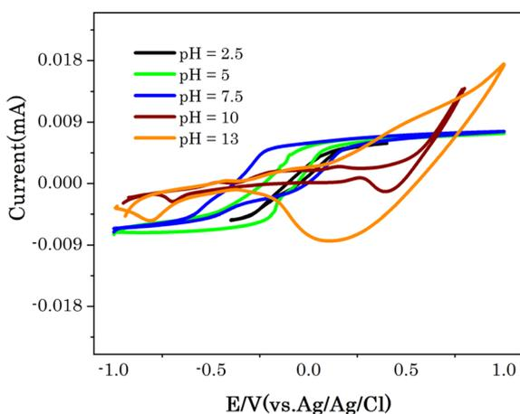
Fig. 4 CV curves of  $\text{Cu}_7\text{S}_4$  at different pH values in 0.1 M NaOH solution with 60  $\mu\text{M}$  glucose at scan rate of 50  $\text{mV s}^{-1}$ .
