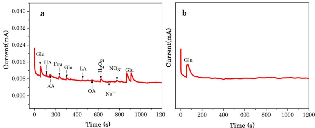
Fig. 8 (a) Chronoamperometric current response of  $\text{Cu}_7\text{S}_4$  hollow nanotubes to  $50 \mu\text{M}$  glucose and  $10 \mu\text{M}$  interferents  $0.1 \text{ M NaOH}$  (b) the chronoamperometric stability test conducted at  $\text{Cu}_7\text{S}_4$  hollow nanotubes electrode with the addition of  $50 \mu\text{M}$  glucose in  $0.1 \text{ M NaOH}$ .
