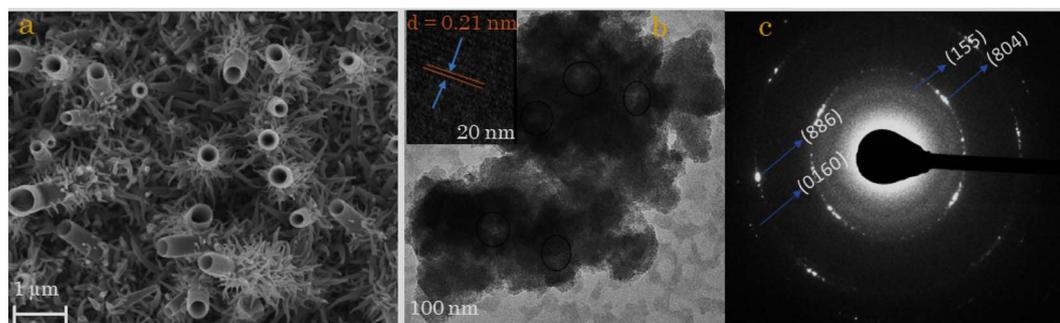
Fig. 1 (a) SEM image, (b) TEM image (inserted HRTEM), and (c) SAED of Cu<sub>7</sub>S<sub>4</sub> at 96 h.
