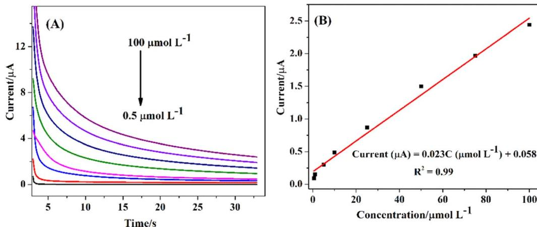
Fig. 7 (A) Chronoamperometry response to various glucose concentrations (0.5 to 100  $\mu\text{mol L}^{-1}$ ) and (B) the corresponding calibration curves for  $\text{Cu}_7\text{S}_4$  hollow nanotubes.
