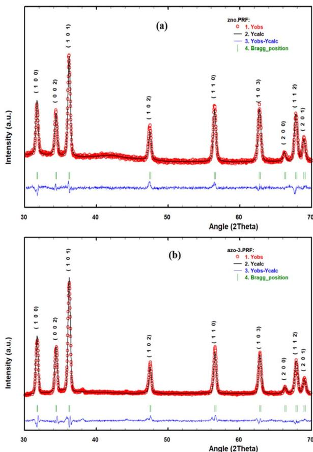
Fig. 2 Rietveld refinement of (a) Un-doped ZnO and (b) AZO-3.
