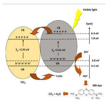
Fig. 9 Proposed mechanism for the degradation of MB dye by  ${\rm TiO_2}$ -CuSe composites.
