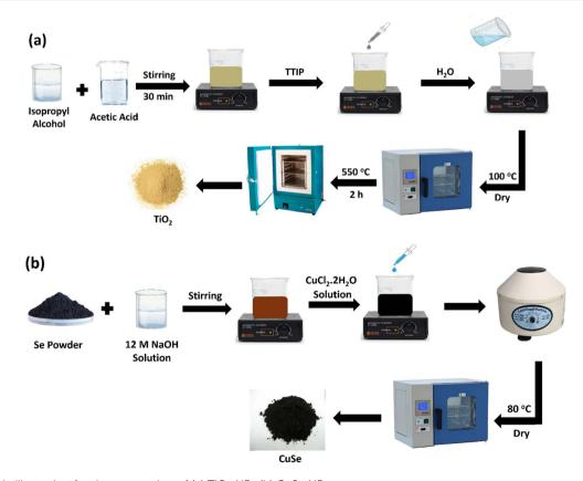
Fig. 1 Schematic illustration for the preparation of (a) TiO<sub>2</sub> NPs (b) CuSe NPs.
