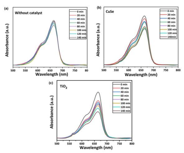
Fig. 6 Absorption spectra of MB solution obtained as a function of exposure time for (a) without any photocatalyst (b) using CuSe as a photocatalyst (c) TiO<sub>2</sub> as a photocatalyst.
