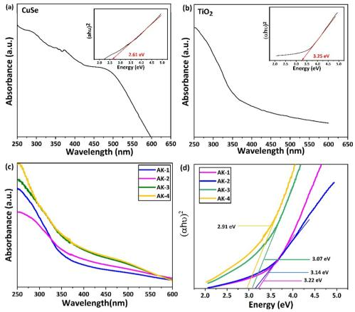
Fig. 5 (a) Absorption spectrum of CuSe. The inset shows the Tauc plot for determination of the bandgap of CuSe (b) absorption spectrum of  $TiO_2$ . The Tauc plot is presented in the inset (c) Absorption spectra of  $TiO_2$ –CuSe composites (d) Tauc plots of  $TiO_2$ –CuSe composites.
