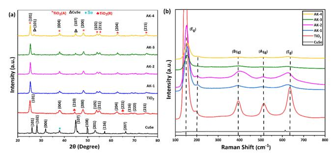
Fig. 2 (a) XRD patterns (b) Raman spectra of TiO<sub>2</sub>, CuSe, and their composites.
