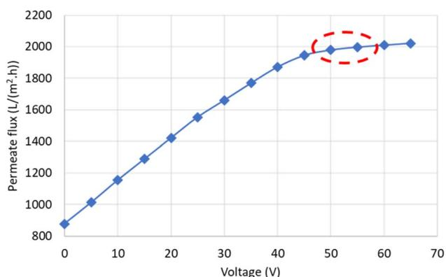
Fig. 9 Variation of permeate flux with changing voltage for oily water emulsion.  $E_{\text{crit}}$  is indicated by a red ellipse on the graph.
