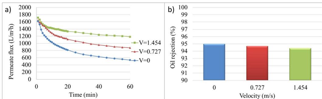
Fig. 6 Membrane performance at 2 bar and cross-flow velocities of 0, 0.727, and 1.454 m s<sup>-1</sup>: (a) permeate flux, (b) final oil rejection percentages (%).
