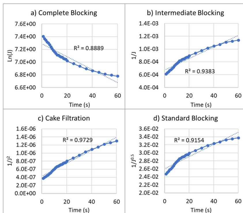
Fig. 7 Reduction of permeate flux over time for oily water emulsion at different fouling models: (a) complete blocking, (b) intermediate blocking, (c) cake filtration, and (d) standard blocking.
